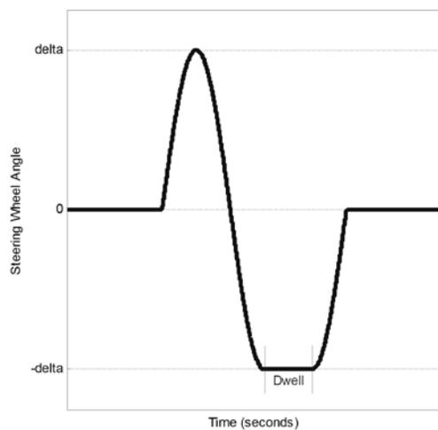
Figure 1. Steering wheel input for Sine with Dwell Maneuver.
