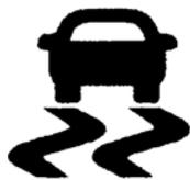
Figure 5: ESC Malfunction Telltale Symbol in FMVSS No. 101
