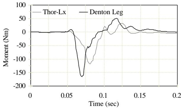
**Figure 8. Right lower tibia Mx moments measured in the Denton leg and the Thor-Lx/HIIIr in the crash test of the Nissan Altima.**
