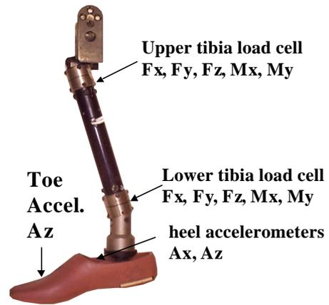
Figure 3. Instrumentation in the Denton leg.
