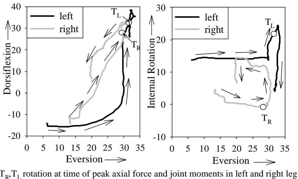
Figure 11. Foot rotations of the left and right foot of the Thor-Lx/HIIIr in the crash test of the Dodge Neon.
