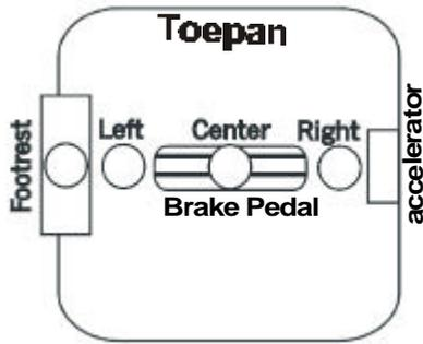
**Figure 4. Location of intrusion measurement on the toe pan.**
