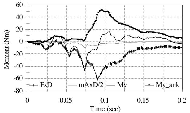
**Figure 10. Left lower tibia My moment (My), moment at ankle due to shear force (FxD), moment at ankle due inertial force (mAx D/2), and computed ankle My moment (My\_ank) from Equation 2 of the Thor-Lx/HIIIr in crash of the Toyota Camry.**
