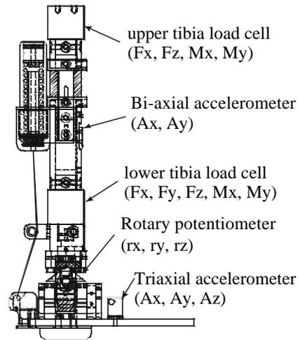
Figure 2. Instrumentation in the Thor-Lx/HIIIr.
