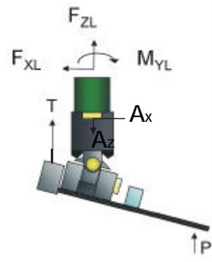
**Figure 9. Free body diagram of the foot and lower tibia load cell of the Thor-Lx/HIIIr to axial loading at the ball of foot.**
