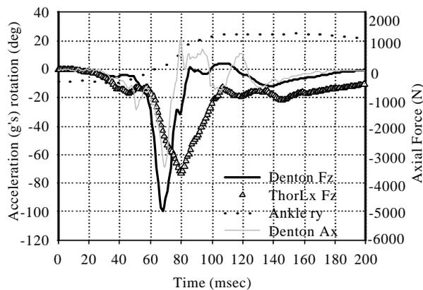
**Figure 6.** Right lower tibia axial force (Fz) in the Denton leg and Thor-Lx/HIIIr, dorsiflexion (ankle ry) in the Thor-Lx/HIIIr and foot acceleration (Ax) in Denton leg in paired tests of the Nissan Altima.
