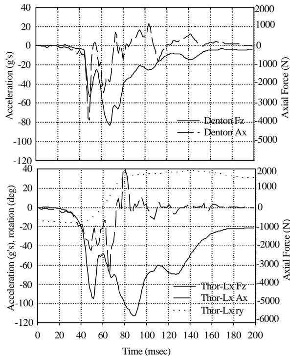
**Figure 5.** Left lower tibia axial force (Fz), longitudinal foot acceleration (Ax) of the Denton leg and Thor-Lx/HIIIr, and dorsiflexion angle (ry) of the Thor-Lx/HIIIr in the crash tests of the Dodge Neon.
