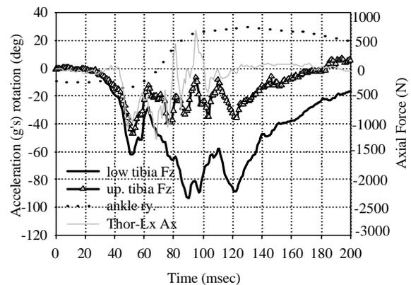
**Figure 7.** Axial force (Fz) measured in the upper and lower tibia load cell, foot acceleration, and dorsiflexion in the right Thor-Lx/HIIIr leg in the crash test of the Toyota Camry .
