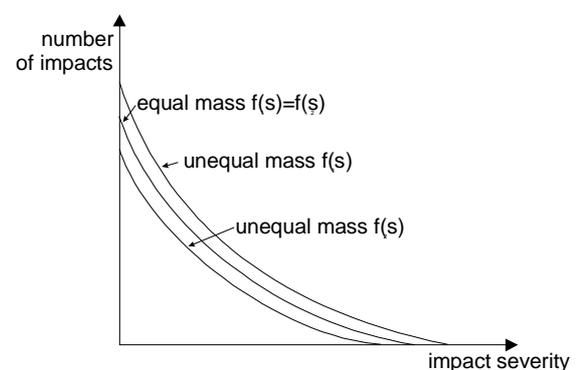
**Figure 1. Impact severity (delta-V) for cars in matching crashes for equal mass:  $f_1(s) = f_2(s)$  and unequal mass:  $f_1(s) \neq f_2(s)$  where car 1 is of less mass than car 2.**
