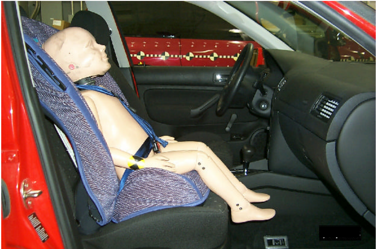
S22.2.1 - 3 year old in forward-facing CRS, seat recline = 30°, seat full rearward, 1999 VW Jetta
