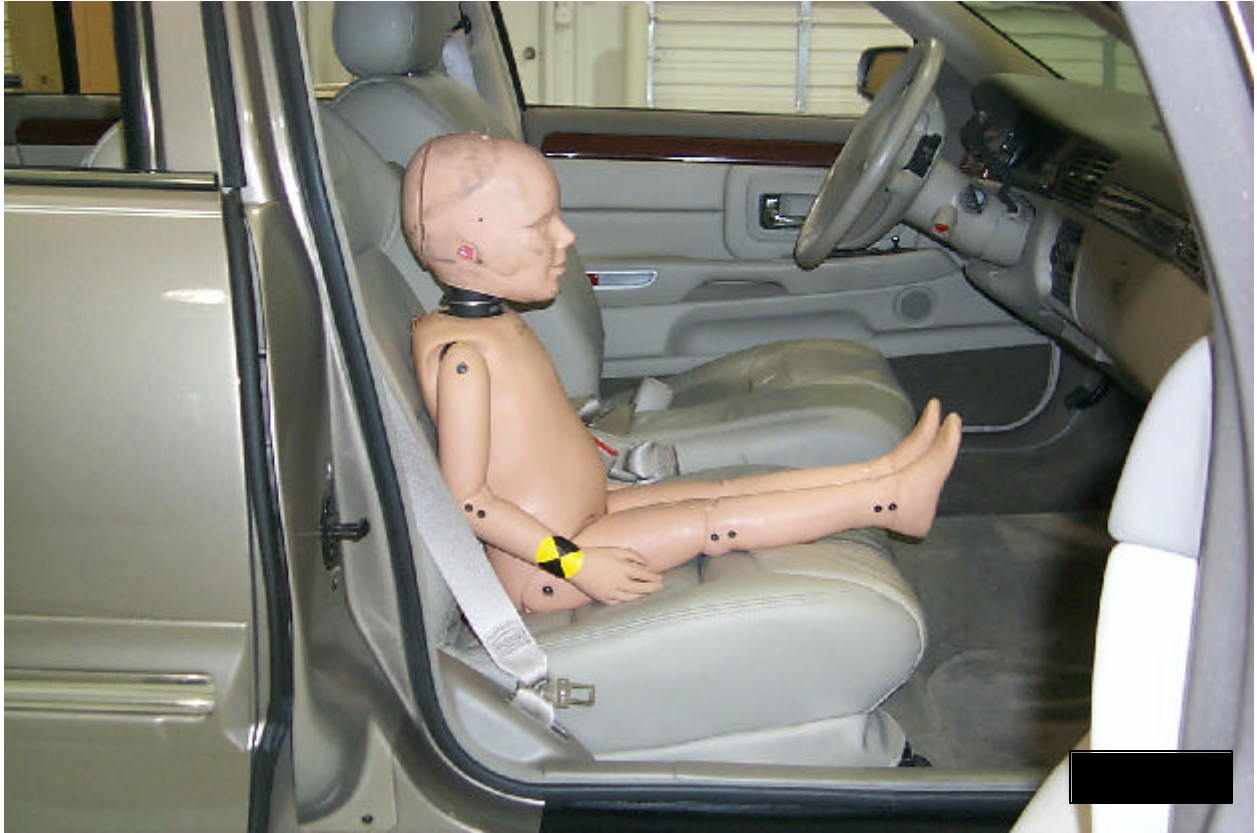
S22.2.2.2(a) - 3 year old, seat recline = 30°, seat full rearward, 1999 Cadillac DeVille (60-40 split bench)
