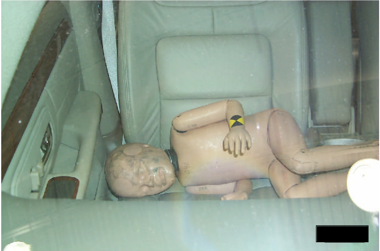
S22.2.2.2(g) - 3 year old (head relative to side door = 2 mm), seat recline = 30E, seat at mid track position, 1999 Cadillac DeVille (60-40 split bench)
