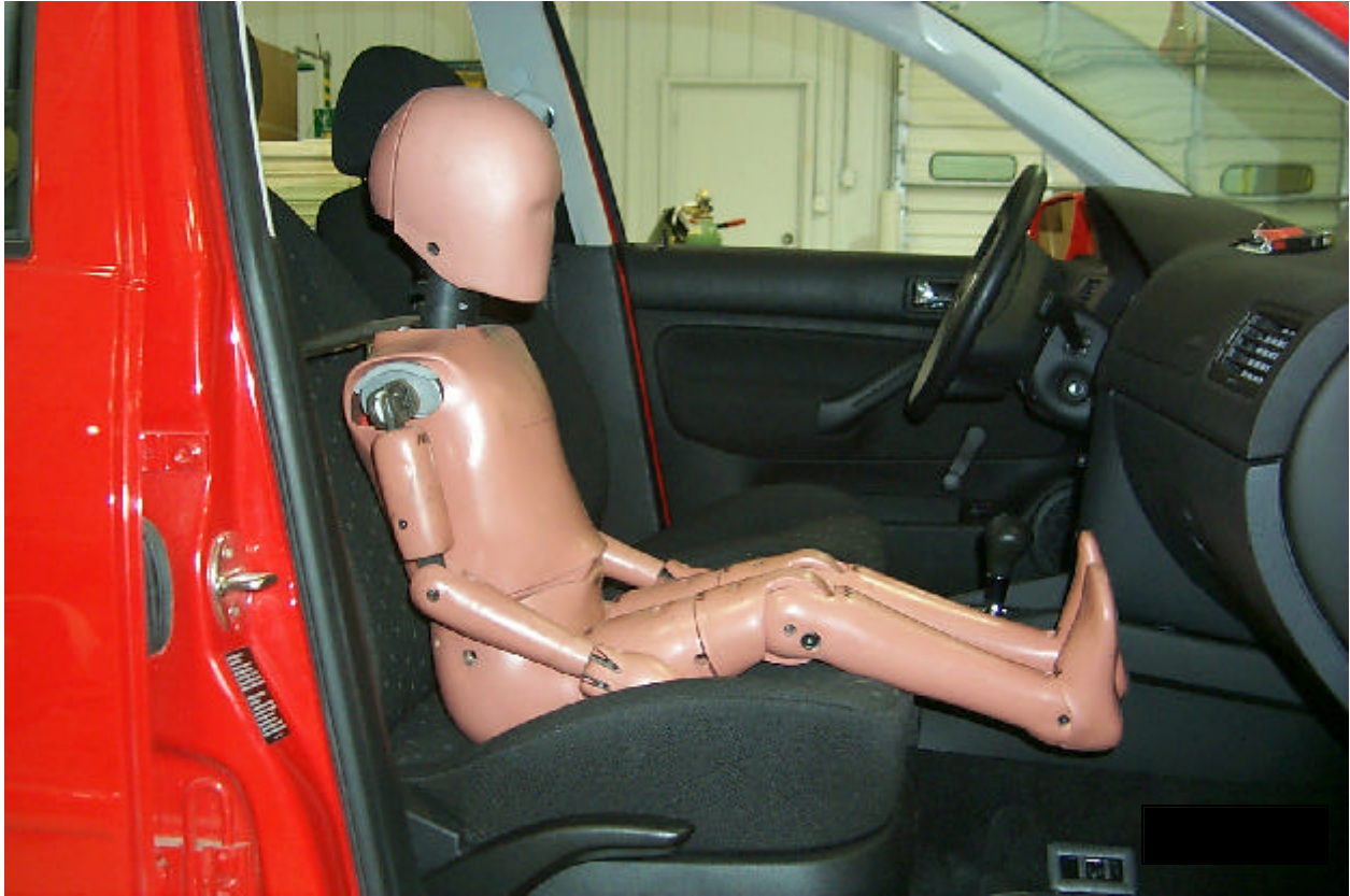
S24.2.1 [S22.2.2.2(b)] - 6 year old seated 3" from seat back, seat recline = 30°, seat full rearward, 1999 VW Jetta
