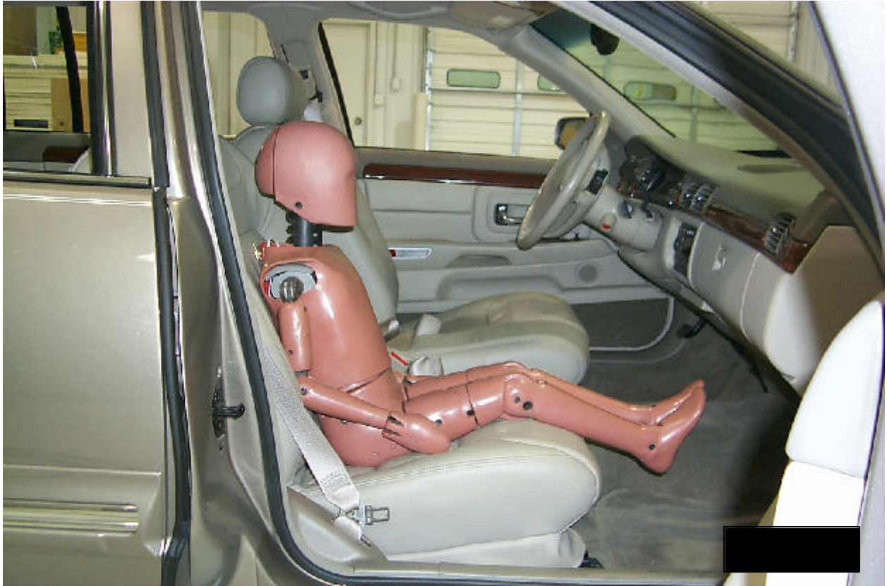
S24.2.1 [S22.2.2.2(a)] - 6 year old, seat recline = 30°, seat full rearward, 1999 Cadillac DeVille (60-40 split bench)
