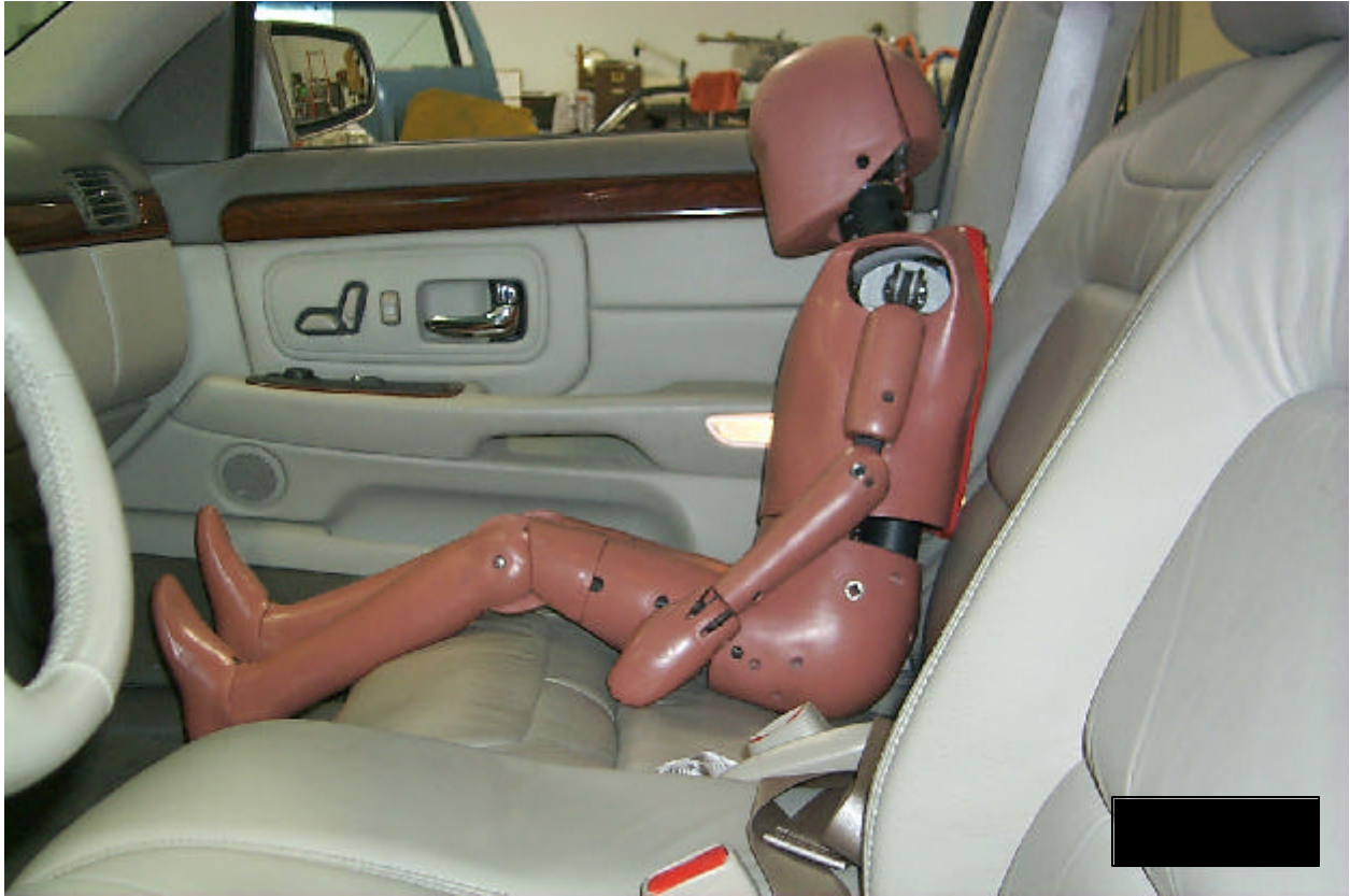
S24.2.3 - 6 year old, seat recline = 30°, seat full rearward, 1999 Cadillac DeVille (60-40 split bench)
