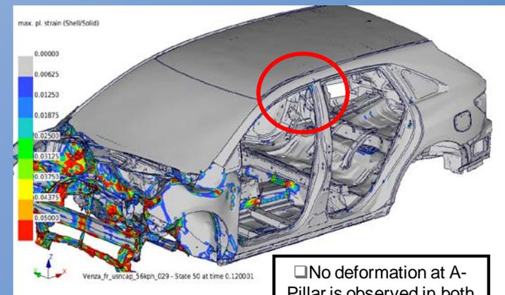
No deformation at A-Pillar is observed in both model.
