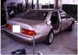
This case involved a 12 year old female who was the left rearseat occupant in a 1997 Lexus LS 400. The occupant was wearing the available 3-point lap and shoulder restraint. The case vehicle was struck on its right side by a 1997 Toyota Tercel. The point of impact was at the rear right door opposite from the case occupant (see Figure 2.6). The lateral delta V was estimated to be 15 mph and the PDOF was 2 o'clock.
