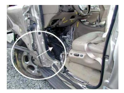
The impact with the tire/axle of the lower passenger vehicle forced the front left tire of the sport utility vehicle (shown here) into the floor and toe pan of the driver position. This resulted in severe bilateral foot fractures. The intruding front left tire of the sport utility vehicle is outlined in white.
