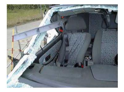
The side impact protection in the passenger vehicle door was overcome by the higher bumper frame of the sport utility vehicle. This is demonstrated by the intrusion of the upper portion of the door. Such intrusion results in a significant risk of severe chest injury.
