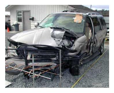
Offset frontal impact in which the pictured sport utility vehicle (SUV) with a higher bumper frame collided with a passenger vehicle with a lower bumper frame. This resulted in an impact to the tire/axles below the SUV bumper frame.
