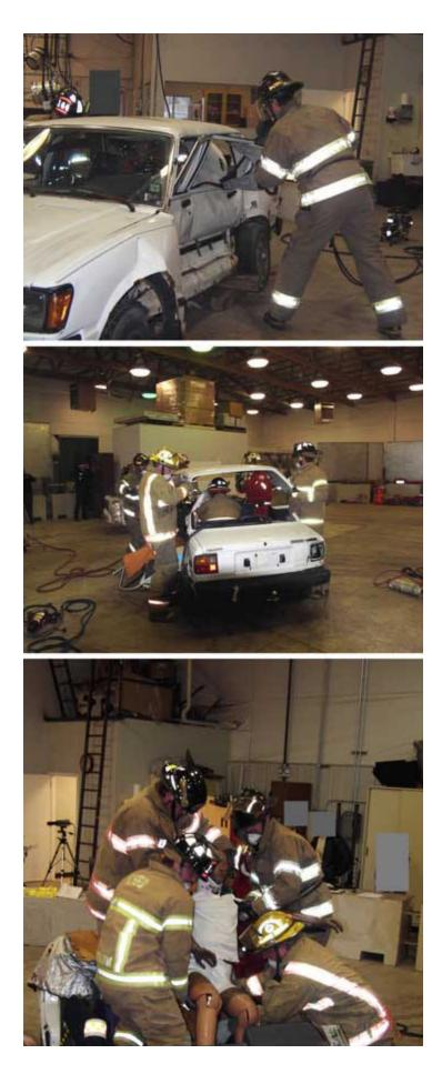
The dummy neck loads are monitored to give firefighter rescuers feedback on techniques.
