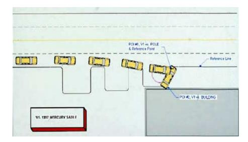
The Delta V was 73kph (41mph) and the maximum crush was 81cm at C2 (Figure 2). The passenger airbag deployed on impact, but because the passenger was unrestrained and the primary impact was on the driver's side at 3500 PDOF, the patient missed the airbag and impacted his anterior left chest wall and sternum on the left side of the central instrument panel (Figure 3).
