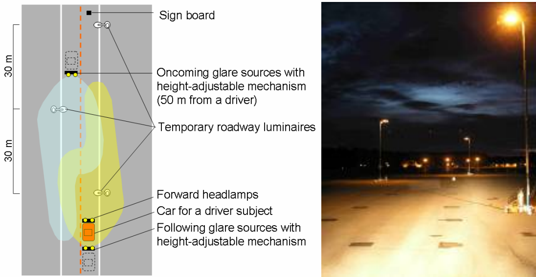
Figure 1. Layout of experimental setup including three fixed roadway lighting poles.
