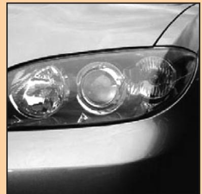
*Directionally Adaptive Headlamps adjust the aim of the headlight beams to illuminate the roadway based on inputs from the vehicle (steering wheel, speed, yaw).*
