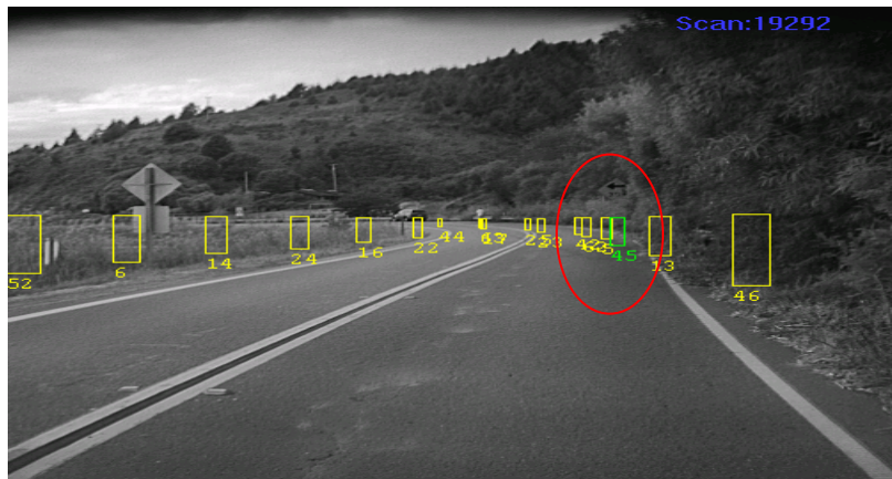
Figure 41: False Activation on Stationary Object during Curve-Exit
