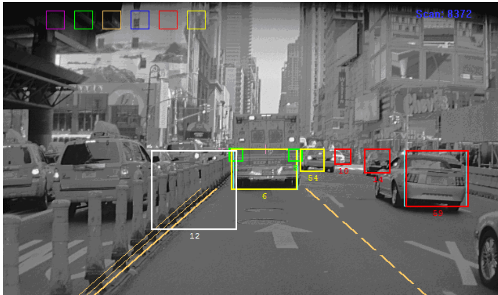
Figure 52: False Precharge Event at Baseline Sensitivity Due to Roadside Object
