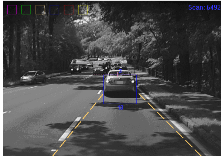
Figure 47: Shadow-on-Road Influencing Vision Measurement
