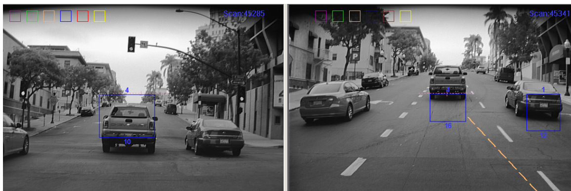
Figure 48: Change-in-Vehicle Pitch Influencing Vision Measurement
