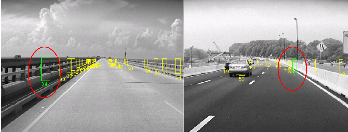
Figure 42: False Events Caused by Roadside Objects
