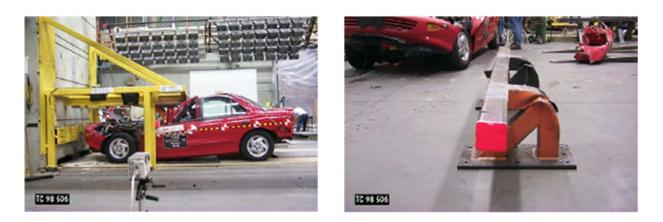
Figure F-2 Crash test, Chevrolet Cavalier into 480 mm guard at 65 km/h. Note the highly deformed guard
