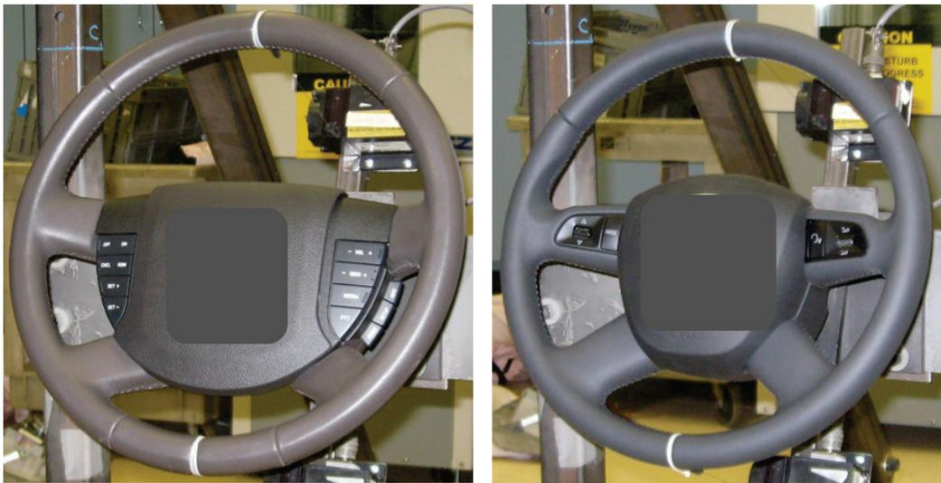
**Figure 23 - PVP Steering Wheel (Left) and ARS Surrogate Steering Wheel (Right)**
