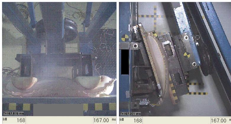
**Figure 28 - ARS KAB Shown in a Pendulum Test Fixture**
