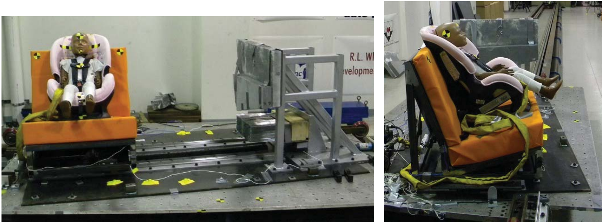
Figure 1: Front and side view of the side impact fixture attached to the deceleration sled
