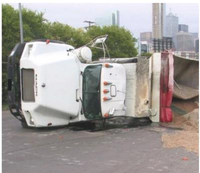
Figure 19 SUT rollover, cab protected by the cargo body
