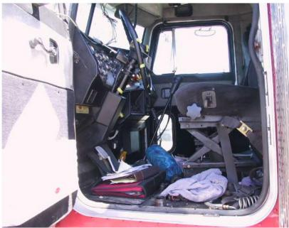
Figure 41 Steering Wheel Deformed by Belted Driver in Frontal Impact
