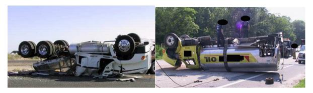
Figure 42: Comparative Images of Truck Body Influence on Cab Crush
