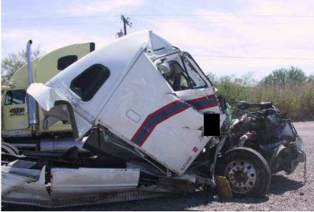
Figure 32 Truck Cab After Rear Trailer Intrusion
