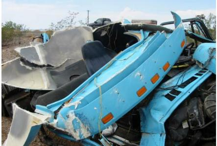
Figure 16 Truck-tractor rolled 4 quarter turns, destroying the cab
