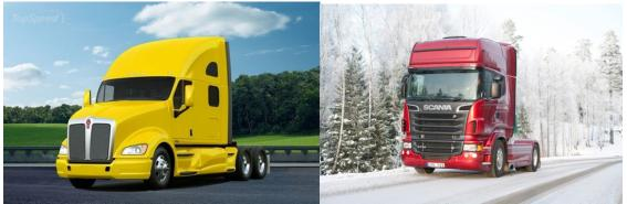
Figure 1 Conventional (left) and Cab Over Engine Cab Styles
