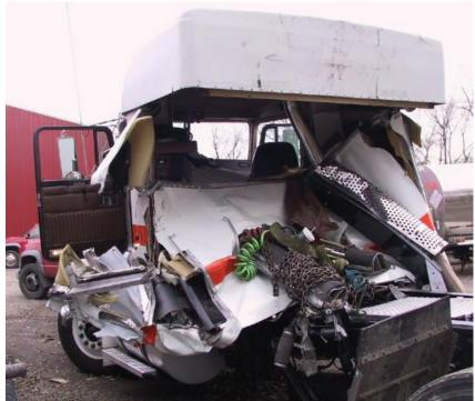
Figure 30 Truck Cab Rear Intrusion from Steel Coil
