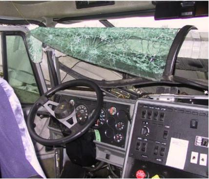
Figure 29 Hood Intrusion in Frontal Collision
