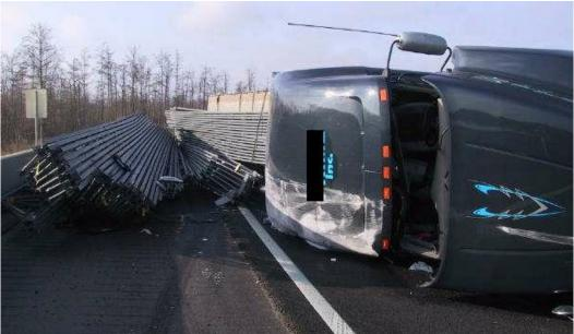
Figure 23 Rollover with subsequent contact with concrete barrier
