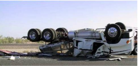
Figure 15 Truck-tractor with 100 percent Crush
