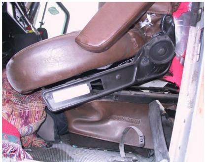
Figure 31 Broken Seat Mount from Rear Intrusion
