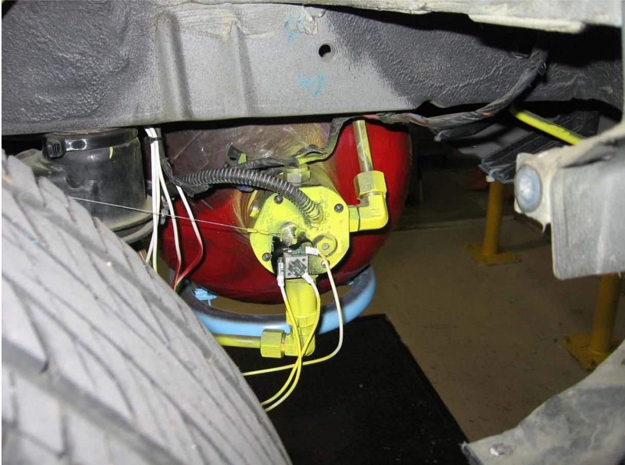
Figure 2-2. A triaxial accelerometer is visible on the valve, which is on the driver side of the rear container. Similar triaxial accelerometers were mounted on both ends of all three containers on both vehicles. The string for the string potentiometer is attached to the hex stem on the solenoid end valve. String potentiometers measured longitudinal displacement in the rear crash (shown here) and lateral displacement in the side crash.
