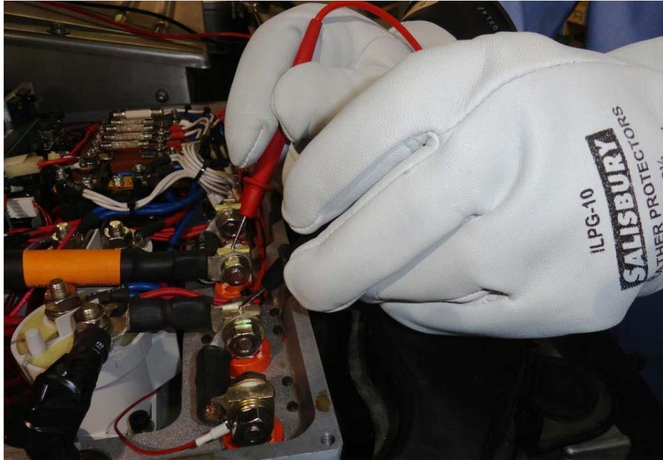
Figure 2-5. Test points were measured with a conventional multimeter to ensure that no voltage was present before the safety analyzer applied the high-voltage for the isolation tests.
