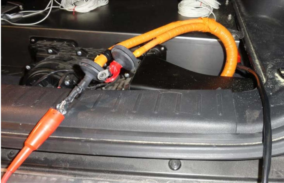
Figure 2-9. Close-up of the connections for testing the isolation of the line that runs to the high-voltage battery.
