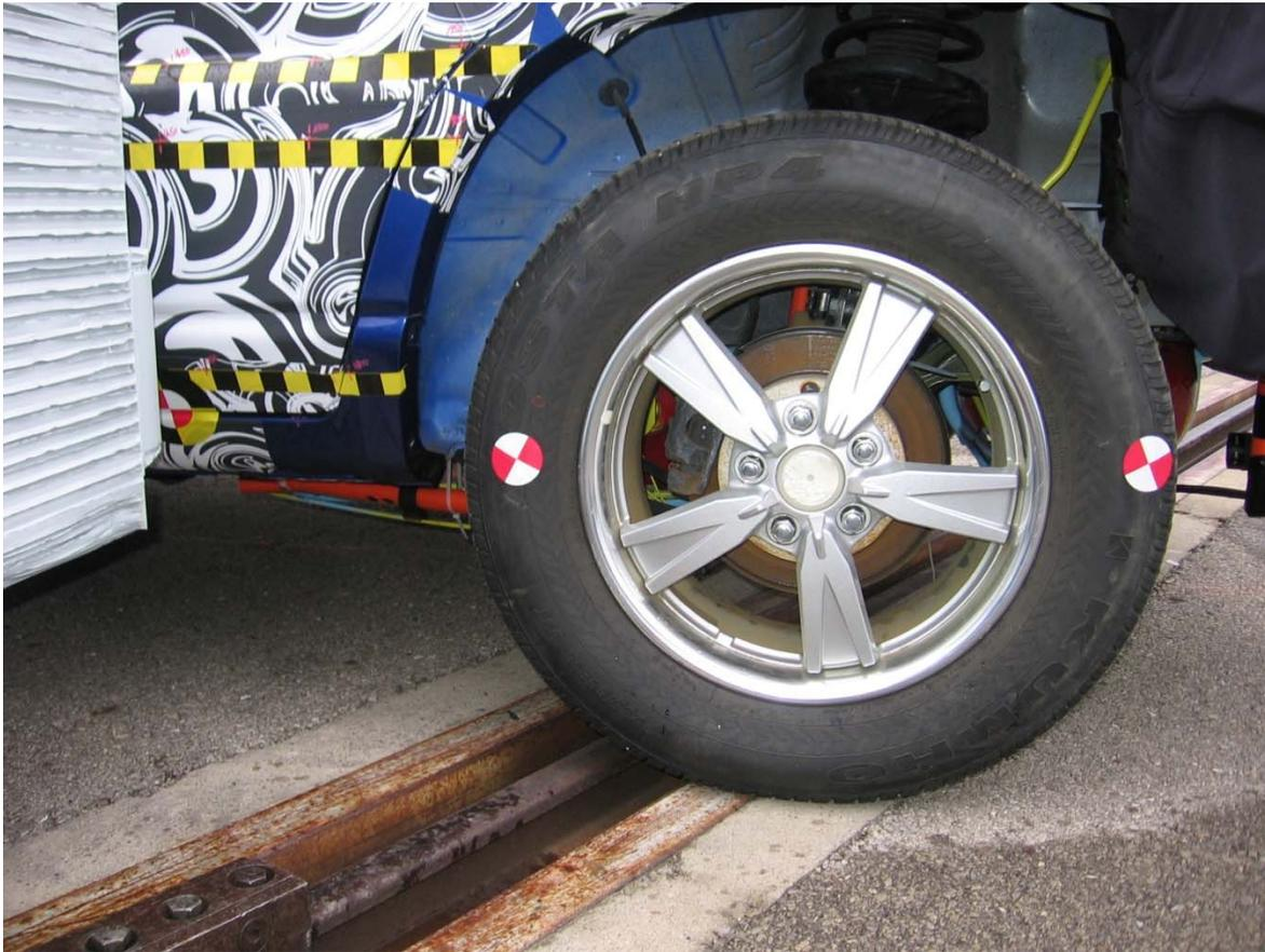
Figure 2-1. The red-and-white targets are aligned with the three fuel containers. One target is on the sill below the rear door, and two are on the rear tire. The forward container was within the span struck by the moving deformable barrier.
