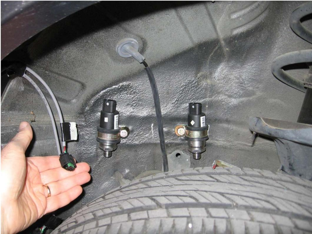
Figure 2-3. The two externally mounted helium sensors were in the driver side rear wheel well, above the two smaller fuel containers, as shown here for the rear crash. The electrical connector for a sensor is in the hand. A sensor was mounted under the vehicle near the valve of the forward container for the side crash.
