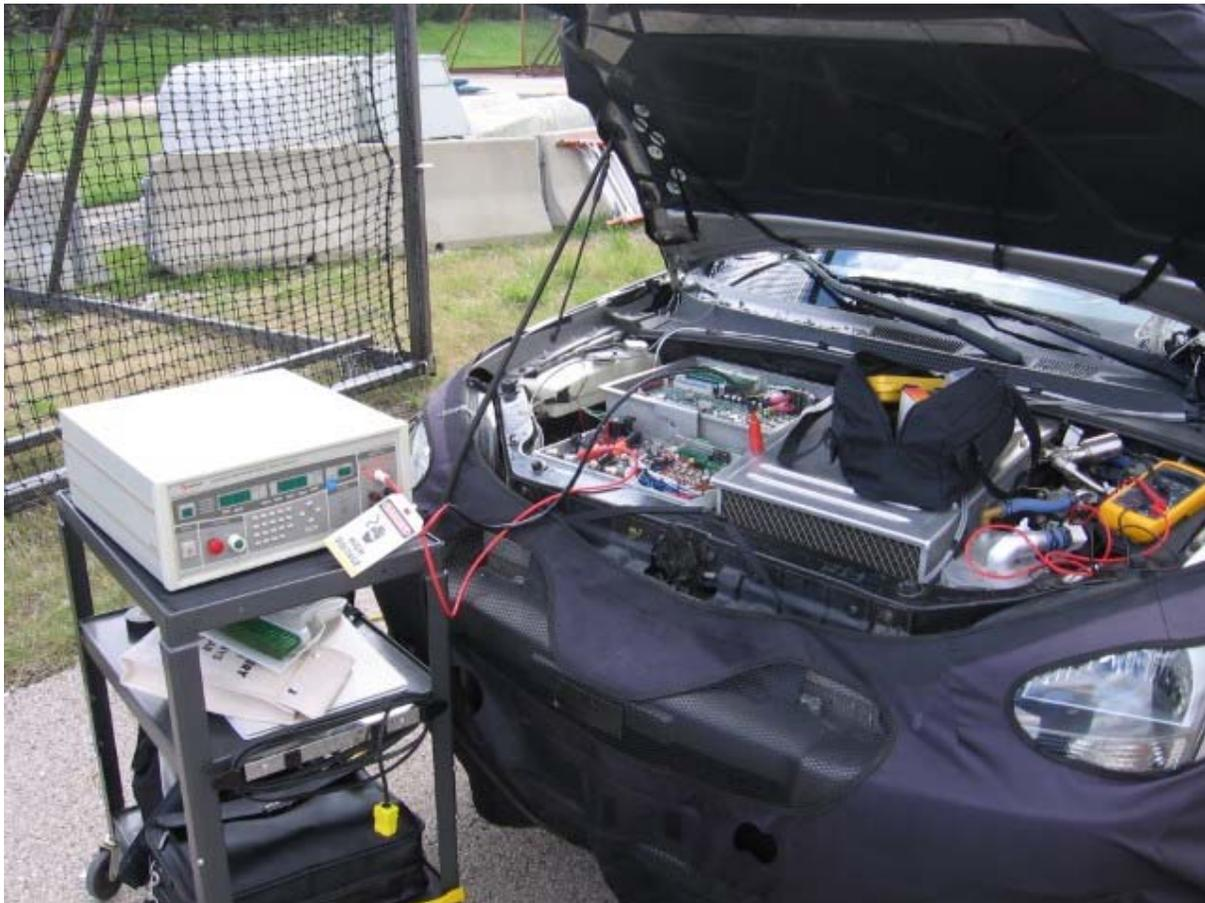
Figure 2-6. The safety analyzer is attached to the fuel cell lines following the rear crash.
