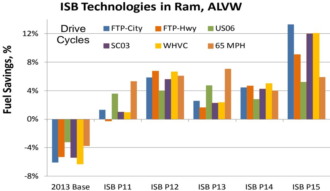
**FIGURE 2.19 DIESEL TECHNOLOGY COMBINATIONS IN THE RAM PICKUP**
