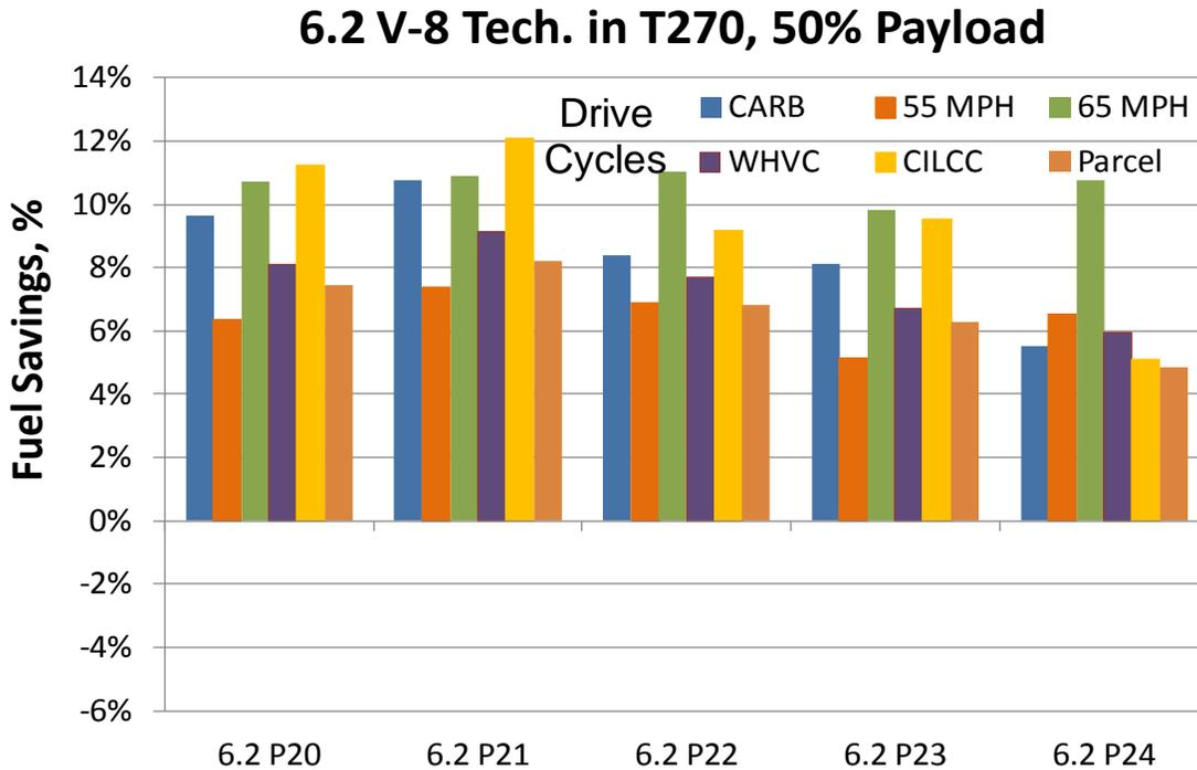
**FIGURE 2.14 FUEL SAVING PERFORMANCE OF 6.2 V8 TECHNOLOGY PACKAGES IN THE T270 TRUCK**
