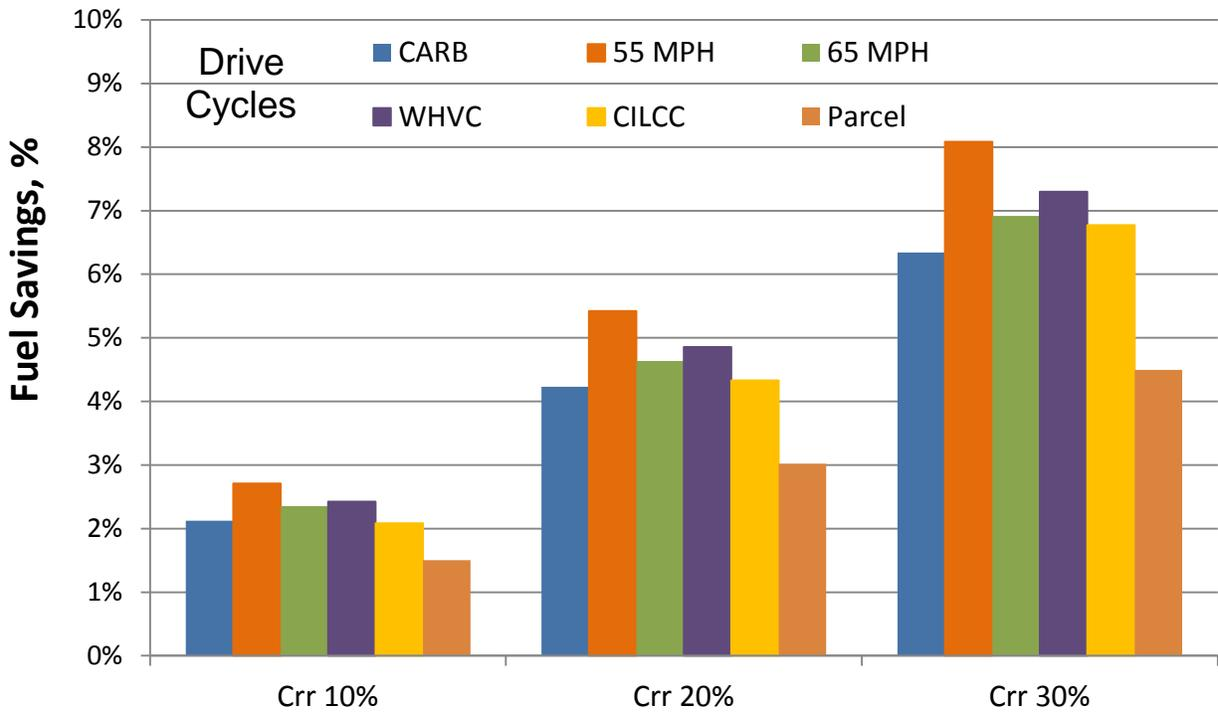
FIGURE 3.5 CRR SWEEP OF THE T270 DELIVERY TRUCK
