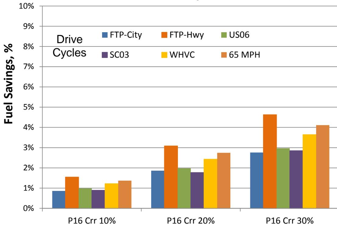
**FIGURE 3.6 CRR SWEEP OF THE RAM PICKUP**
