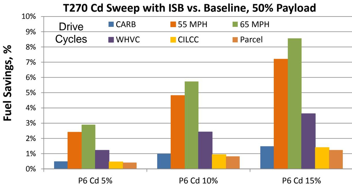
**FIGURE 3.2 CD SWEEP OF T270 DELIVERY TRUCK**
