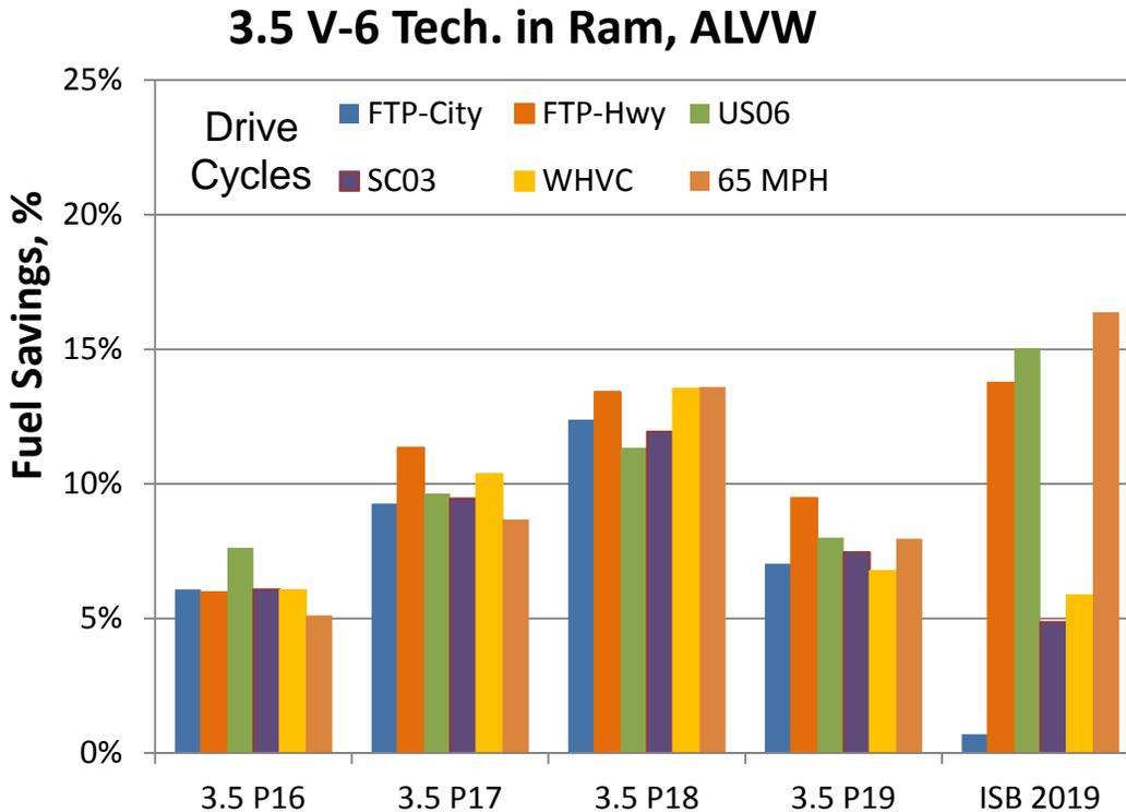
**FIGURE 2.20 3.5 V6 TECHNOLOGY COMBINATIONS IN THE RAM PICKUP**
