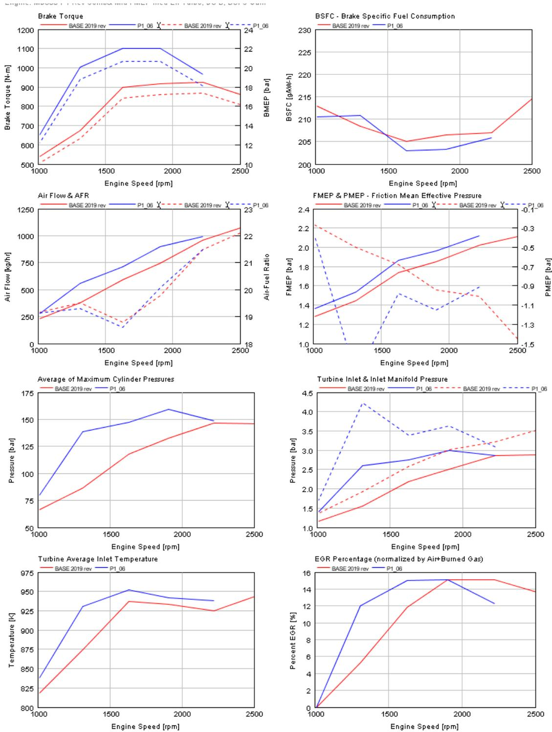
**FIGURE B2.2C PACKAGE 6 FULL LOAD PERFORMANCE COMPARISON**
