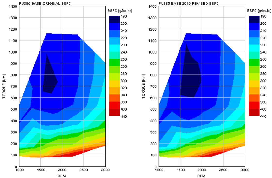
**FIGURE B3.1A BSFC MAPS OF 2013 BASE ENGINE AND 2019 BASE ENGINE**
