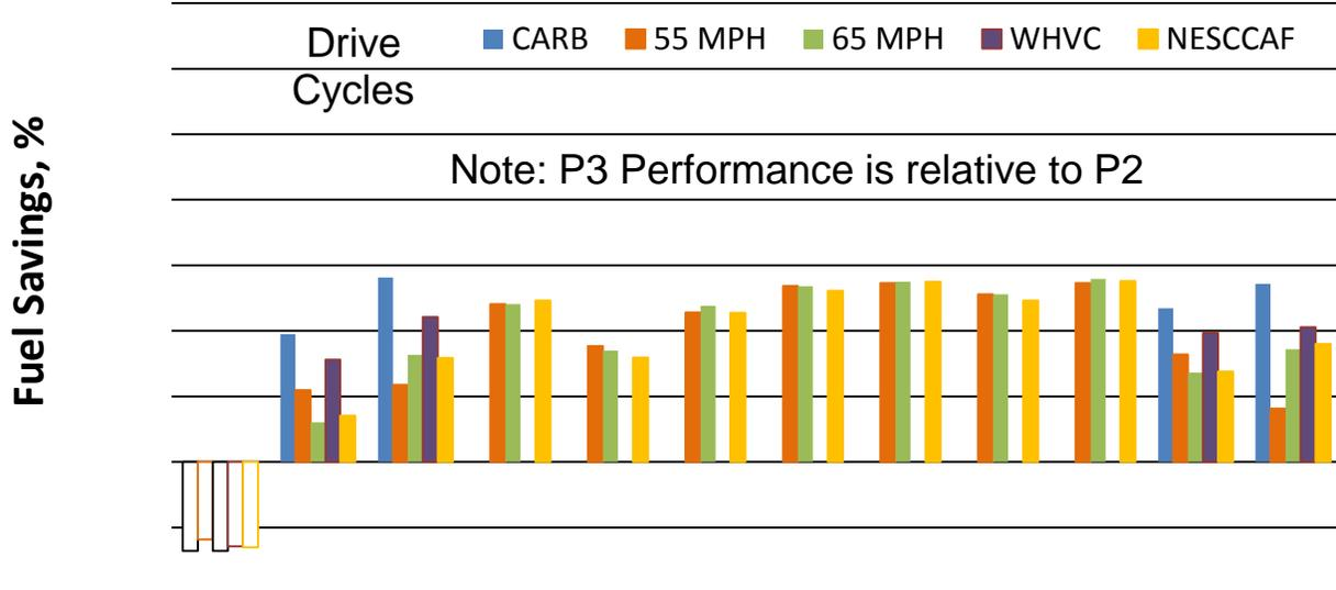
**FIGURE 2.1 FUEL SAVING PERFORMANCE OF DD15 TECHNOLOGY PACKAGES, WITH P3 RESULTS DISPLAYED RELATIVE TO THE P2 RESULTS RATHER THAN TO THE 2019 BASELINE**
