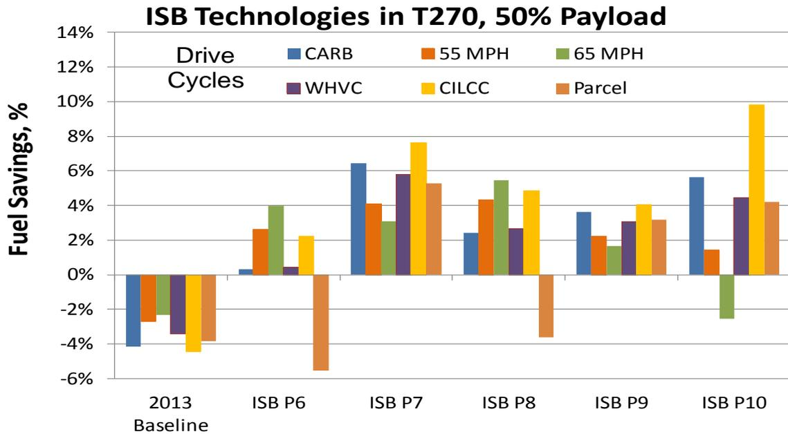
**FIGURE 2.12 FUEL SAVING PERFORMANCE OF ISB TECHNOLOGY PACKAGES IN THE T270 TRUCK**
