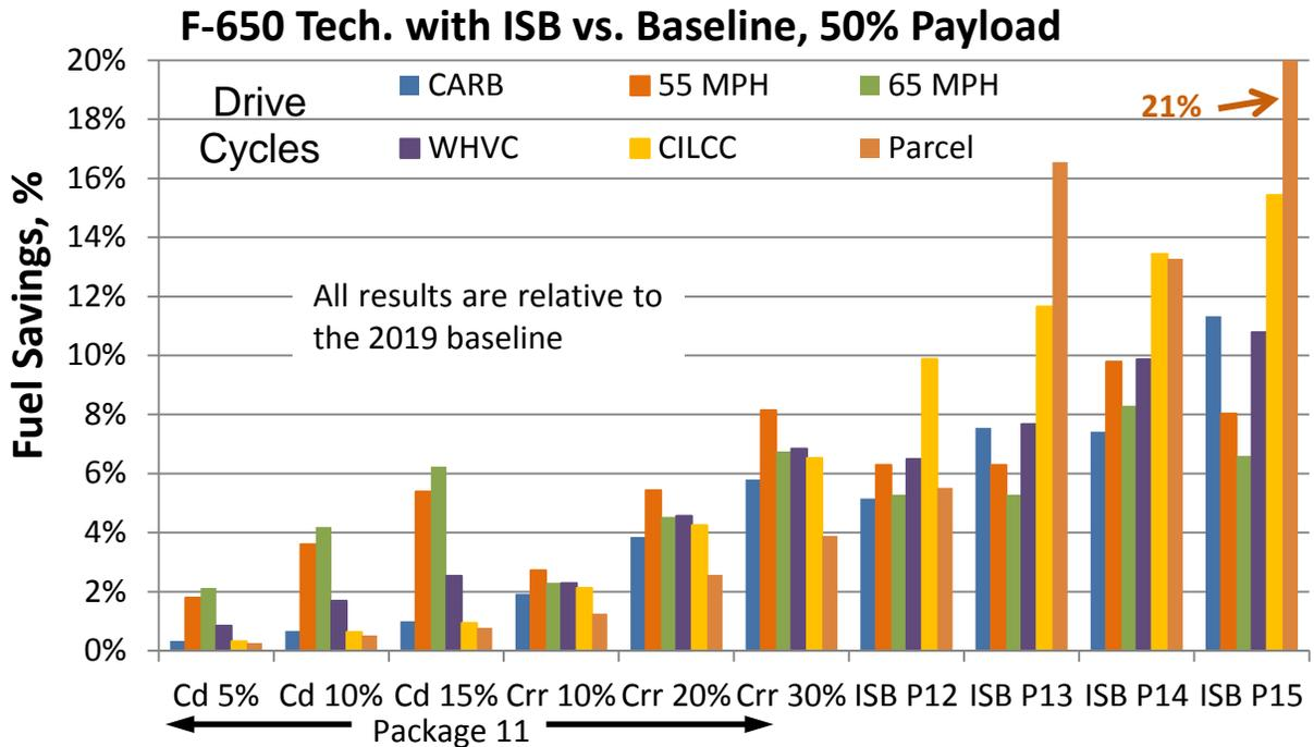
**FIGURE 2.10 F-650 VEHICLE TECHNOLOGY COMBINATION FUEL SAVINGS RESULTS WITH THE 2019 BASELINE ISB ENGINE. ALL RESULTS ARE RELATIVE TO THE 2019 ISB BASELINE**
