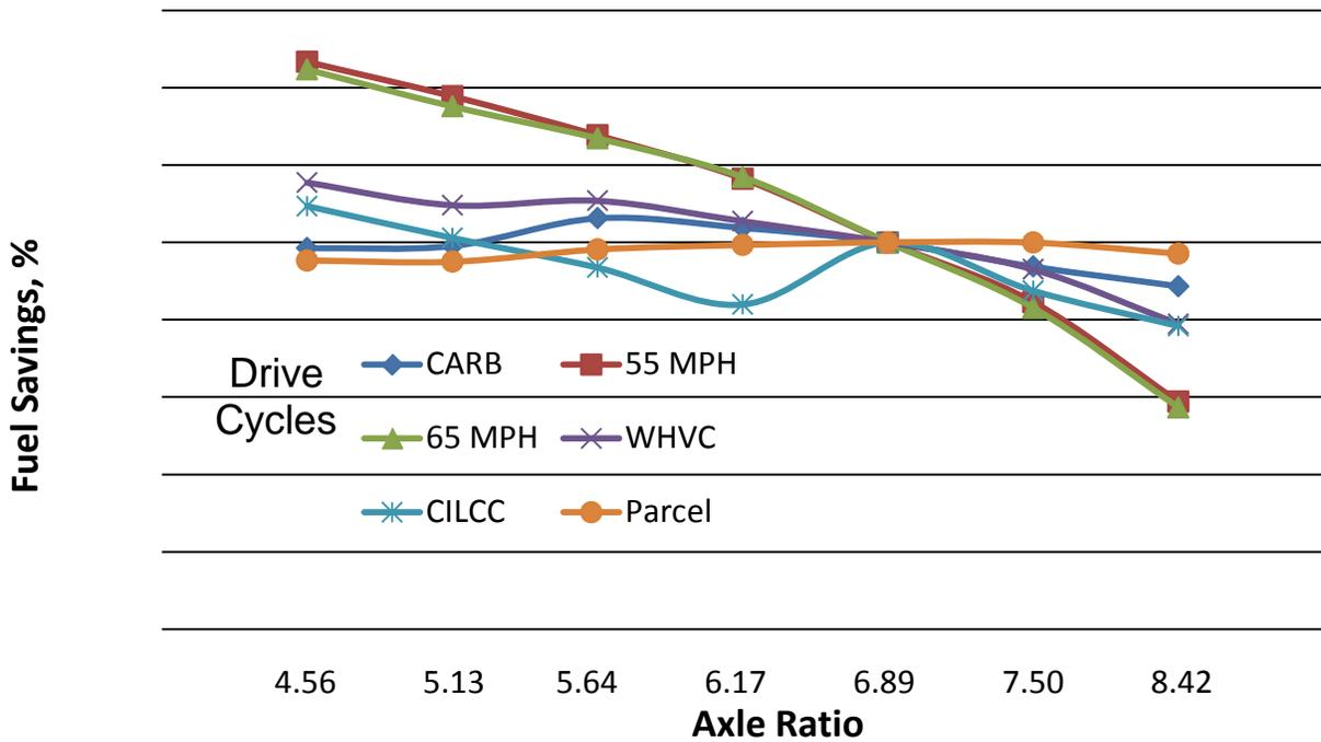
FIGURE 3.12 AXLE RATIO SWEEP ON F-650 WITH THE 6.2 V-8
