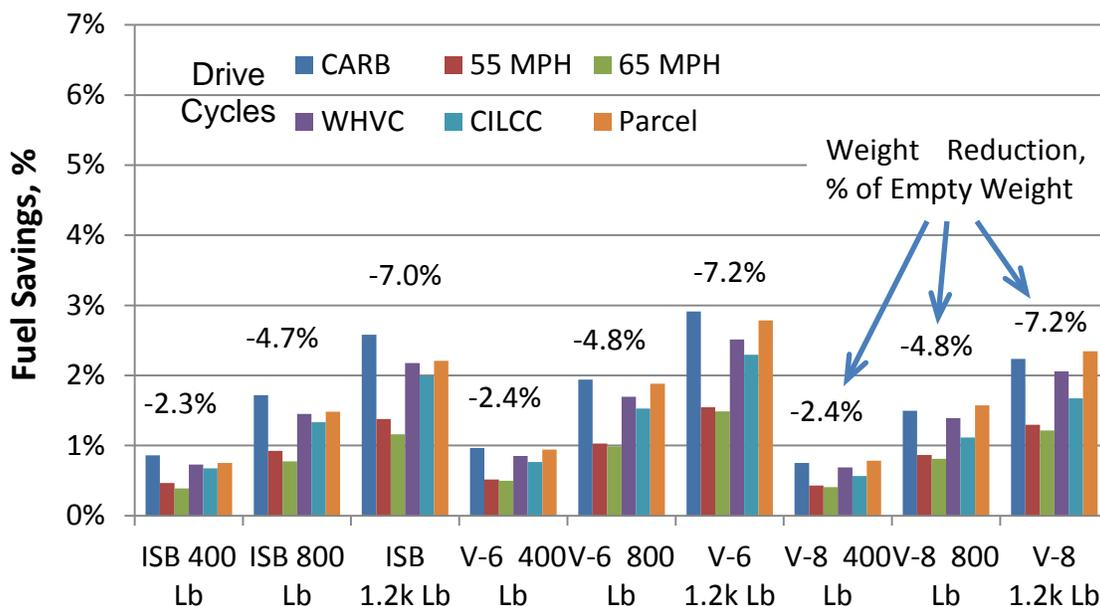
FIGURE 3.8 EFFECT OF EMPTY WEIGHT REDUCTION ON T270
