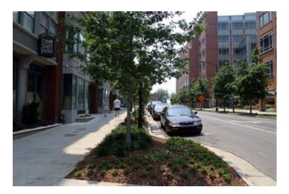
Figure 27. Sidewalk with landscaped buffer and curb extension. (Source: pedbikeimages.org / Dan Burden).
