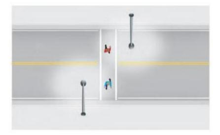
Figure 18. Proper placement of pedestrian-scale lamp posts provides illumination for the crosswalk. (Source: Michele Weisbart for the Model Design Manual for Living Streets).
