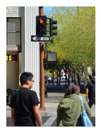
Figure 29. This Leading Pedestrian Interval in Phoenix, Arizona, gives pedestrians a five second head-start before drivers get a green light. Note that the pedestrian WALK indication is on while the motorists are still briefly held with a red light. (Source: Federal Highway Administration, Designing for Pedestrian Safety Course 201).
