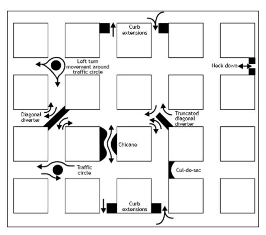
Figure 30. Visualization of various traffic calming devices. (Source: FHWA university course on bicycle and pedestrian transportation).
