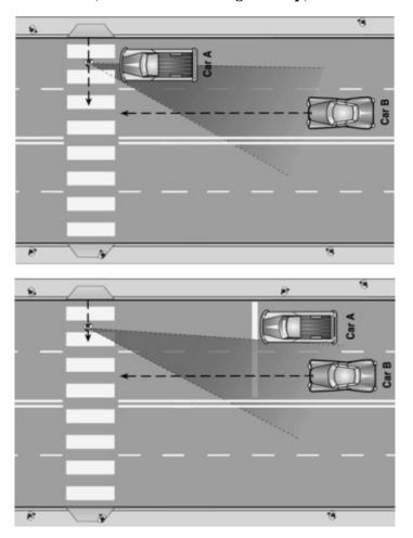
Figure 9. Before and after illustrations show how compliance with an advance stop/yield line can improve the view for pedestrians and drivers. (Source: National Center for Safe Routes to School Guide).
