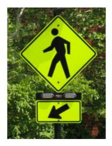
Figure 23. Rectangular Rapid Flashing Beacon. (Source: Carol Kachadoorian).
