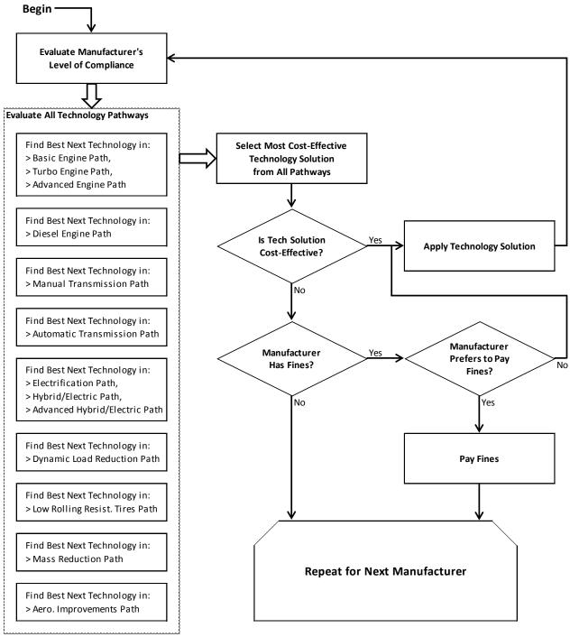
Figure 7. Compliance Simulation Algorithm
