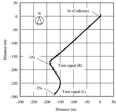
**Figure 3. Driving path of Car A.**
