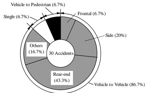
**Figure 1. Configurations of the accidents in a fleet test.**
