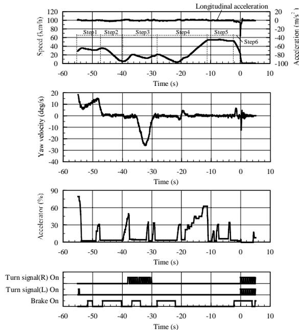
**Figure 2. Accident data collected by Recorder-A.**
