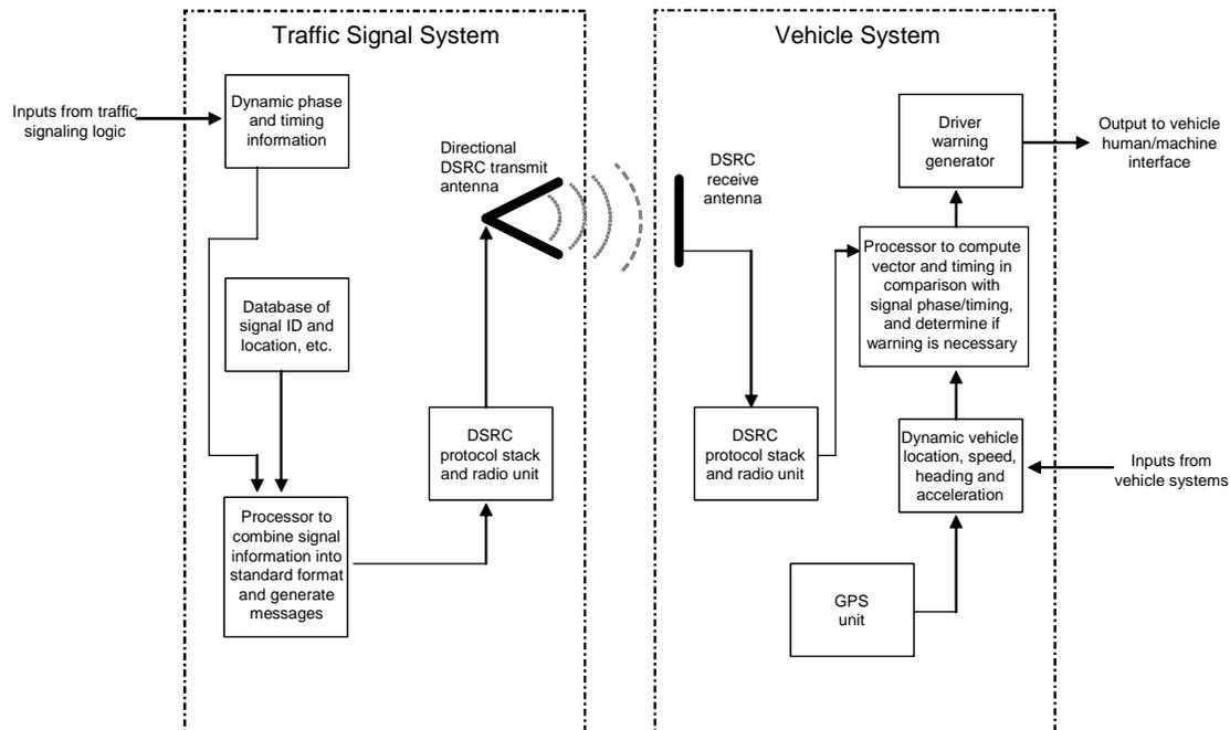
**Figure 4.5 Traffic Signal Violation Warning Block Diagram**
