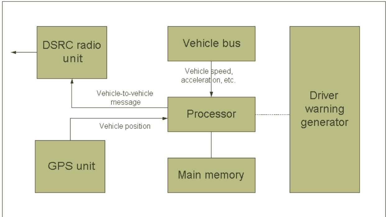
**Figure 4.37 Vehicle-to-Vehicle Message Sender Architecture and Information Flow**
