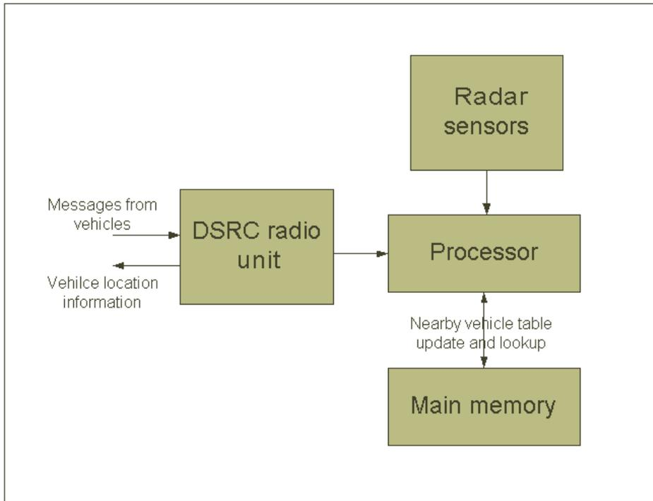
**Figure 4.38 Roadside Unit Hardware Architecture and Information Flow**
