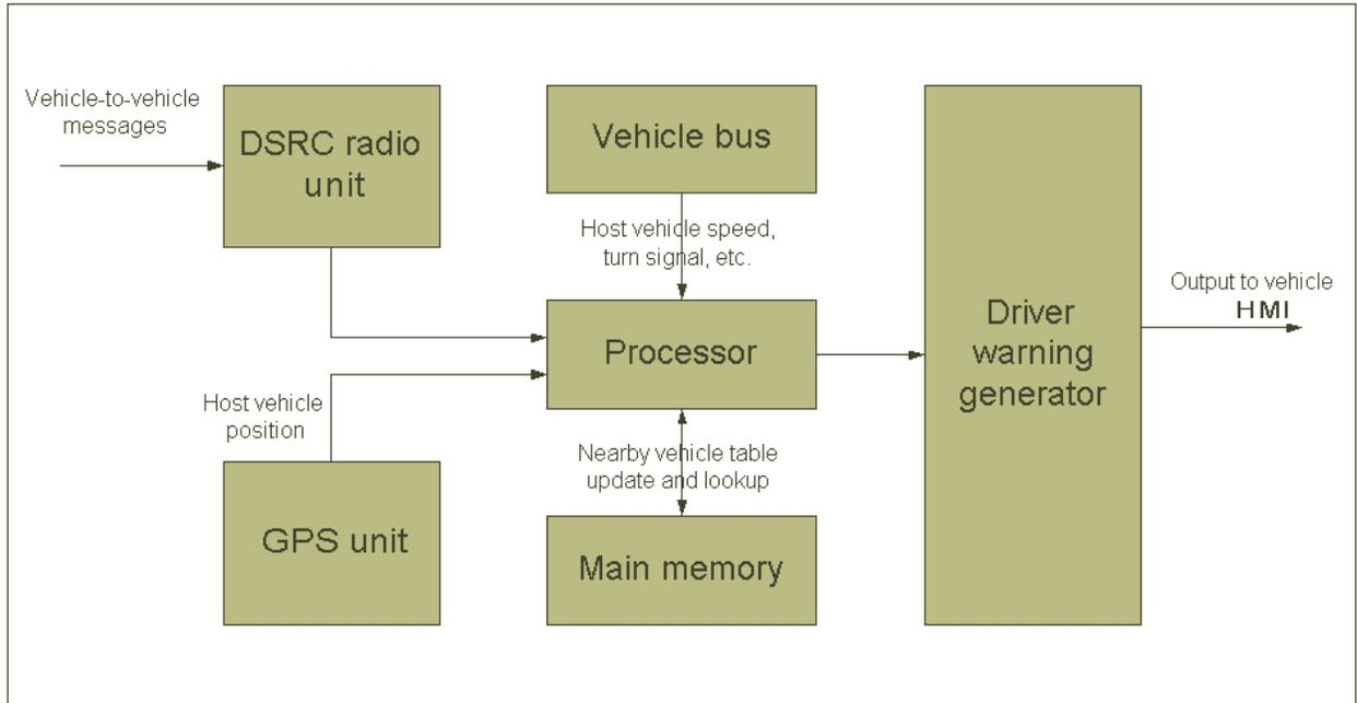
**Figure 4.36 Application Host Vehicle Architecture and Information Flow**
