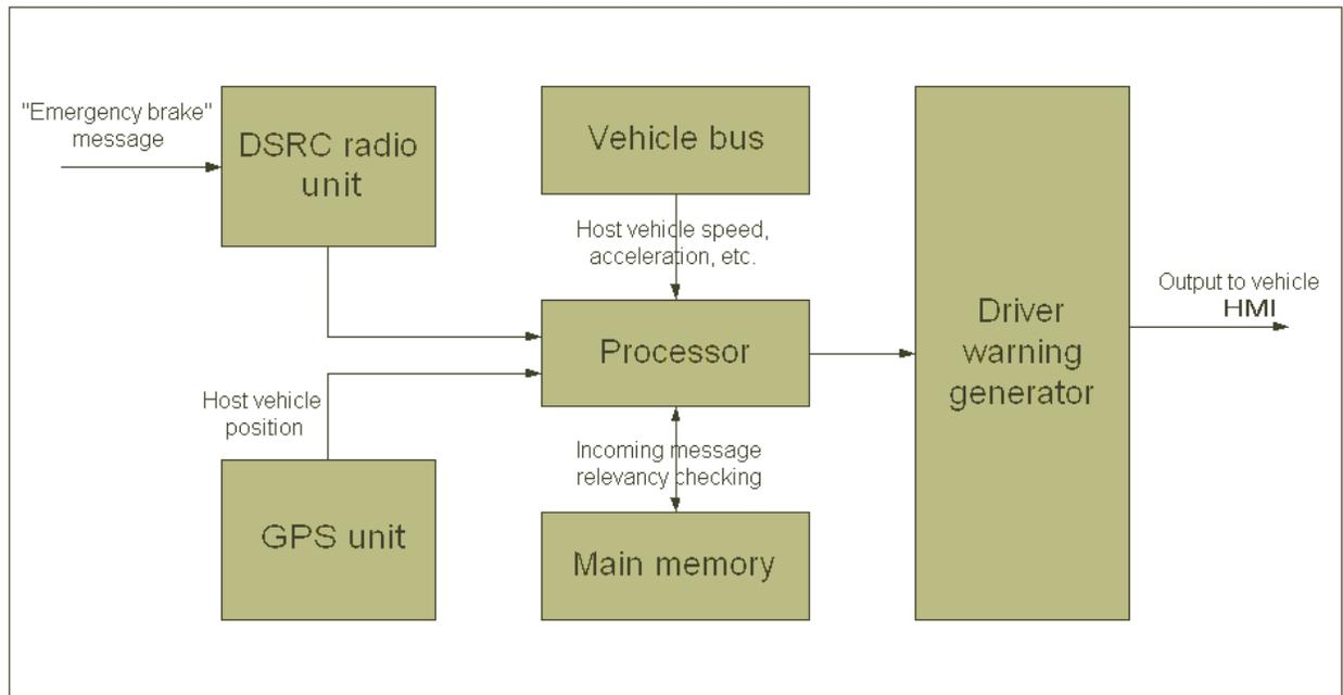
**Figure 4.10 Emergency Electronic Brake Light Block Diagram I**
