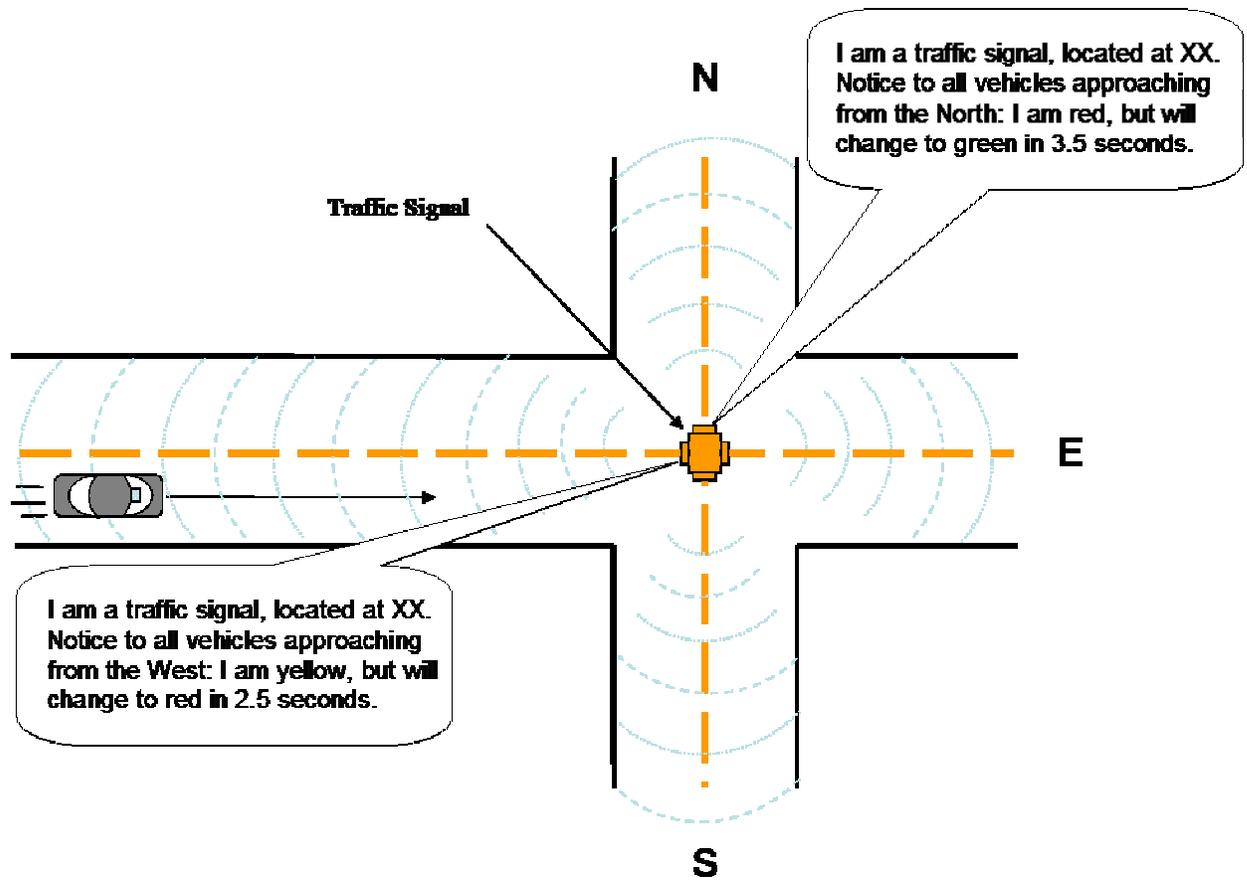
Figure 4.3 Traffic Signal Violation Warning: Directed Signal Phase Messages – Turning Red
