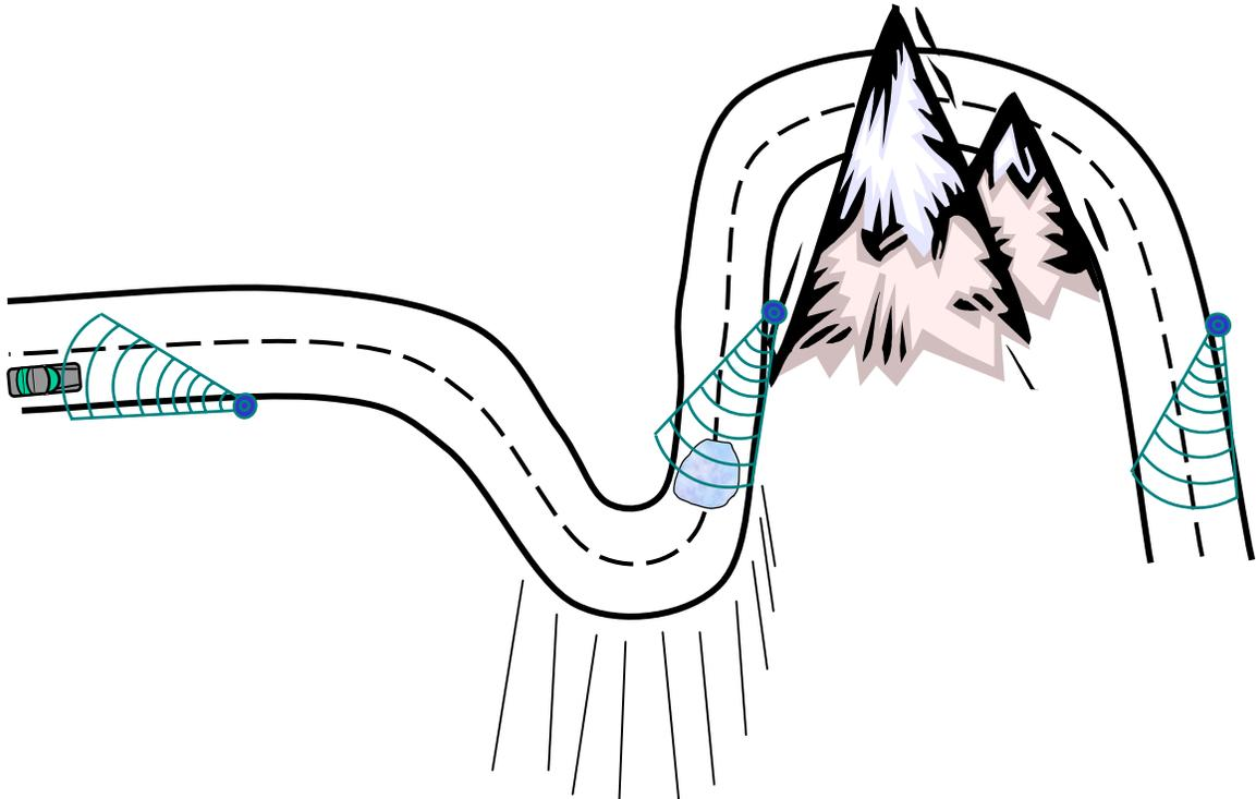
Figure 4.6 Curve Speed Warning Scenario
