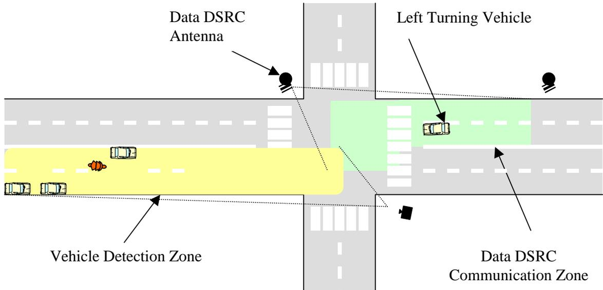
**Figure 4.20 Data DSRC Communications**
