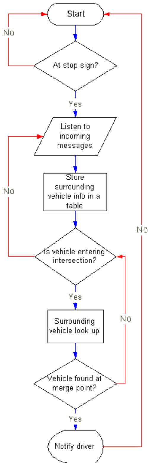
**Figure 4.39 Stop Sign Movement Assistant Application Flow Chart**
