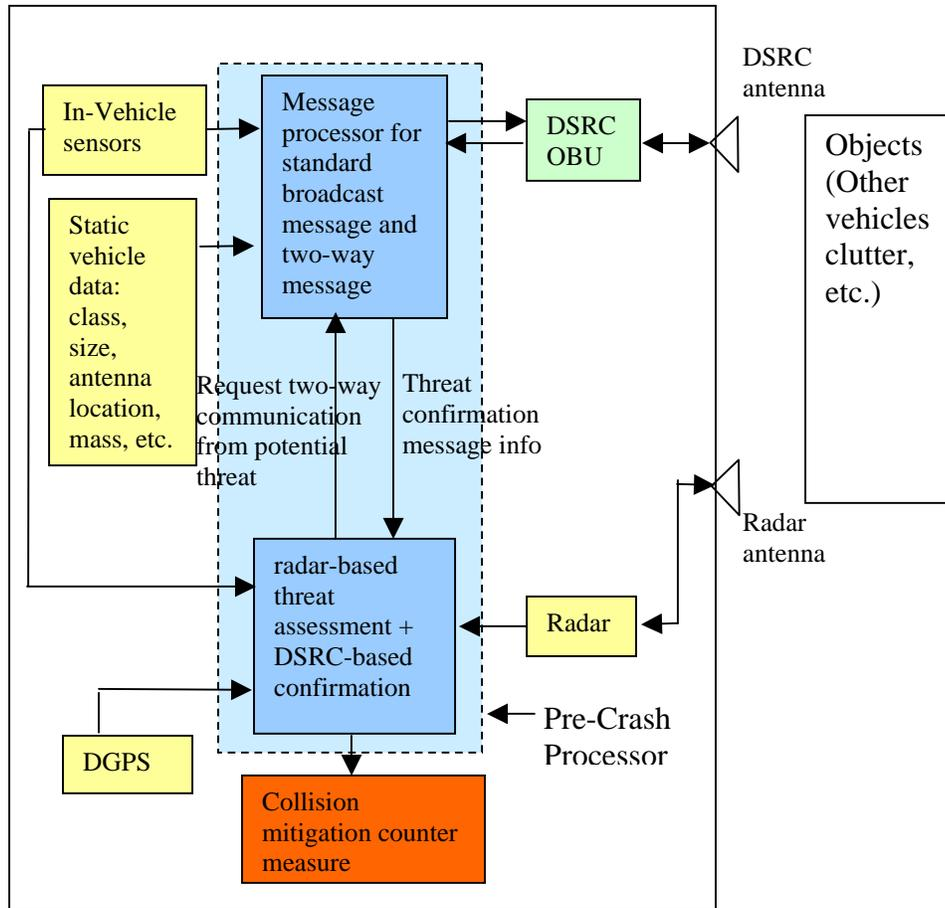
**Figure 4.15 Example of Block Diagram for Cooperative Collision Mitigation System Based on Pre-Crash Sensing**
