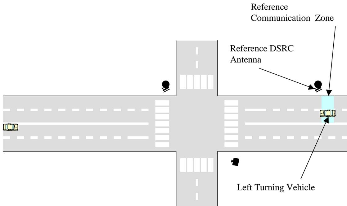
**Figure 4.18 Reference DSRC Communications**
