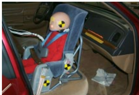
Figure 4. Setup for Reconstruction Test #1200.
