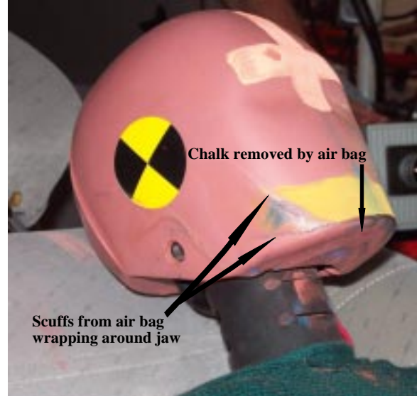
Figure 8. Evidence of air bag "wrapping" around chin on test dummy.
