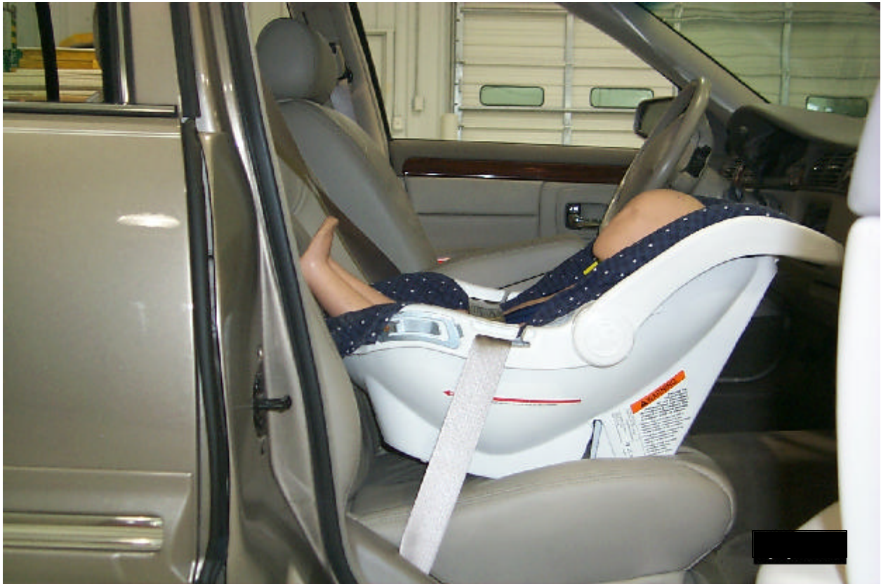
S20.2.1.8 - 12 month CRABI, seat recline = 30°, seat full rearward, 1999 Cadillac DeVille (60-40 split bench)
