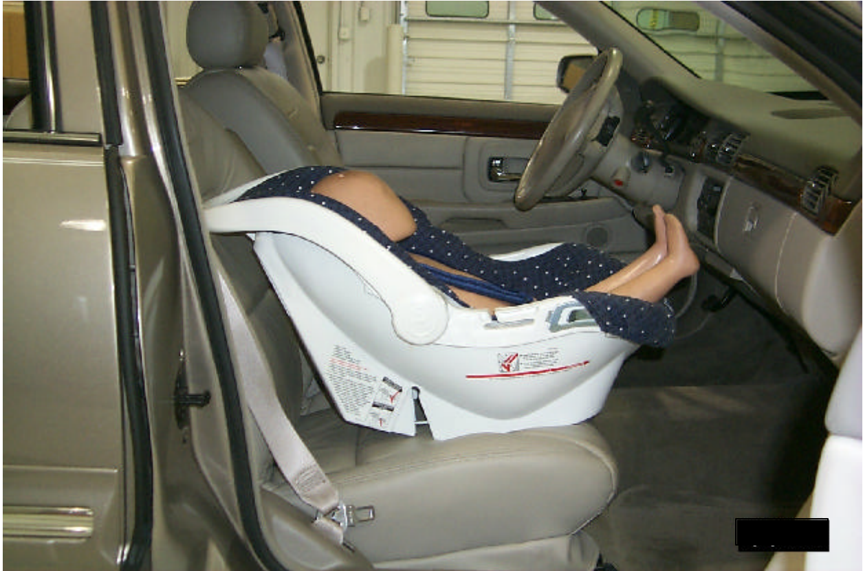
S20.2.2.9 - 12 month CRABI, seat recline = 30°, seat full rearward, 1999 Cadillac DeVille (60-40 split bench)
