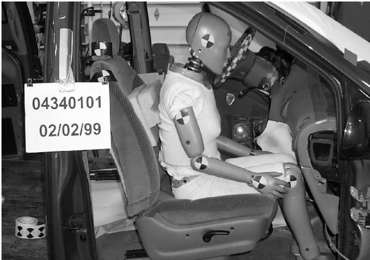
Fig. 5. Typical Test Seating Position.
