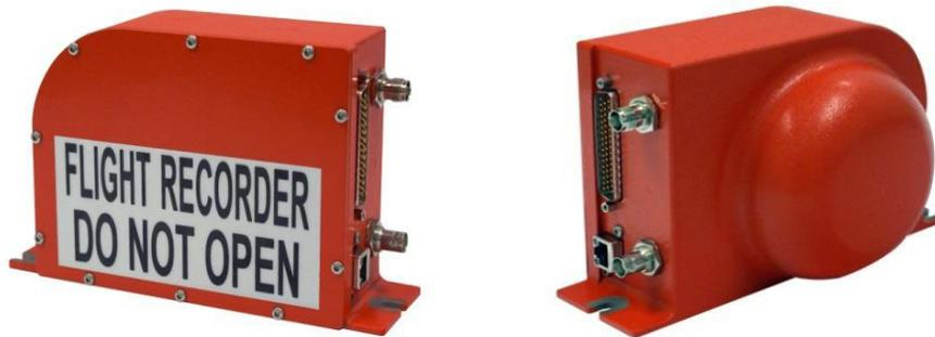
Figure 22. L3ARD lightweight data recorder.
