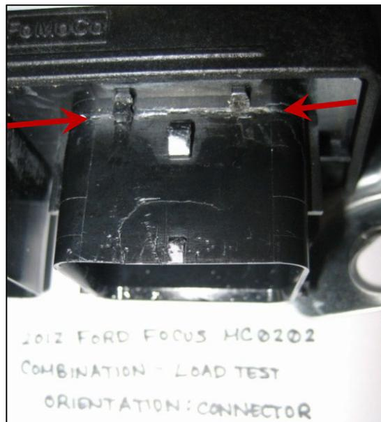
**Figure 17. Broken connector on Ford Focus (MC0202) that hindered initial downloading attempt.**
