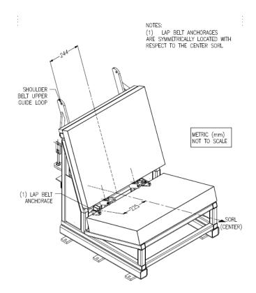
SEAT ORIENTATION REFERENCE LINE AND SEAT BELT ANCHORAGE POINT LOCATIONS ON THE STANDARD SEAT ASSEMBLY Figure 1D
