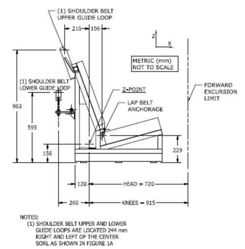
LOCATION OF SHOULDER BELT UPPER AND LOWER GUIDE LOOPS AND FORWARD EXCURSION LIMITS ON THE STANDARD SEAT ASSEMBLY Figure 1E
