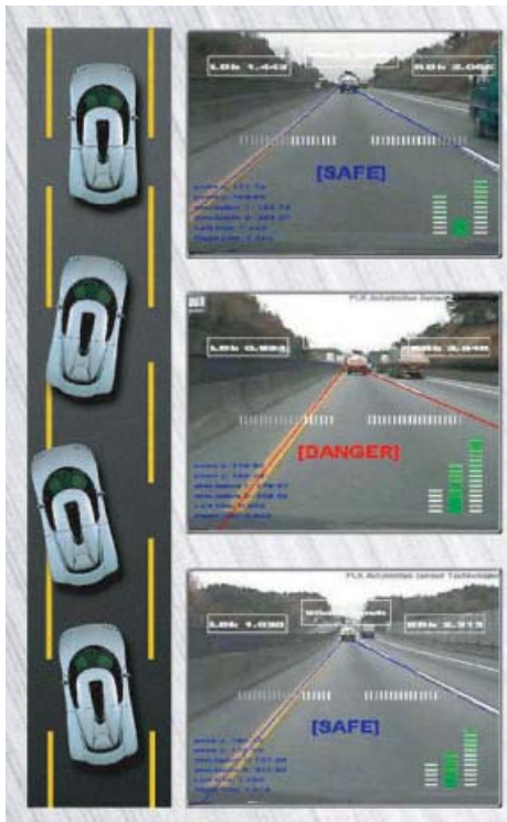
Figure 2.16 How BLS-3000 LDWS Works
