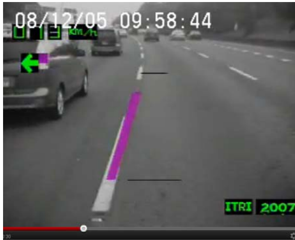
Figure 2.12. MINTRON- Imaged-Based Lane Departure Warning System Operating on Highway
