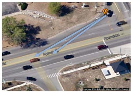
Figure 33 – IMA Scenario Examples: HV Stopped While RV Was Turning Right Onto Far Lane (Imagery ©2014 Google, Map data ©2014 Google. Used with permission.)
