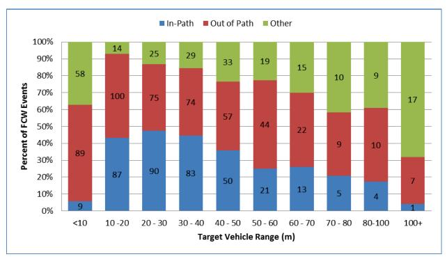
Figure 62. Target Location for FCW Alerts by Target Range
