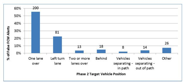
Figure 13. Detailed Breakdown of Phase 2 False FCW Alerts
