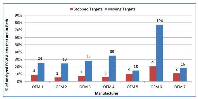
Figure 17. Percentage of FCW Alerts Issued for In-Path Targets by OEM and Target Vehicle Motion
