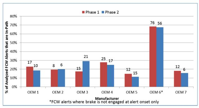
Figure 15. In-Path Percentage of FCW Alerts Issued Without Brake Engaged at Alert Onset
