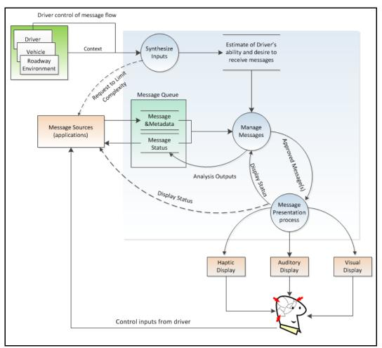
Figure 12-3. Exploded view of the dynamic integrator (within the blue box) illustrating management of three aspects of the integration architecture: synthesis of input, management of message traffic, and presentation of information to drivers.
