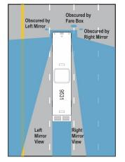
Figure 12-15. Depiction of typical transit bus blind spots (adapted from Thorpe, Duggins, McNeil, & Mertz, 2002).
