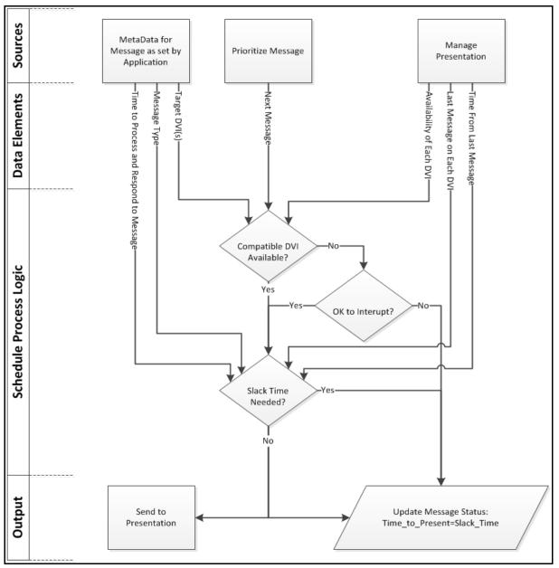
Figure 12-10. Example of a Schedule process applied to messages that are intended for the driver.
