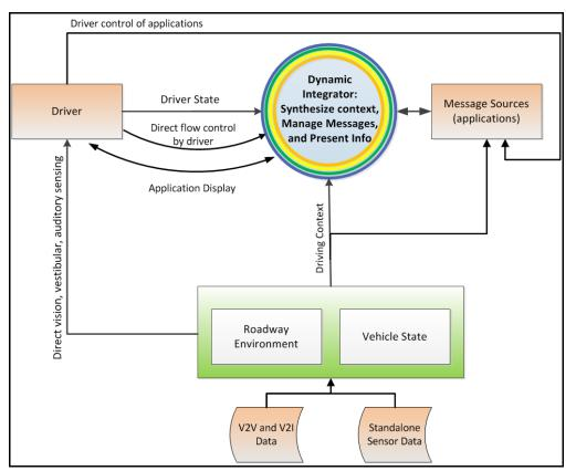
Figure 12-2. Context diagram for Connected Vehicle integration process.
