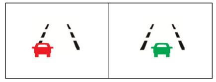
This image shows a hypothetical lane centering status display. The left image indicates that the car is not centered in the lane. The non-centered status is provided through position of the car on the lane display, as well as through the red color of the car. The right image indicates that the car is centered in the lane. The centered status is portrayed through showing the car in the center of the lane display and through the green color of the car.
