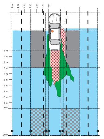
The purpose of the diagram for this topic is to demonstrate the extent that standardized blind-spot warning zones match up with actual measurements of driver visibility of the sides and rear areas of a vehicle.
