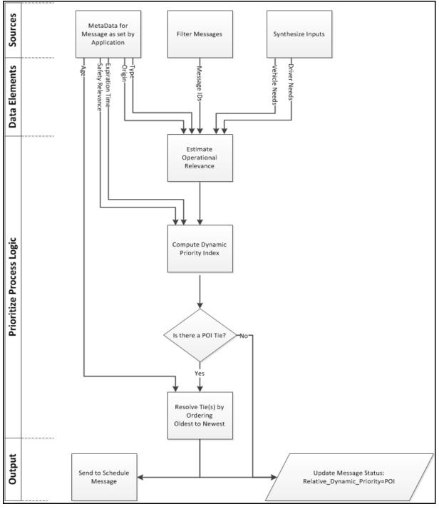
Figure 12-9. Example of a Prioritize process applied to messages that are intended for the driver.
