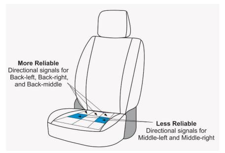
Although the research examining effectiveness of delivering spatial/directional information to a driver through a vibrotactile seat is quite limited, there is sufficient information within the literature to provide information on design elements.
