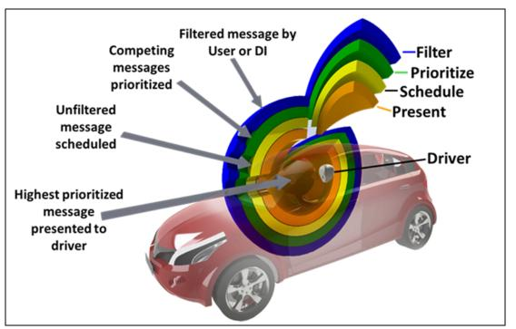
Figure 12-4. Connected Vehicle dynamic integrator model.
