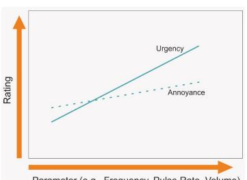
Example of one analytical method for estimating the effect on perceived urgency and annoyance by varying sound parameters.
