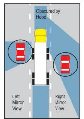
Figure 12-14. Depiction of heavy truck blind spots (adapted from FMCSA, n.d.).
