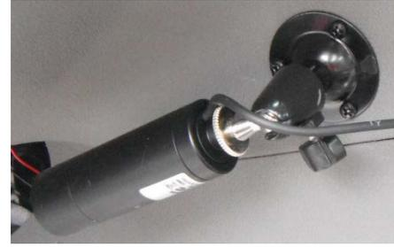
Figure 2. Weldex WDB 5407 SS bullet camera.
