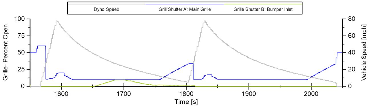
Figure 48: Grille Shutter operation on the dynamometer coast downs
