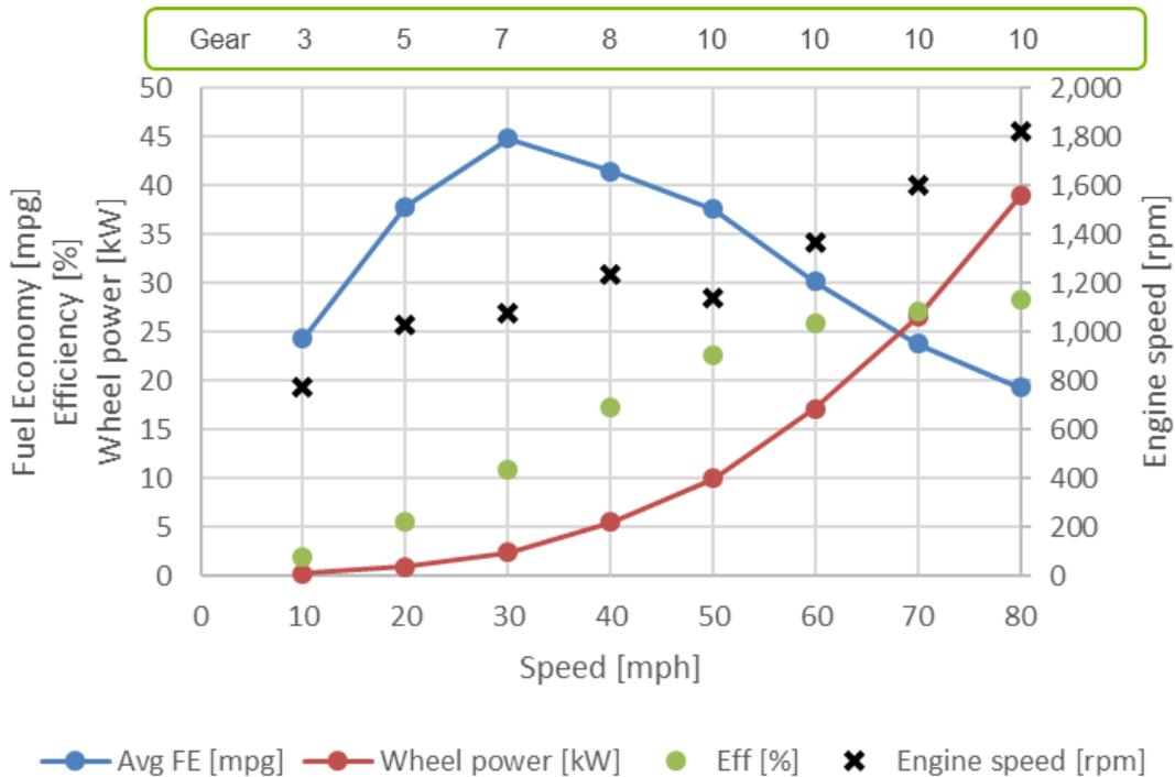
Figure 22: Steady state speed fuel economy with other powertrain measurements on Tier 2 – 93 AKI fuel
