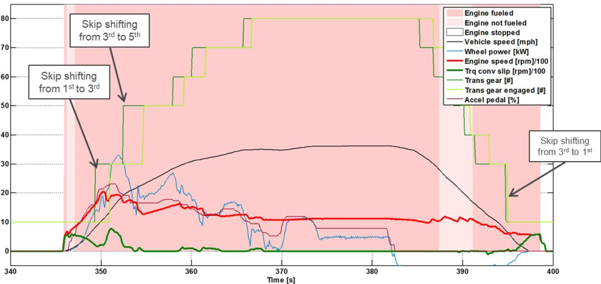
Figure 9: F-150 shift operation on cold start UDDS
