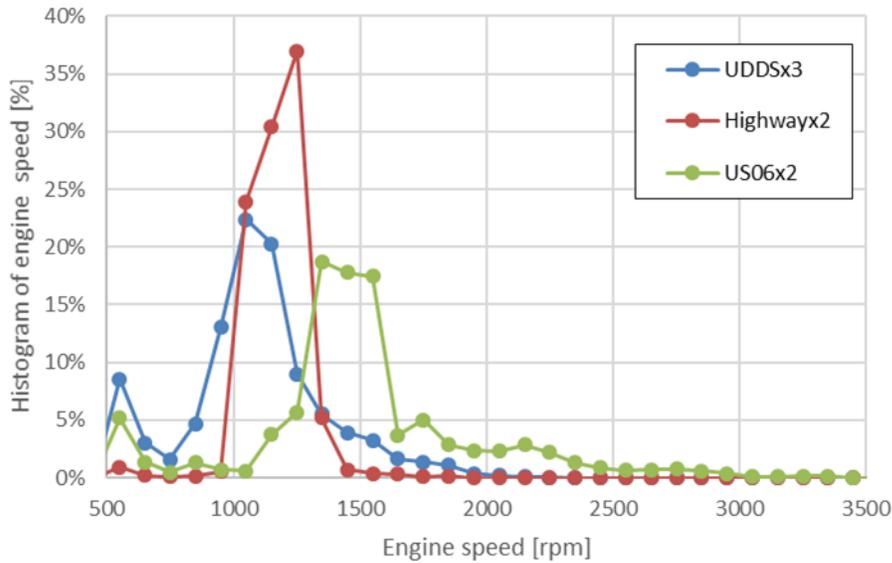
Figure 14: Engine speed histogram for certification cycles
