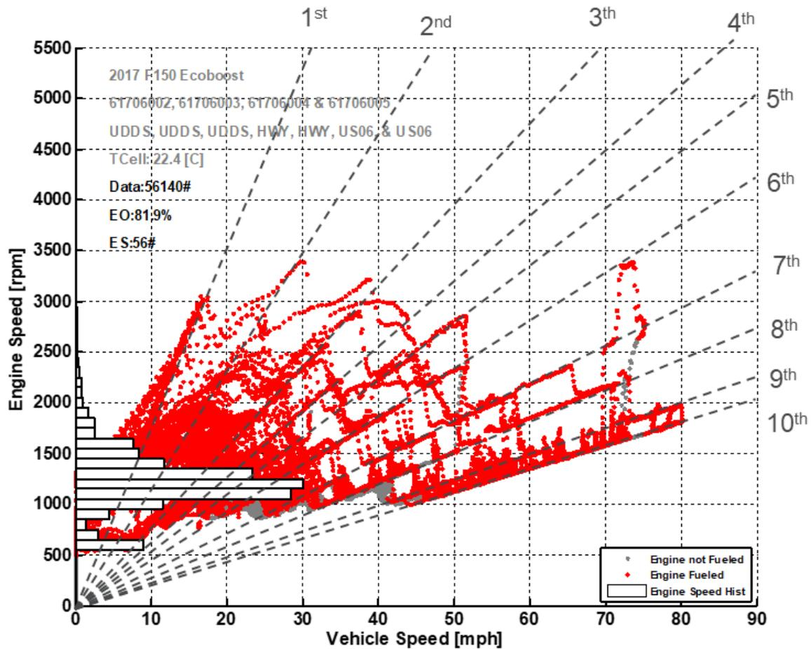
Figure 19: 10-speed transmission shift ratios and engine speed usage
