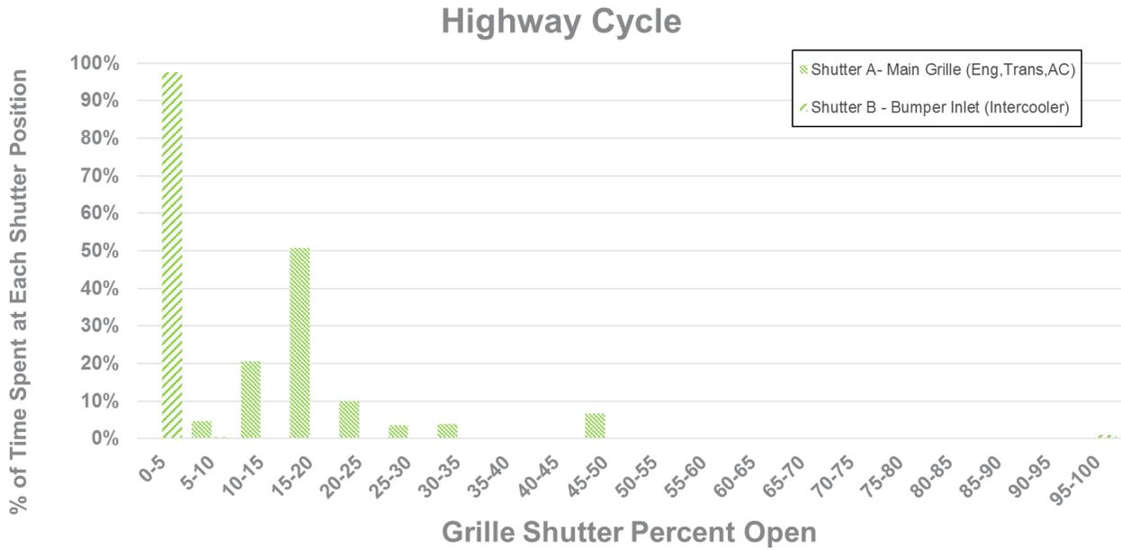
Figure 54: Active grille shutter operation on the HWY cycle
