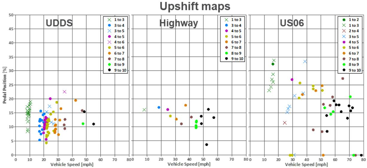
Figure 20: Transmission shift operation on certification drive cycles
