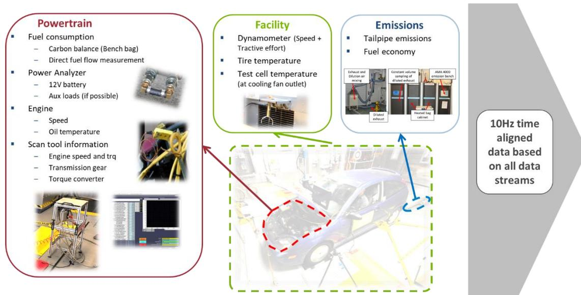
Figure 3: Overview of general instrumentation for conventional vehicle
