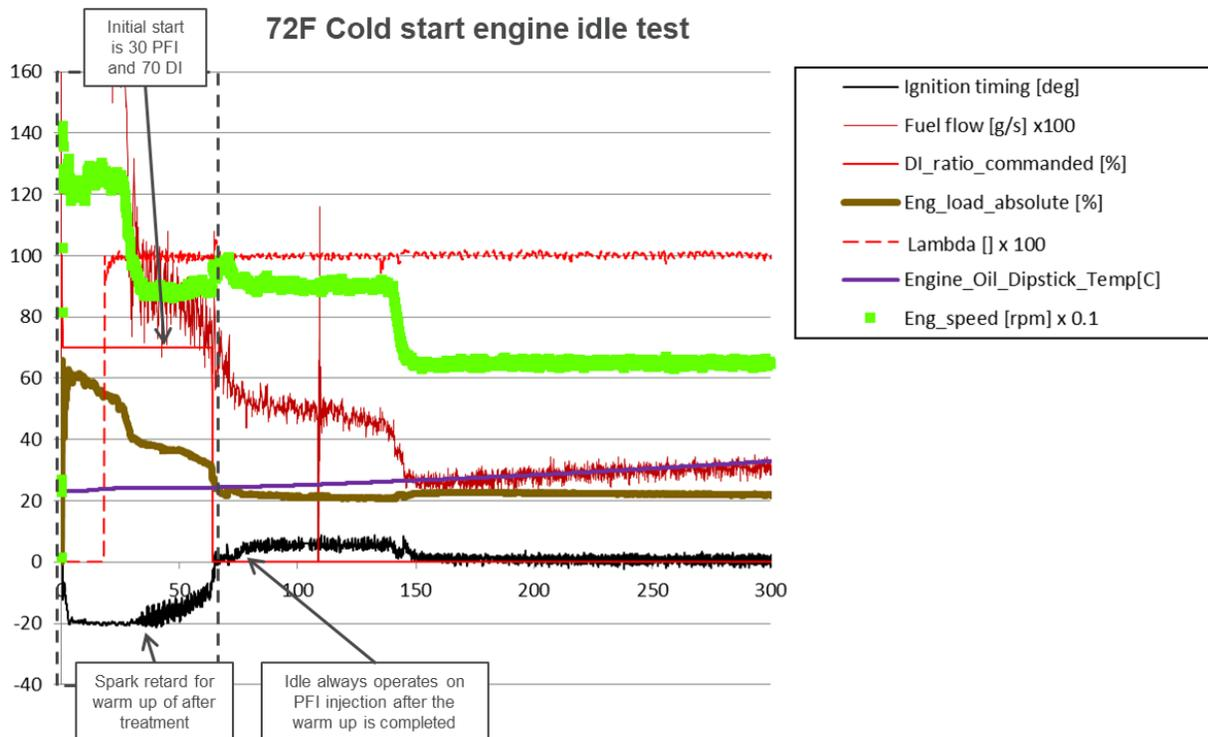
Figure 26: Analysis on a cold engine start and idle
