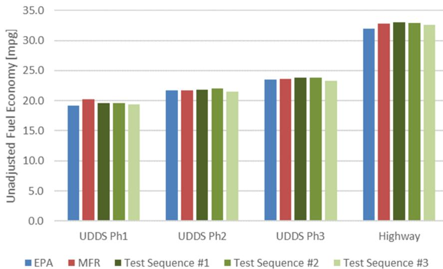
Figure 10: Raw fuel economy results for the UDDS and Highway certification cycles from EPA and Argonne
