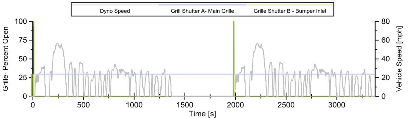
Figure 55: Active grille shutter operation on the UDDS at 20° F
