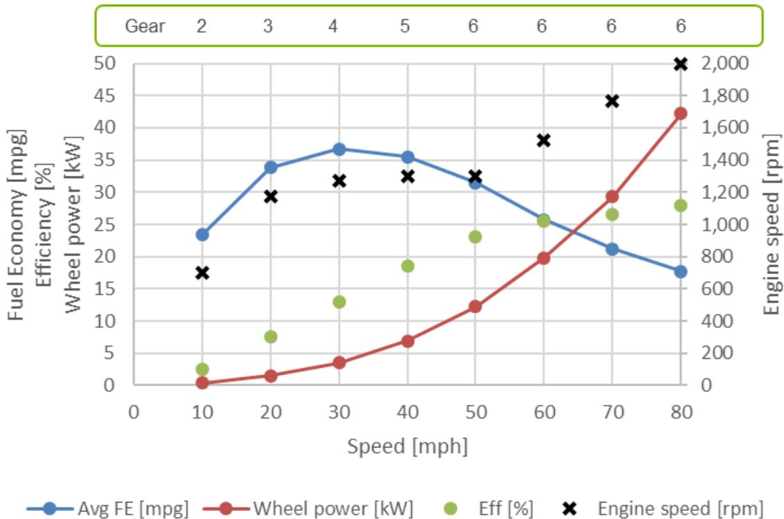
Figure 23: 2012 Ford F150 3.5L EcoBoost Steady state speed fuel economy with other powertrain measurements
