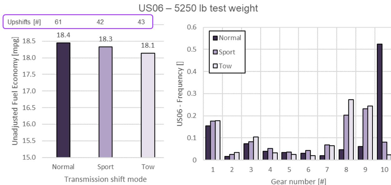
Figure 43: Fuel economy results and transmission gear histogram for different transmission shift modes on US06
