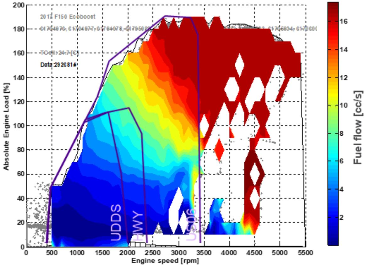
Figure 32: Fuel flow map as a function of the engine speed and load
