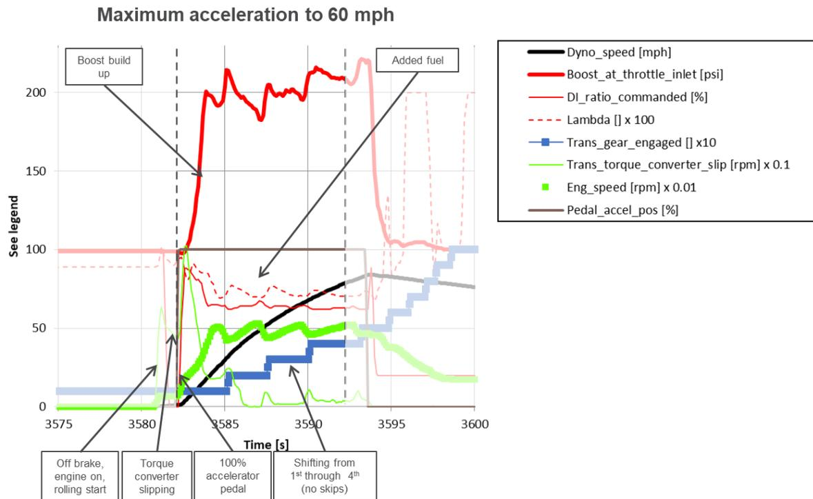
Figure 24: Powertrain operation during maximum acceleration
