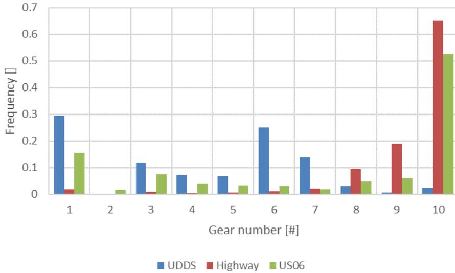
Figure 17: Histogram of gear usage on certification drive cycles
