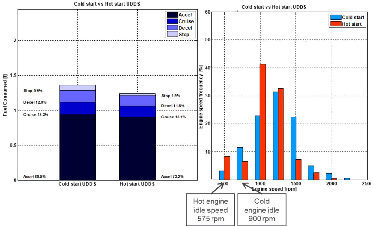
Figure 13: Fuel consumption inventory by drive mode and engine speed operation comparison between cold and hot start UDDS
