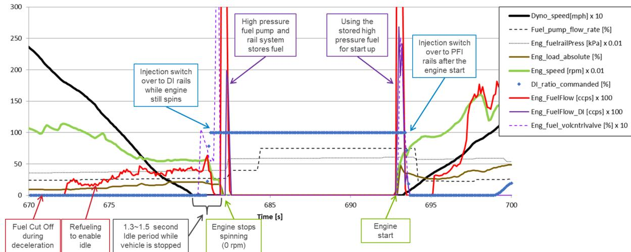
Figure 28: Mechanics of the engine start stop system
