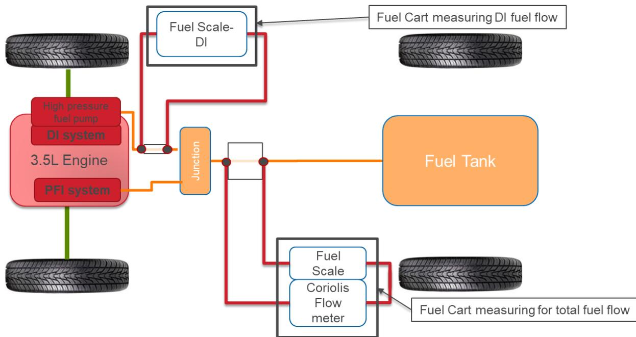
Figure 7: Fuel flow instrumentation diagram
