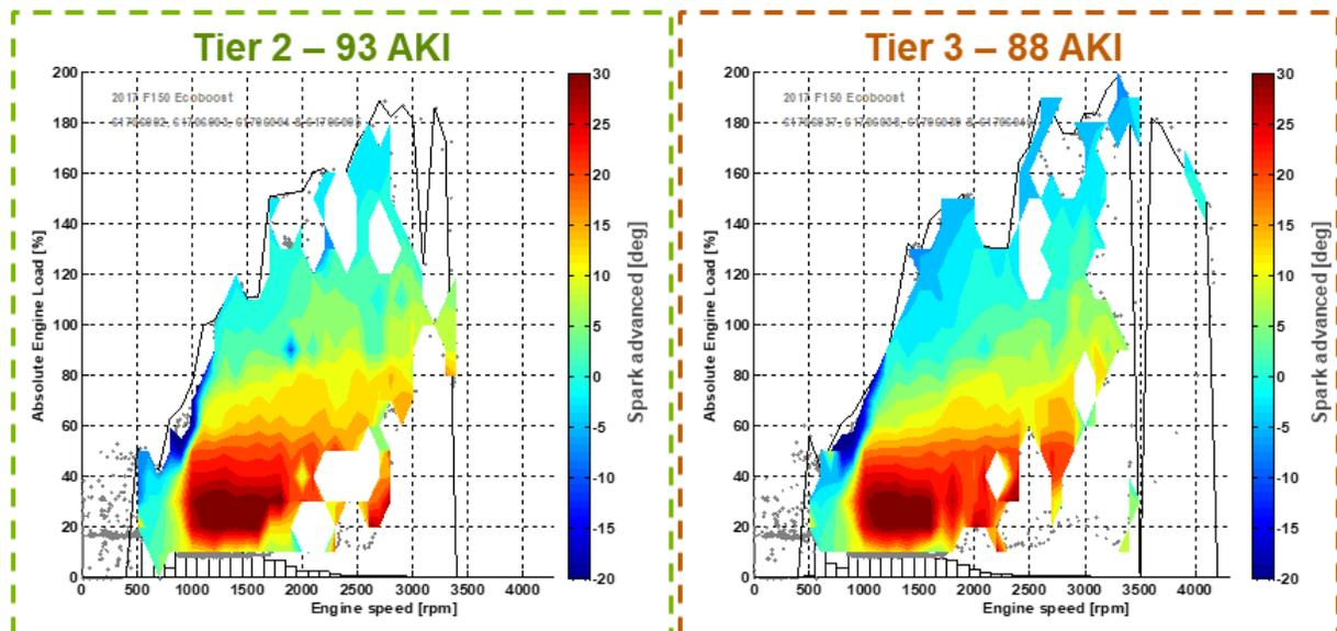
Figure 41: Spark advance comparison between Tier 2 and Tier 3 fuels
