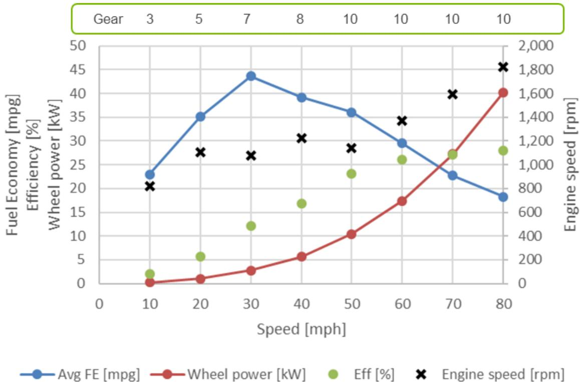
Figure 42: Steady state speed fuel economy with other powertrain measurements on Tier 3 – 88AKI
