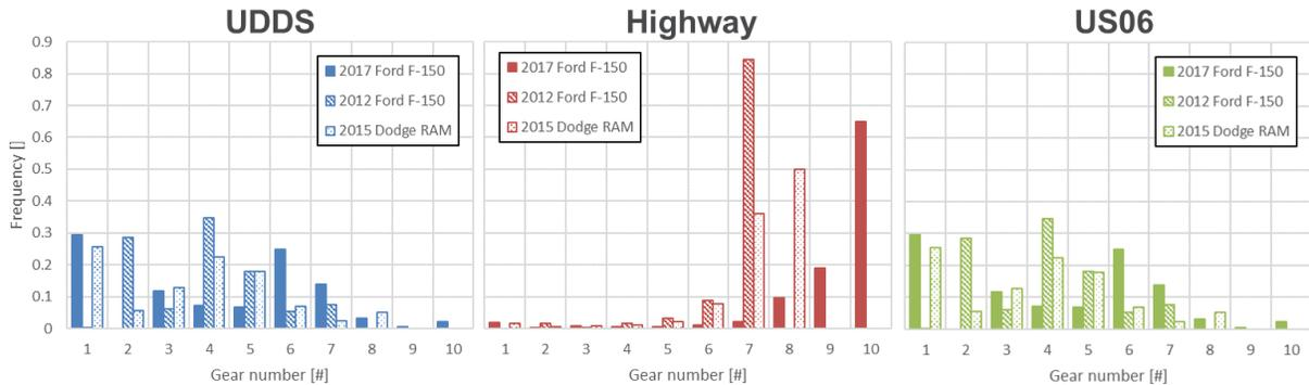
Figure 18: Histogram of gear usage for several vehicles across the certification drive cycles
