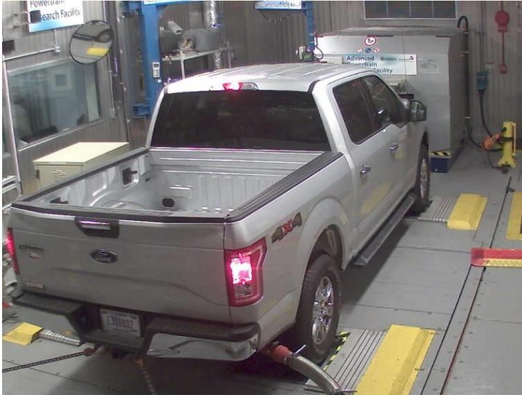
Figure 6: Ford F-150 test vehicle mounted to the chassis dynamometer inside of the test cell. Note that even though the front wheels are on the rolls in this picture, the front wheels were never spinning for duration of the testing.
