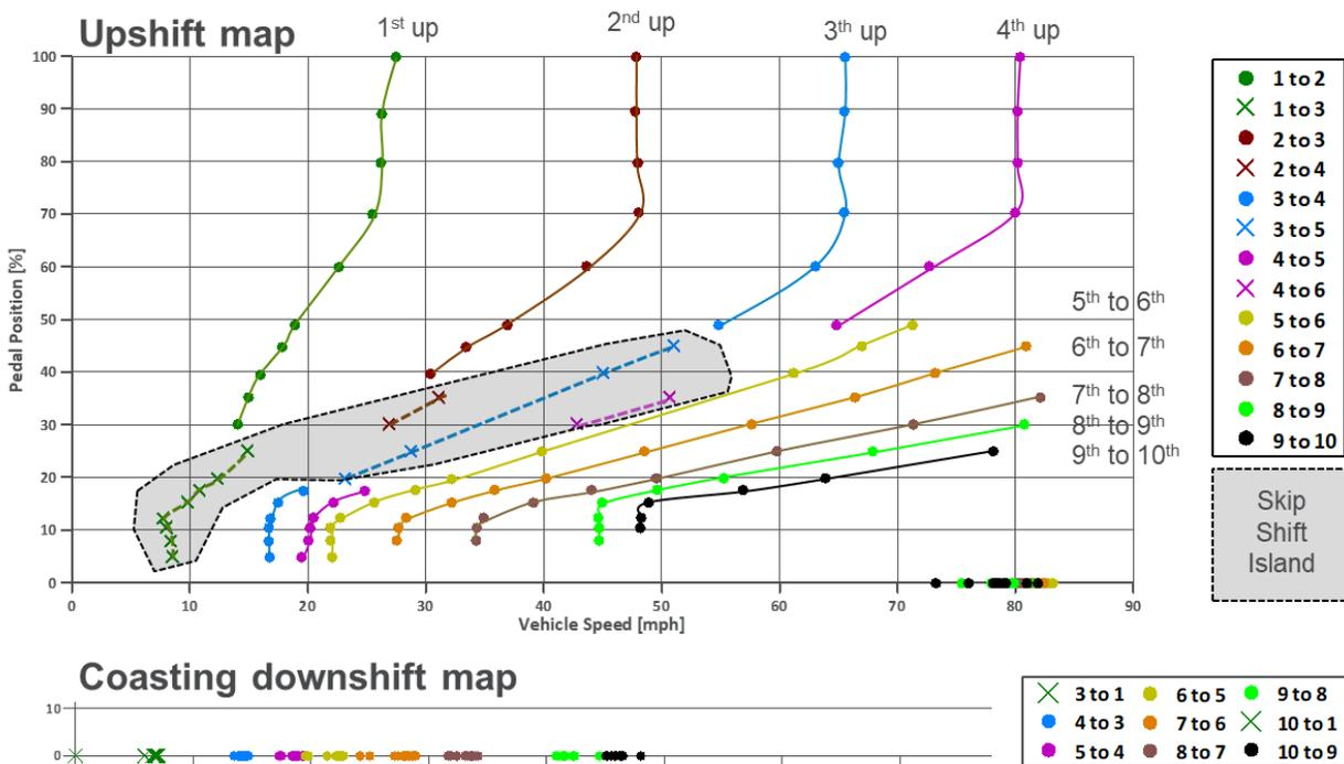
Figure 34: Shift strategy for the 10-speed automatic transmission (including skip-shifting)
