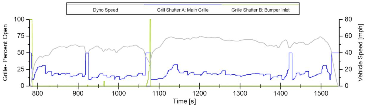
Figure 53: Highway Cycle Active Grille Shutter Commanded Operation
