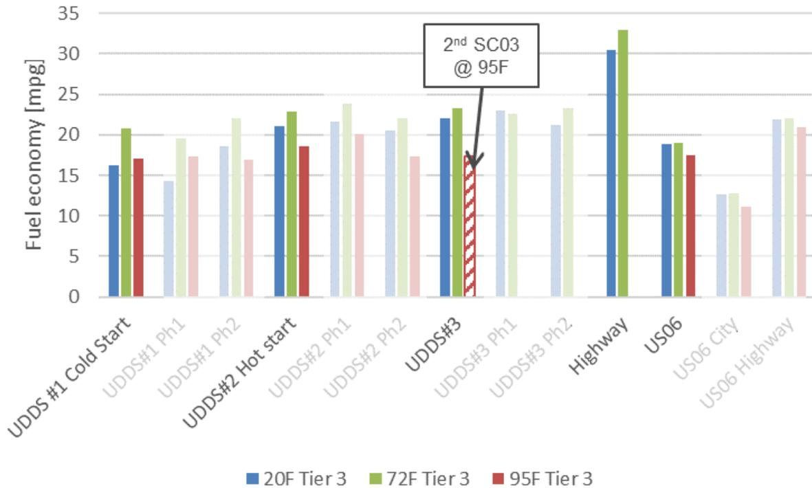
Figure 36: Raw fuel economy results for certification cycles across different temperature conditions
