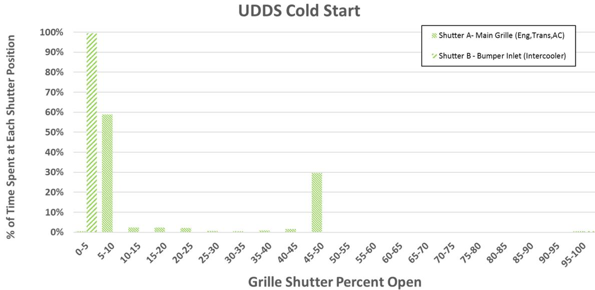
Figure 50: Histogram of Active Grille Shutter Operation on a UDDS Cold Start Test
