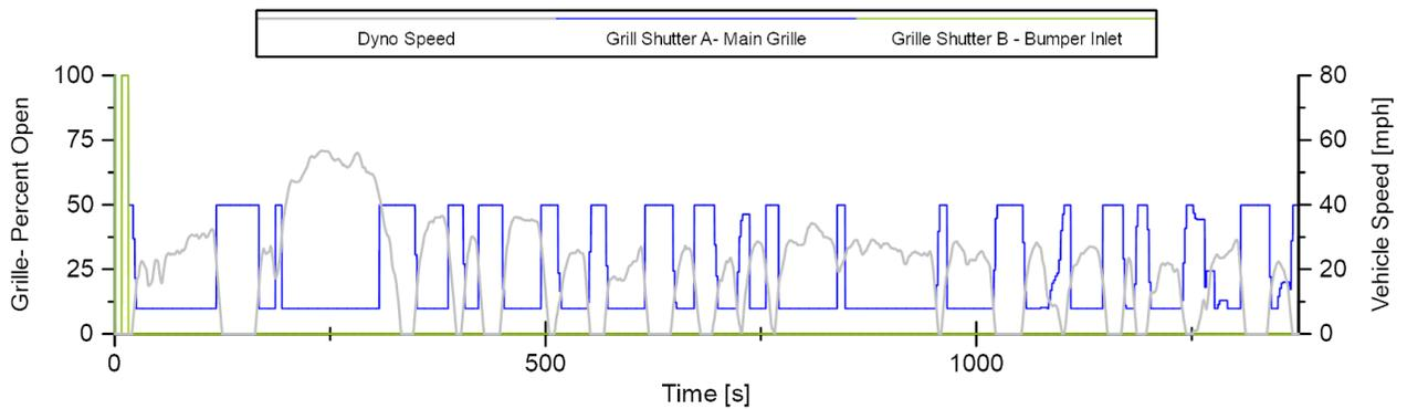
Figure 49: UDDS Cold Start Grille Shutter Commanded Operation
