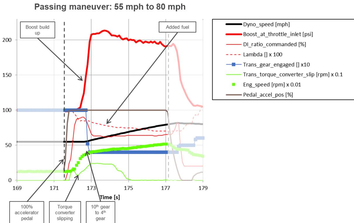
Figure 25: Powertrain operation during the 55 mph to 80 mph passing maneuver
