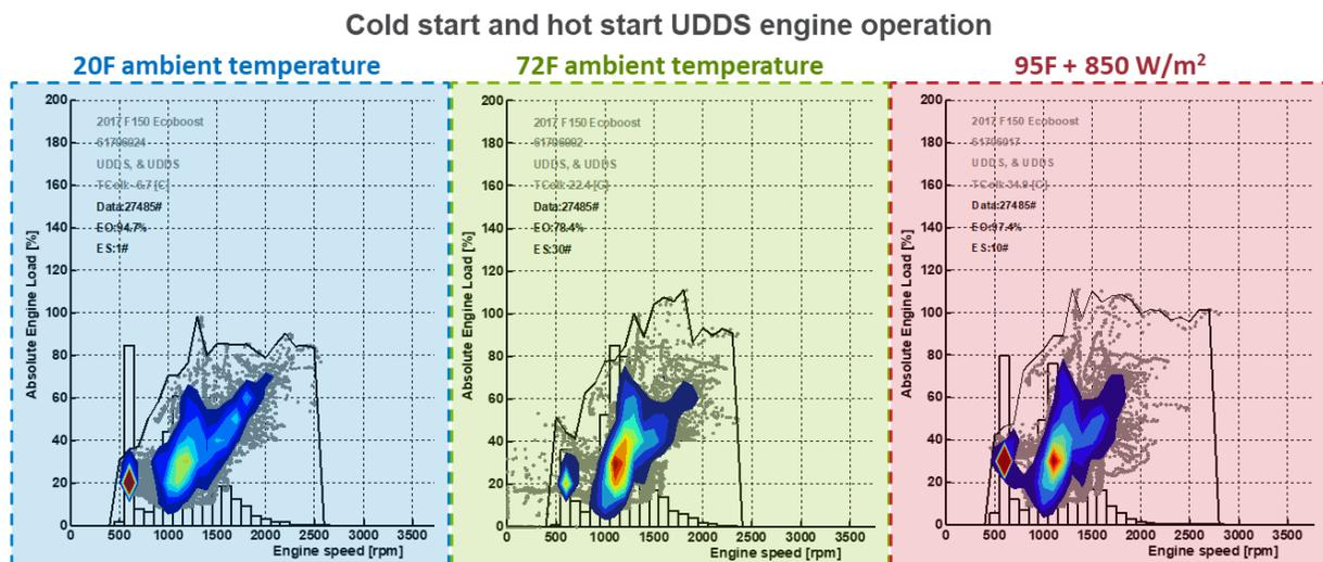
Figure 37: Engine operation on the UDDS across different temperatures
