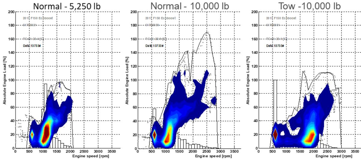
Figure 46: Engine operation for the different payload conditions
