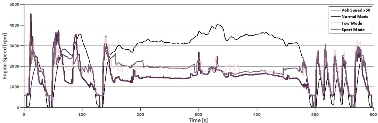
Figure 44: Engine speed differences on US06 for different transmission shift modes
