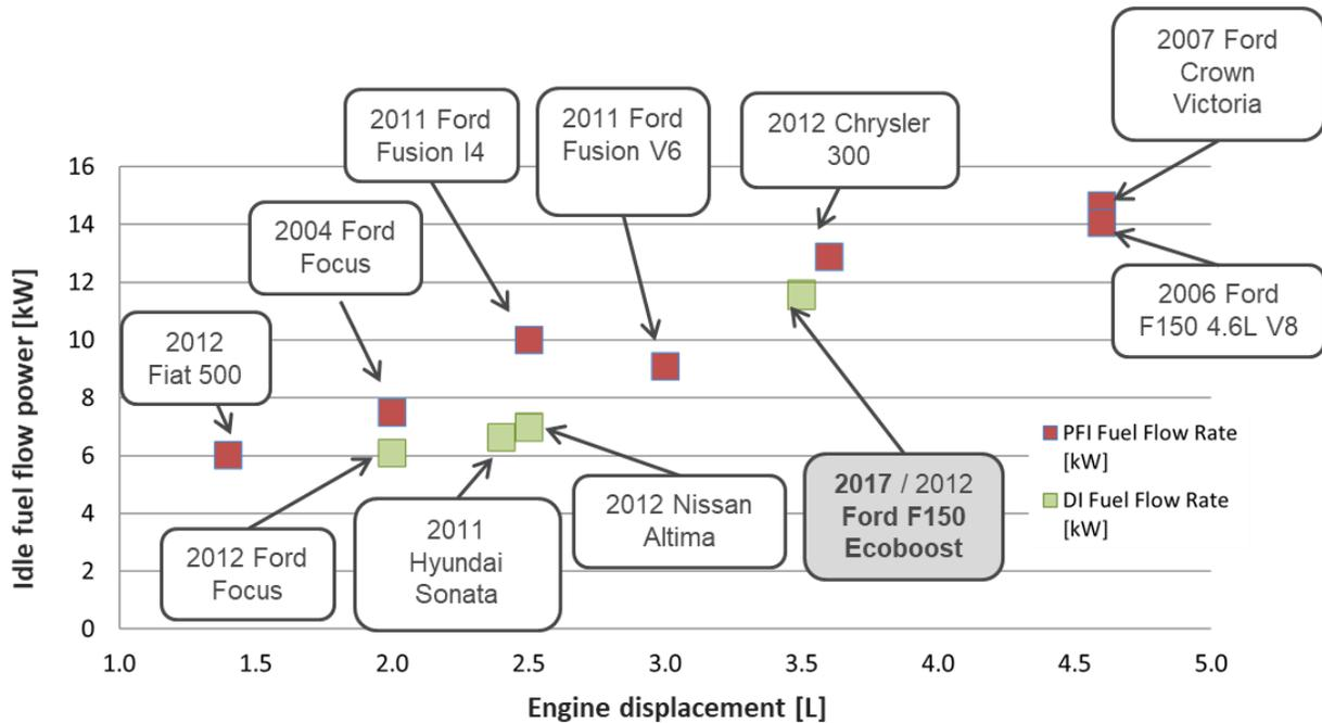
Figure 27: Idle fuel flow rate comparisons
