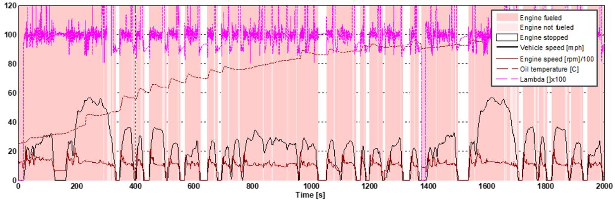
Figure 21: Engine start stop behavior on cold start UDDS
