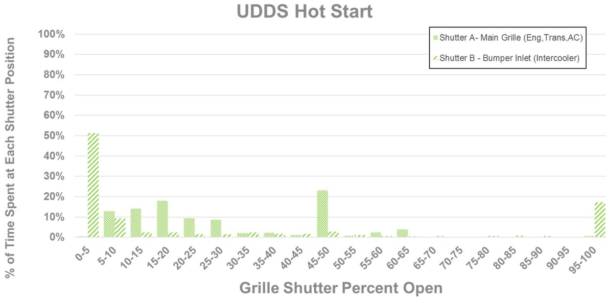
Figure 52: Active grille shutter operation on the UDDS Hot Start test
