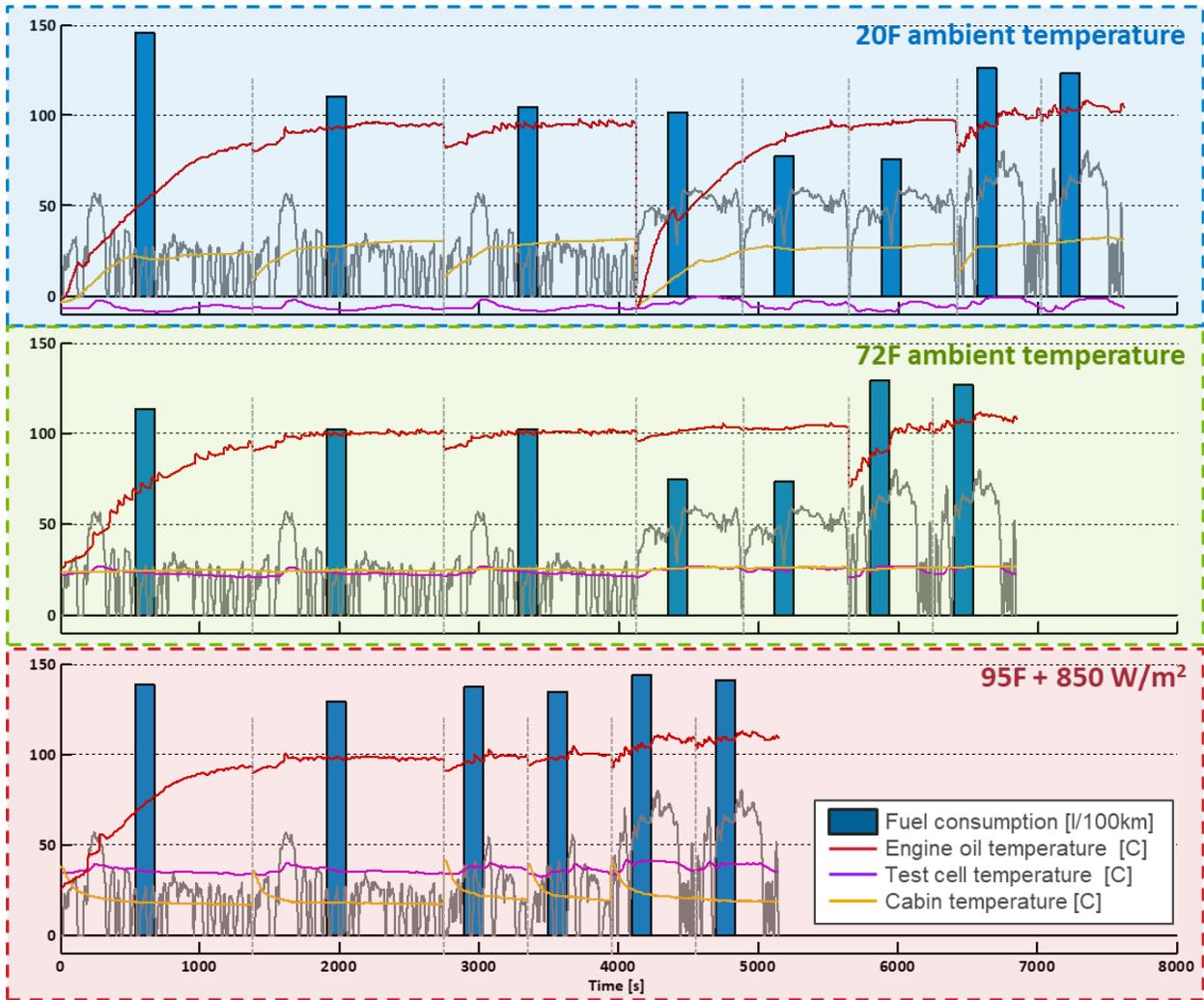
Figure 38: Powertrain and cabin temperature profits across different temperature
