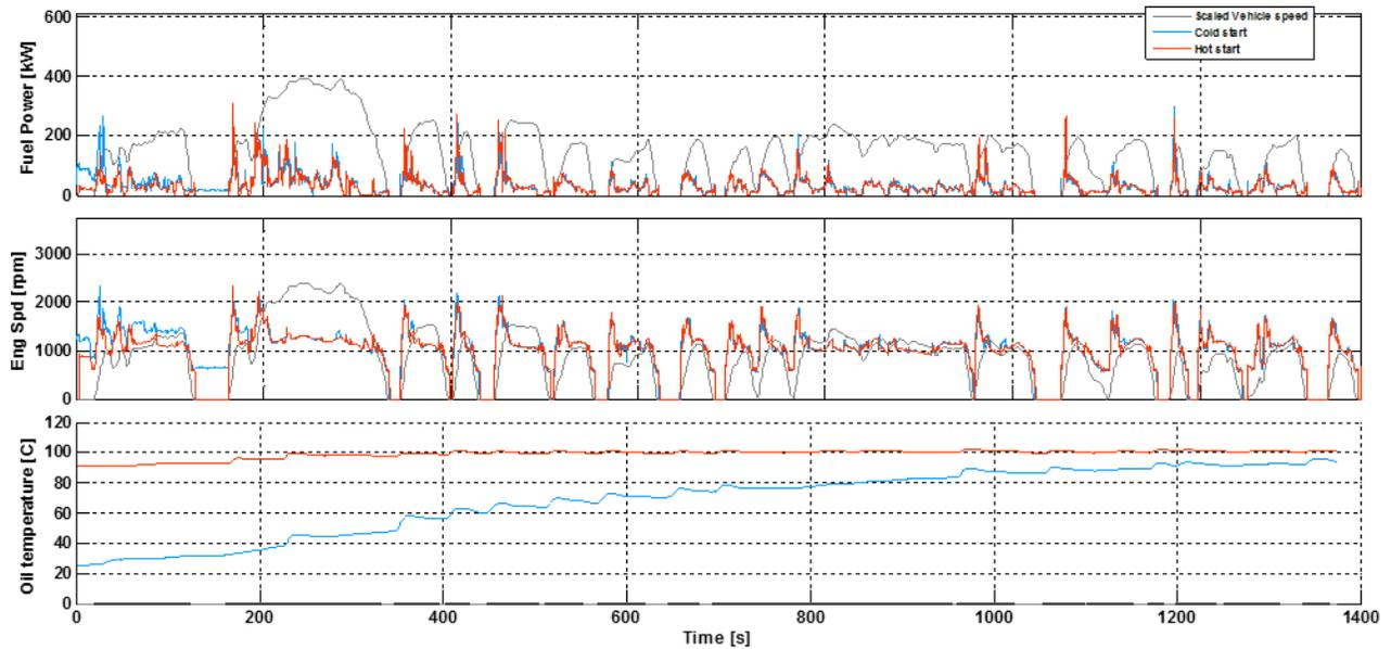
Figure 12: Comparison of powertrain operation on a cold start UDDS and a hot start UDDS
