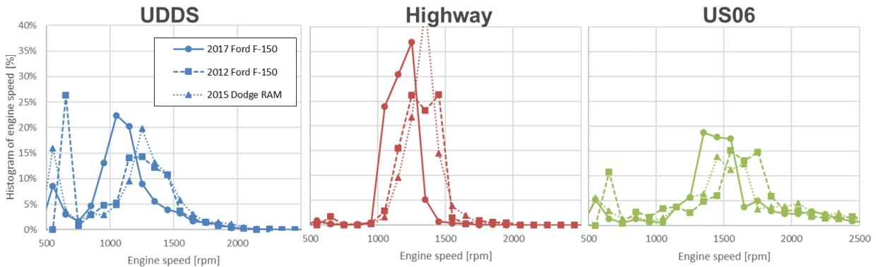
Figure 15: Engine speed histograms of comparison vehicles on certification cycles
