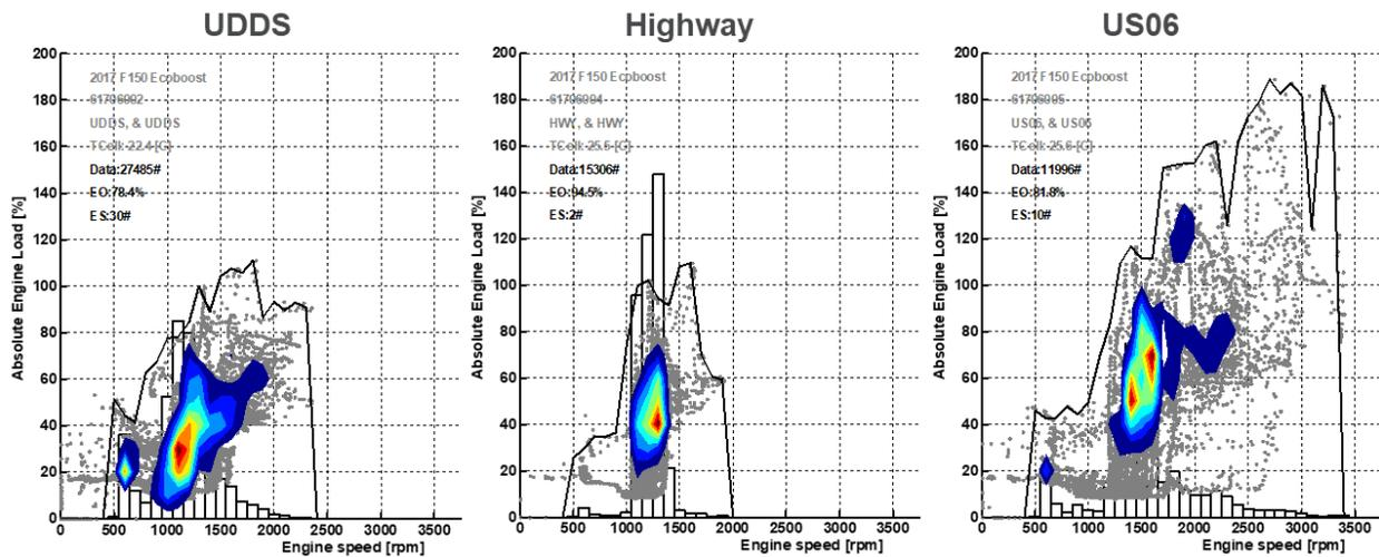
Figure 16: Engine operating area on certification drive cycles
