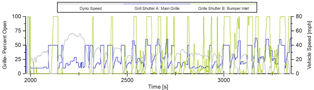
Figure 51: UDDS Hot Start Cycle Active Grille Shutter Commanded Operation
