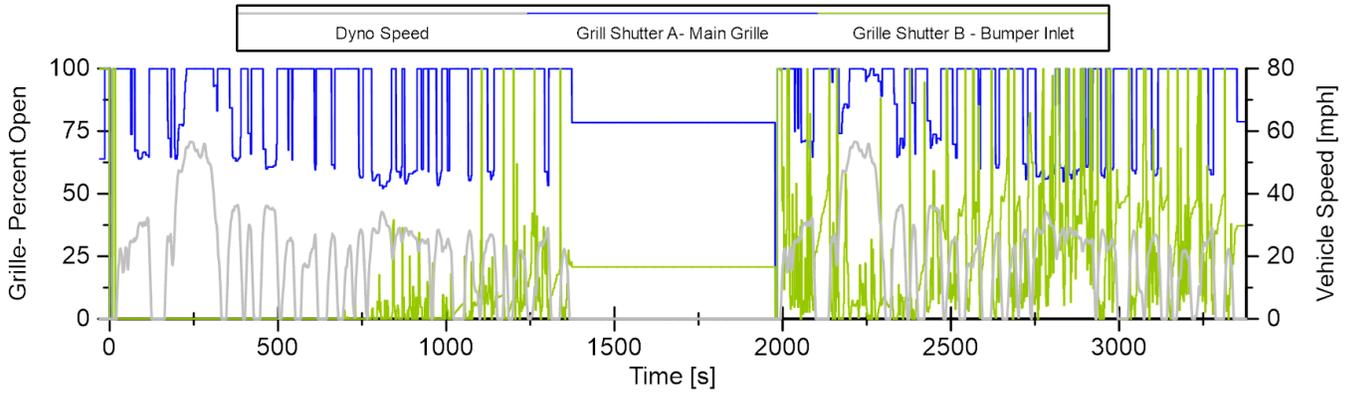
Figure 56: Active grille shutter operation on the UDDS test at 95° F with solar emulation
