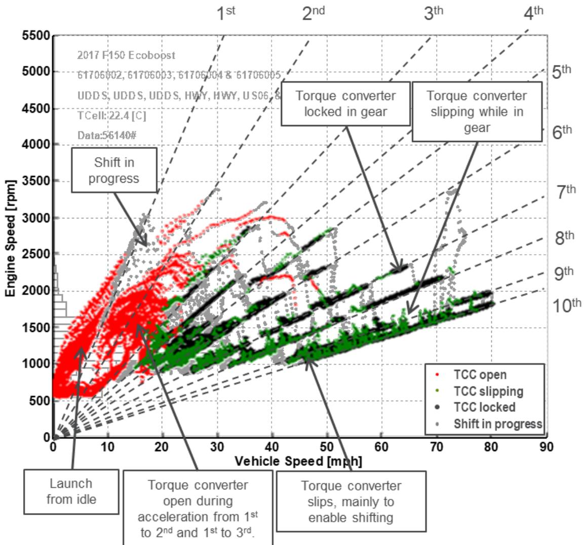
Figure 35: Torque converter operation on certification drive cycles (UDDS, Highway and US06)
