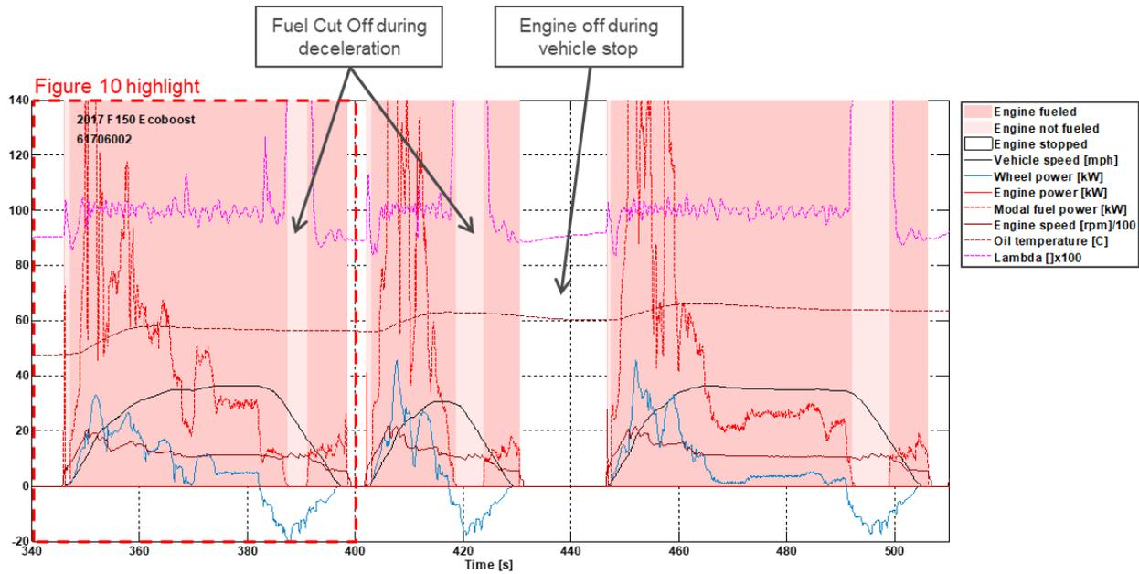
Figure 8: F-150 powertrain operation on cold start UDDS
