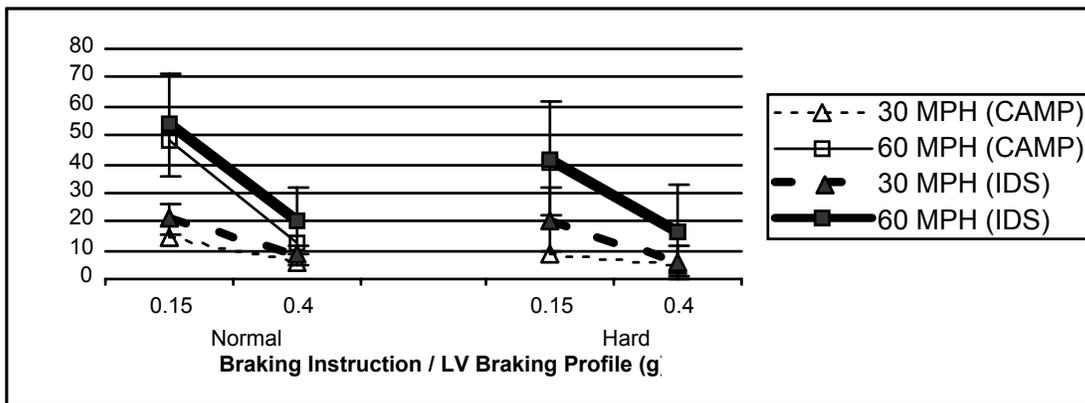
**FIGURE 7. Mean end range as a function of braking instruction, LV braking profile, and speed condition (CAMP data obtained from Figure 3-13).**
