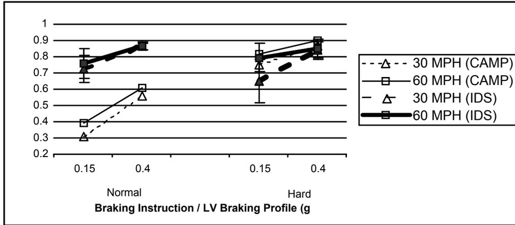
**FIGURE 5. Mean peak deceleration of the SV as a function of braking instruction, LV profile, and speed condition (CAMP data obtained from Figure 3-9).**
