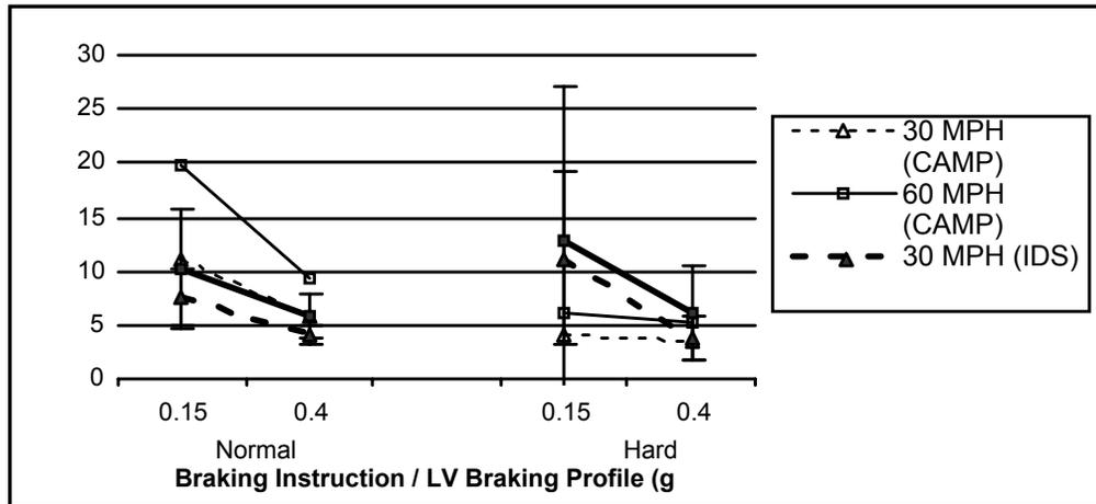
**FIGURE 3. Mean TTC at SV braking onset as a function of braking instruction, LV braking profile, and speed condition (CAMP data obtained from Figure 3-21).**
