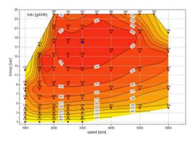
Figure 6-91 - Engine efficiency map for eng14.
