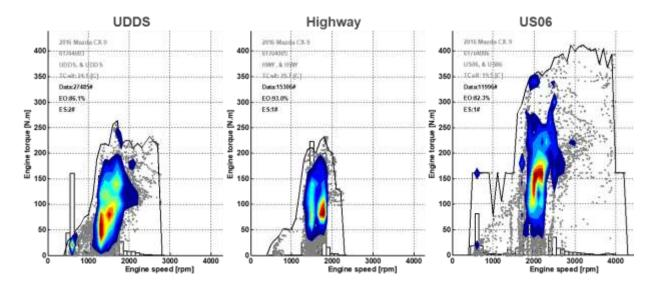
Figure 6-42 - Engine operating Area on certification cycles of 2016 Mazda CX-9 benchmarked by NHTSA $^{200}$
