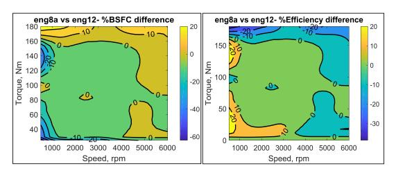
Figure 6-82 - incremental BSFC and thermal efficiency difference between ENG8A versus  $\hbox{ENG12}$
