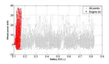
Figure 6-21 - Engine-On Condition – 2017 Prius Prime Example Based on 25 Test Cycles
