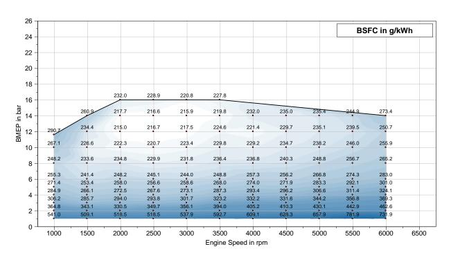
Figure 6-112 - IAV's 2-step VCR engine 26a in 12:1 CR mode
