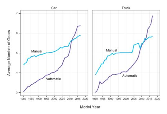
Figure 6-123 - Average Number of Transmission Gears for New Vehicles<sup>257</sup>
