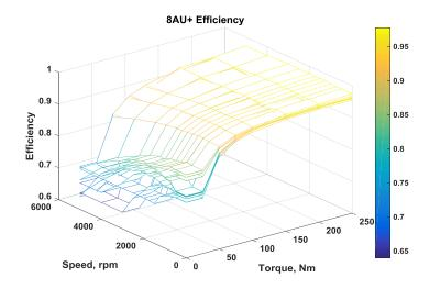
Figure 6-132 - Efficiency map - 8-speed automatic Level 2
