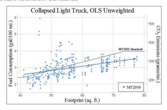
Figure 4-15 - Light Truck Curves Fit with an Unweighted OLS Regression from the Collapsed Dataset
