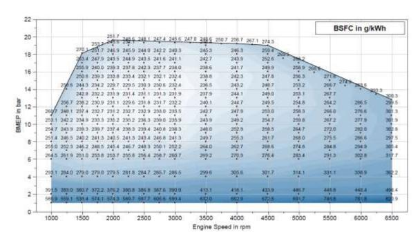
Figure 6-58 - IAV engine 25a BSFC map in 4-cylinder mode
