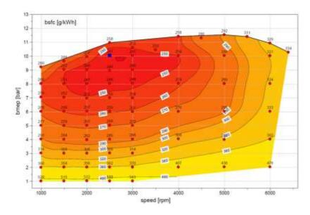
Figure 6-73 - Engine efficiency map for eng5b
