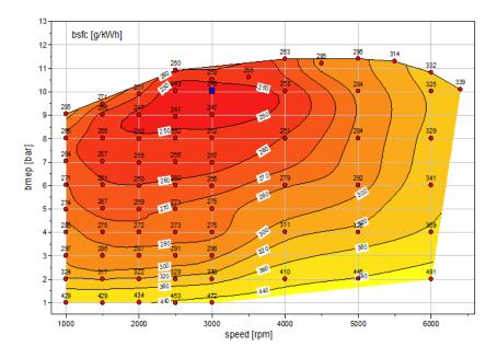
Figure 6-100 - Engine Efficiency map for eng19
