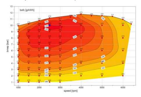
Figure 6-75 - Engine Efficiency Map for eng6a
