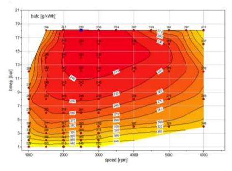
Figure 6-81 - Engine efficiency map for eng12
