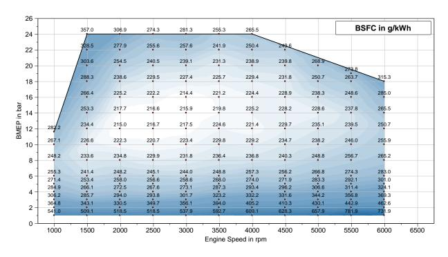
Figure 6-111 - IAV's 2-step VCR engine 26a merged in normal operation
