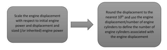
Figure 6-4 - Engine Displacement / Number of Engine Cylinder Relationship
