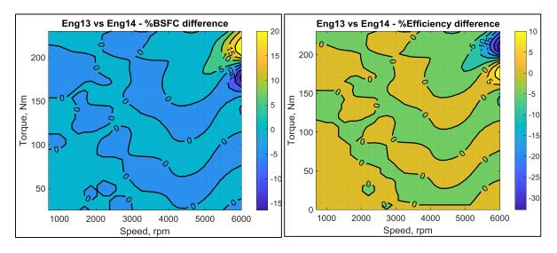
Figure 6-92 shows incremental BSFC and thermal efficiency difference between ENG13 versus ENG14
