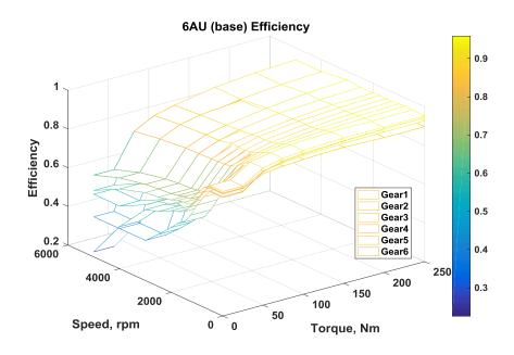
Figure 6-127 - Efficiency map - Base 6-speed automatic level 1
