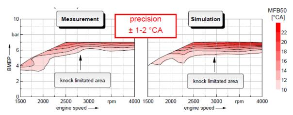
Figure 6-46 - Example of advanced calculation of knock tendency due to cylinder deactivation.
