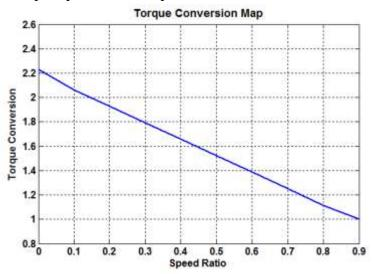
Figure 6-137 - Base vehicle Torque Converter Lock Up map
