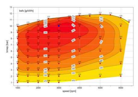
Figure 6-69 - Engine Efficiency Map for Eng03
