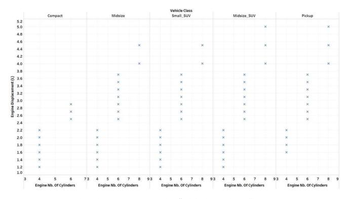
Figure 6-5 - Engine Displacement vs. Engine # of Cylinders from Simulation Results
