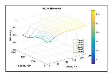
Figure 6-129 - Efficiency map - 6-speed Automatic level 2
