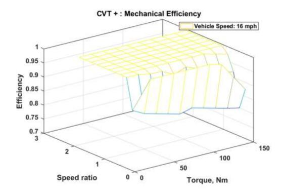
Figure 6-145 - Mechanical Efficiency map of CVT level 2 at 16 mph
