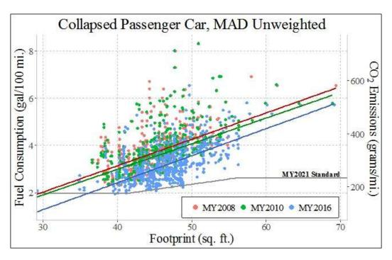
Figure 4-12 - Passenger Car Curves Fit with an Unweighted MAD Regression from the Collapsed Dataset
