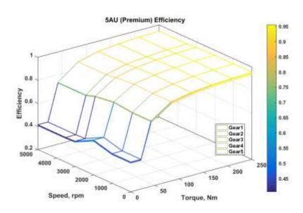
Figure 6-126 - Efficiency map of 5-speed automatic - performance classes
