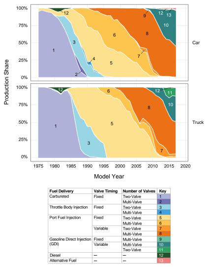
Figure 6-37 - Engine Technology Production Share, 1980-2017<sup>164</sup>
