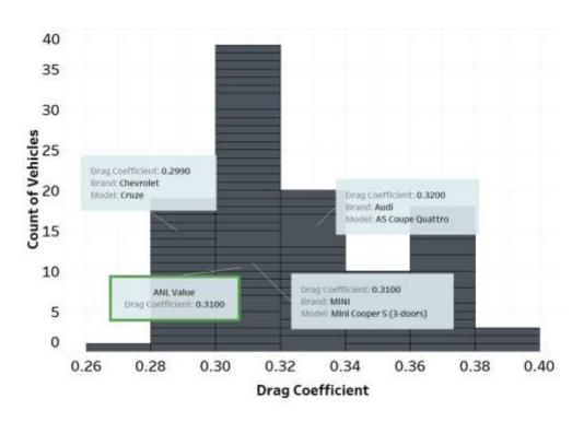
Figure 6-29 - Example of drag Coefficients for Compact Performance Vehicle
