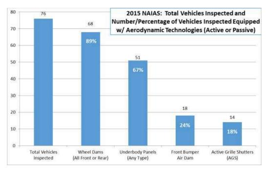
Figure 6-171 - Distribution of Aerodynamic Technologies observed during 2015 NAIAS by EPA staff
