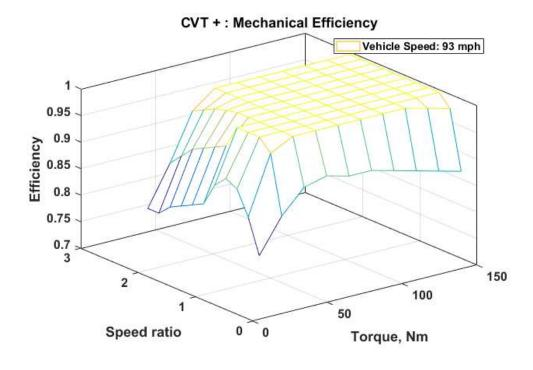
Figure 6-148 - Mechanical Efficiency map of CVT level 2 at 93 mph
