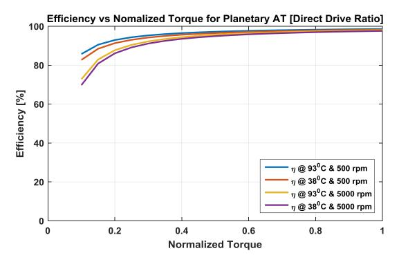
Figure 6-124 - Efficiency for direct drive
