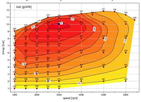
Figure 6-98 - Engine Efficiency map for eng18
