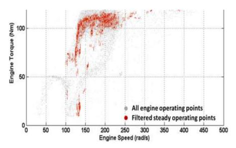
Figure 6-23 - Example of Engine Operating Target – 2017 Prius Prime Example Based on 25 Test Cycles
