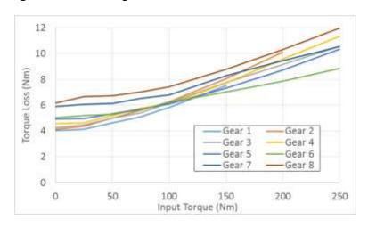
Figure 6-121 - Average Torque Losses in Each Gear for an Eight-Speed 845RE Transmission<sup>252</sup>
