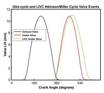
Figure 6-39 - Comparison of The Timing of Valve Events for Otto-Cycle (black and orange lines) and LIVC Implementations of Atkinson- Or Miller-Cycle (black and green lines).
