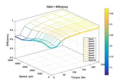
Figure 6-135 - Efficiency map for the 10-speed automatic level 1
