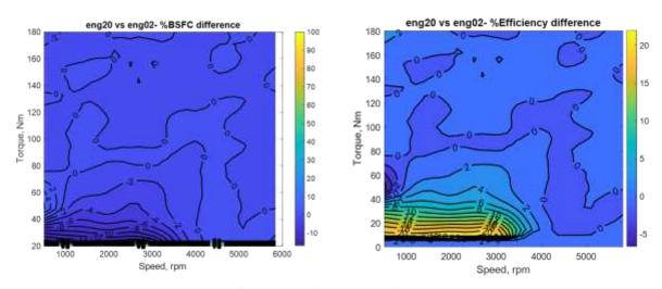
Figure 6-103 - Engine BSFC and efficiency difference between engine 20 and engine 2
