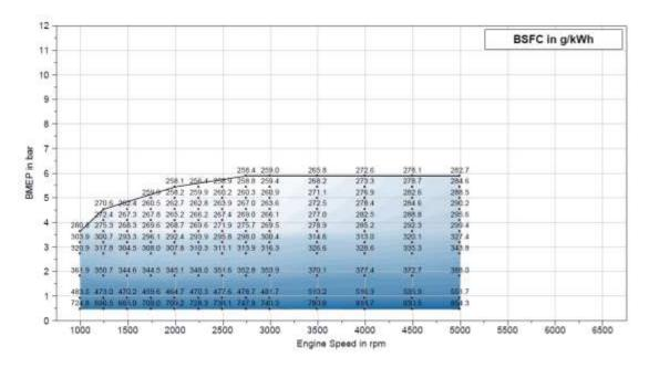
Figure 6-61 - IAV engine 25a BSFC map in 2-cylinder mode
