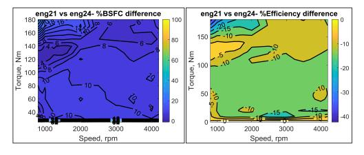
Figure 6-107 shows incremental BSFC and thermal efficiency difference between ENG21 versus ENG24
