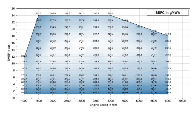
Figure 6-113 - IAV's 2-step VCR engine 26a in 9:1 CR mode
