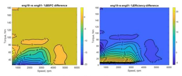
Figure 6-101 - Engine BSFC and Efficiency difference between engine 19 and engine 1
