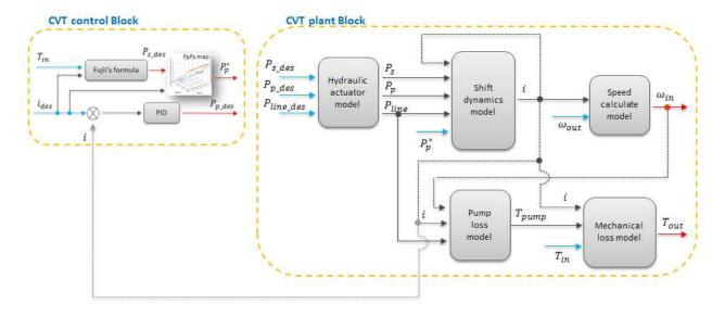
Figure 6-8 - CVT Model Block Diagram
