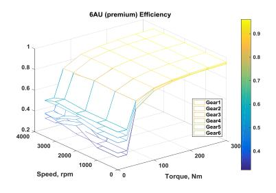
Figure 6-128 - Efficiency map - Performance 6-speed automatic Level 1
