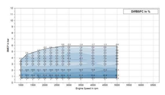
Figure 6-62 - IAV engine 25a incremental difference between 3-cylinder mode versus 2-cylinder mode
