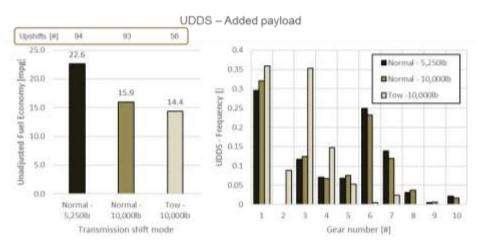
Figure 6-34 - Fuel economy results and transmission gear histogram for different payloads and shift modes on UDDS
