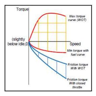
Figure 6-1 - Engine Operating Regions for Throttled Engines
