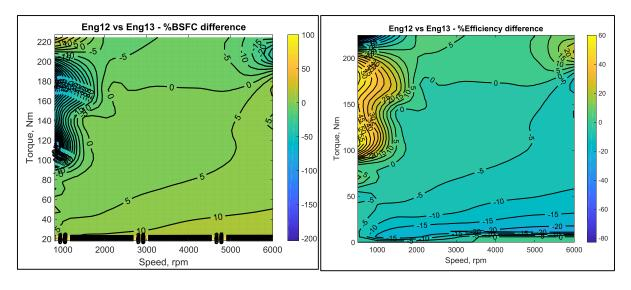
Figure 6-87 - Incremental BSFC and Thermal Efficiency between ENG12 and ENG13
