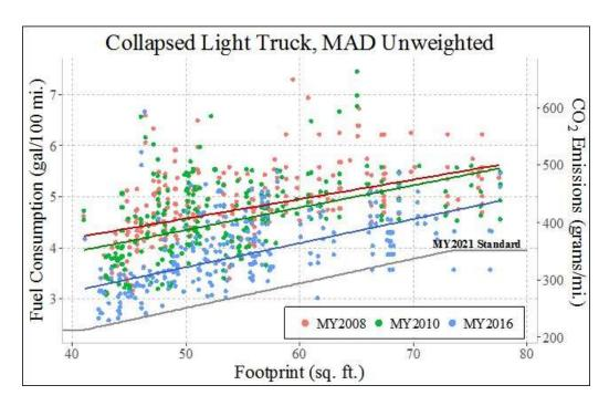
Figure 4-8 - Light Truck Curves Fit with an Unweighted MAD Regression from the Collapsed Dataset
