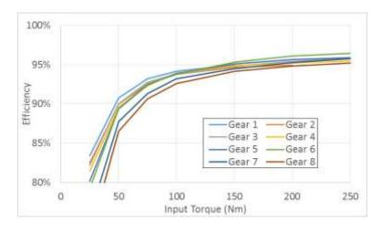
Figure 6-122 - And Efficiency (Right) in Each Gear for an Eight-Speed 845RE
