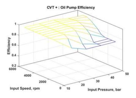
Figure 6-144 - Oil pump efficiency map of CVT Level 2
