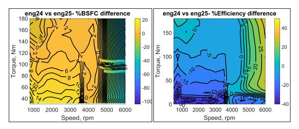
Figure 6-109 - Incremental BSFC and Thermal Efficiency between ENG24 and ENG25
