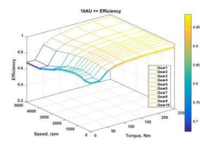
Figure 6-136 - Efficiency map for the 10-speed automatic Level 2
