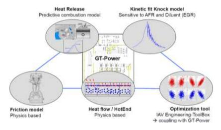
Figure 6-44 - Overview of the engine model development
