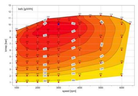
Figure 6-66 - Engine efficiency map for eng01
