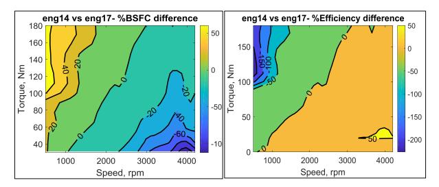
Figure 6-97 - Incremental BSFC and thermal efficiency difference between eng14 versus eng17  $\,$
