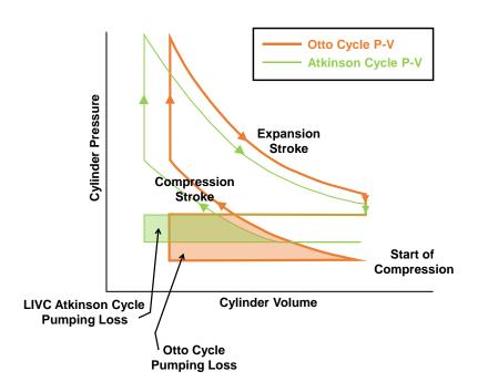
Figure 6-40 - Diagrams of Cylinder Pressure Vs. Cylinder Volume for A Conventional Otto-Cycle SI Engine (orange line) Compared to A LIVC Implementation of Atkinson Cycle (green line) Highlighting the Reduction in Pumping Losses.
