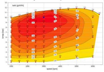
Figure 6-71 - Engine Efficiency Map for Eng04
