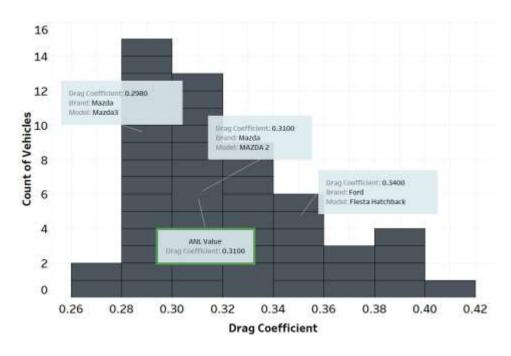
Figure 6-28 - Example of drag Coefficients for Compact Base Vehicle
