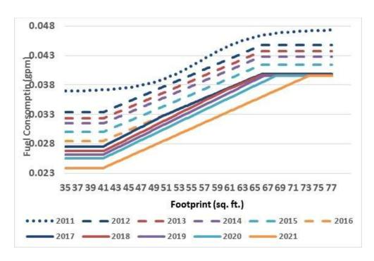
Figure 4-3 - Final Light Truck GPM Target Curves for MYs 2011-2021
