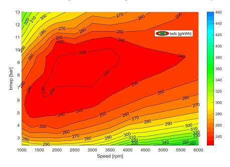
Figure 6-106 - Engine Efficiency map for eng24
