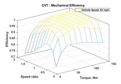
Figure 6-142 - Mechanical Efficiency map of CVT Level 1 at 62 mph
