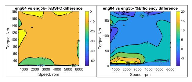
Figure 6-74- incremental BSFC and thermal efficiency difference between eng04 versus eng05b
