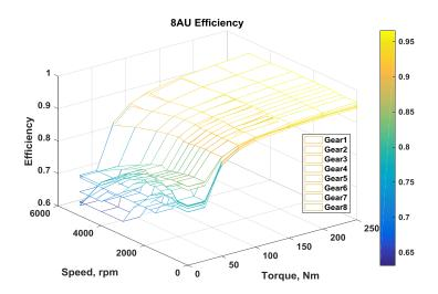
Figure 6-131 - Efficiency map - 8-speed automatic Level 1
