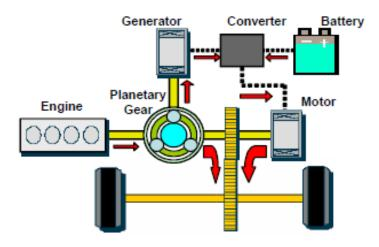
Figure 6-20 - Power Split Hybrid Electric Vehicle
