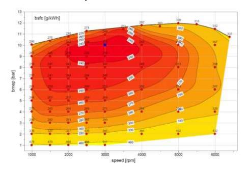
Figure 6-77 - Engine efficiency map for eng7a
