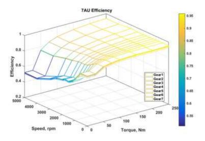
Figure 6-130 - Efficiency map - 7-speed automatic
