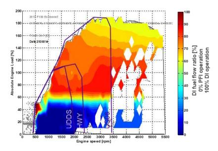
Figure 6-38 - DI and PFI usage map as function of engine speed and load for a 2017 Ford F150 3.5L Ecoboost 187
