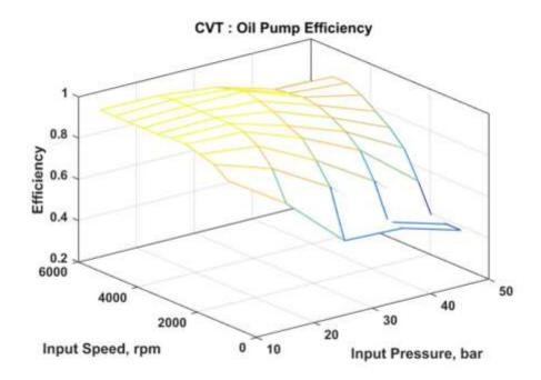
Figure 6-139 - Oil Pump efficiency map of CVT Level 1
