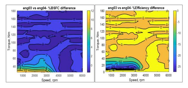
Figure 6-72 - incremental BSFC and Thermal Efficiency difference between eng03 versus eng04
