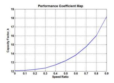
Figure 6-138 - Performance Vehicle Torque Converter Lock up map
