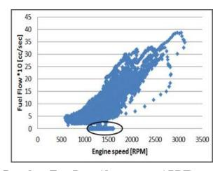
Figure 6-19 - Engine Fuel Cut-off Analysis Based on Test Data (data source APRF)
