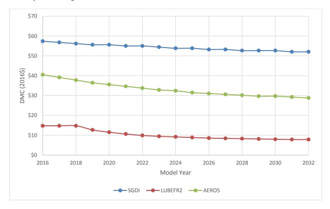
Figure 9-9 - Examples of Learning Curves for Selected CAFE Technologies (Progress Ratio = 0.89)
