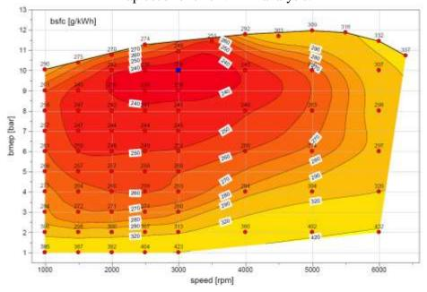
Figure 6-79 - Engine efficiency map for eng8a
