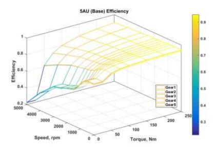
Figure 6-125 - Efficiency map of 5-speed automatic - non-performance classes
