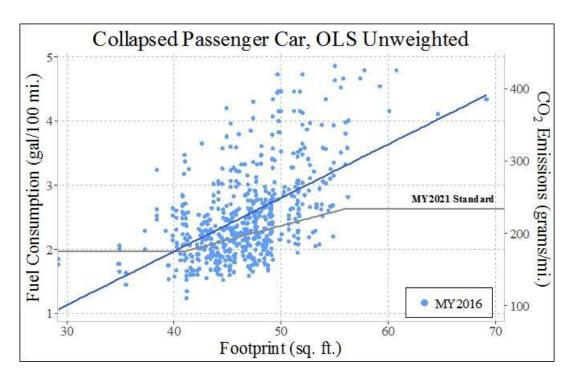
Figure 4-19 - Passenger Car Curves Fit with an Unweighted OLS Regression from the Collapsed Dataset
