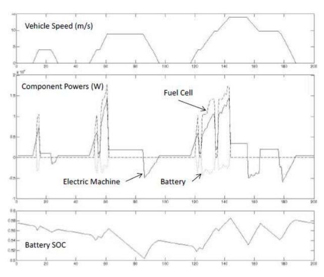
Figure 6-27 - Component Operating Conditions of a FCV on the Urban EDC using Dynamic Programming
