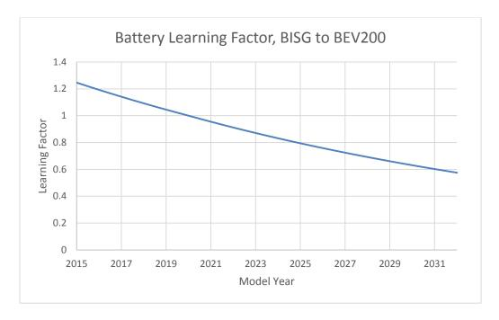
Figure 6-154 - Battery learning factor used for all electrification technologies, BISG to  $$\operatorname{BEV}200$$
