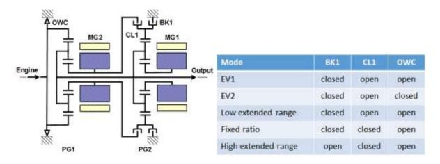
Figure 6-25 - Configuration of the Chevrolet Volt 2016 Powertrain System
