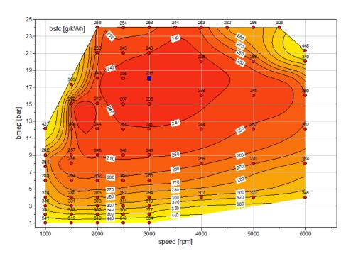
Figure 6-86 - Engine efficiency map for eng13
