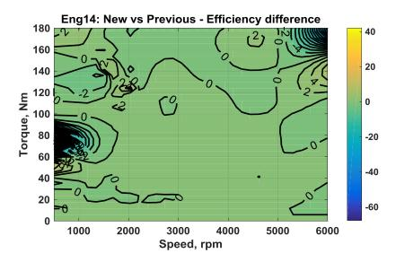
Figure 6-95 - Engine efficiency difference in percent for 93 vs. 87 octane fuel for engine 14 6.3.2.2.20.12 Engine 17 – Diesel 2.2L
