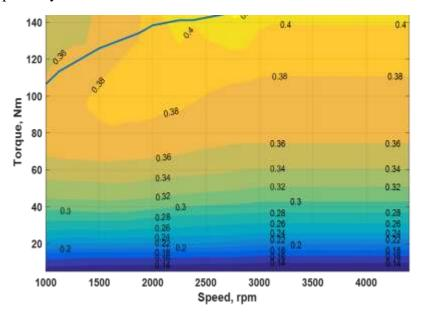
Figure 6-110 - Engine Efficiency Map for eng26
