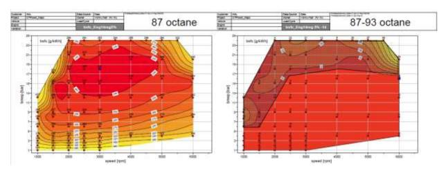
Figure 6-94 - Delta BSFC of 93 (right) versus 87 (left) octane fuel for eng14
