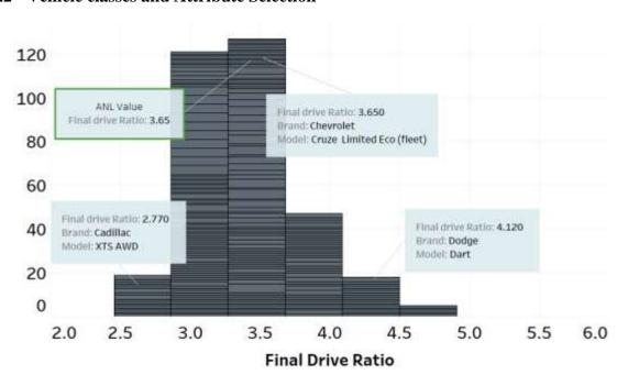
Figure 6-30 - Example of vehicle attribute analysis for final drive ratio of 6AU transmission
