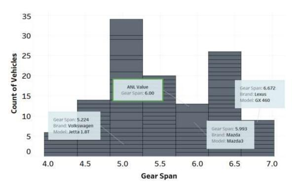
Figure 6-31 - Example of vehicle attribute analysis for gear span of 6AU transmission
