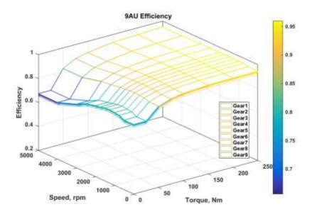
Figure 6-134 - Efficiency map for the 9-speed automatic
