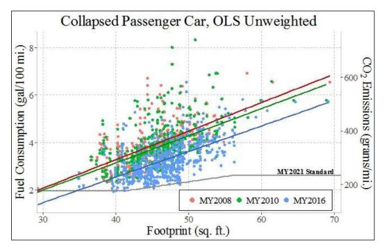
Figure 4-11 - Passenger Car Curves Fit with an Unweighted OLS Regression from the Collapsed Dataset
