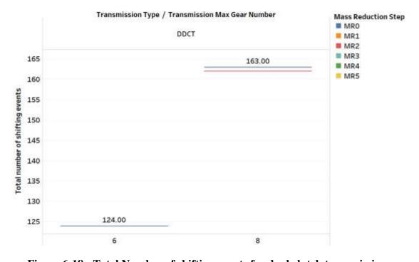
Figure 6-18 - Total Number of shifting events for dual clutch transmissions
