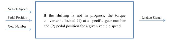
Figure 6-11 - Torque Converter Lockup Control Algorithm
