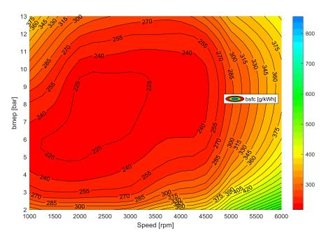
Figure 6-108 - Engine Efficiency Map for eng25
