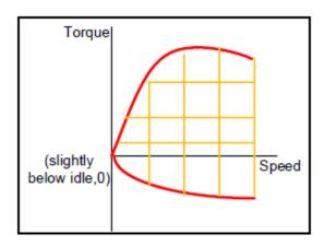
Figure 6-2 - Engine Operating Region for Un-throttled Engines
