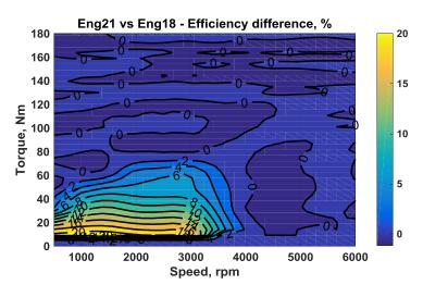
Figure 6-105 - Engine efficiency difference between engine 21 and engine 18
