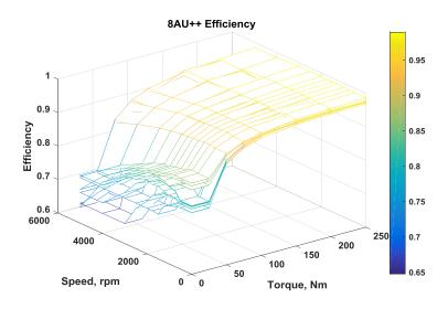
Figure 6-133 - Efficiency map - 8-speed automatic Level 3
