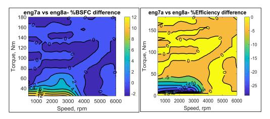
Figure 6-80 - incremental BSFC and thermal efficiency difference between eng7a versus eng8a
