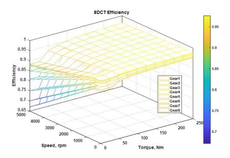
Figure 6-150 - Efficiency map for the 8-speed Dual Clutch Transmission
