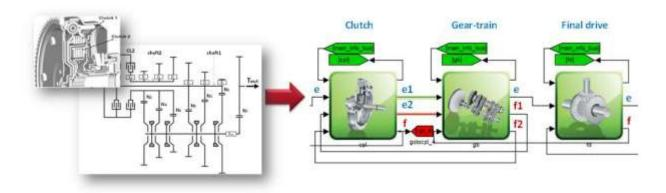
Figure 6-7 - Dual Clutch Gearbox Model Input/Output
