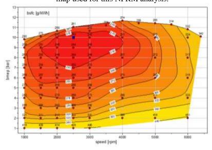
Figure 6-102 - Engine Efficiency Map for eng20
