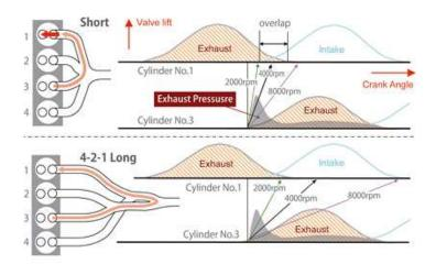
Figure 6-43 - Mazda SkyActiv 4-2-1 exhaust system to mitigate knocking by reducing residual gas.<sup>201</sup>
