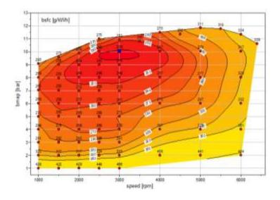
Figure 6-104 - Engine Efficiency for eng21
