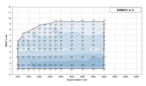
Figure 6-60 - IAV engine 25a incremental difference between 4-cylinder mode versus 3-cylinder mode
