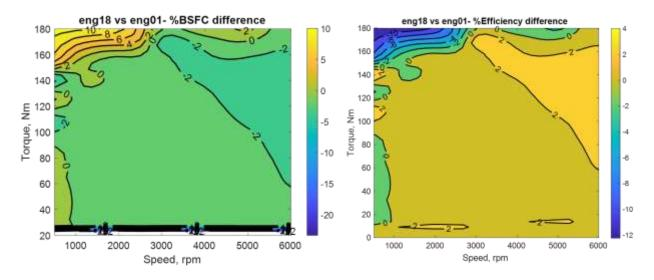
Figure 6-99 - Incremental BSFC and thermal efficiency between IAV eng18 versus eng01
