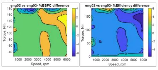
Figure 6-70 incremental BSFC and thermal efficiency difference between eng02 versus eng03
