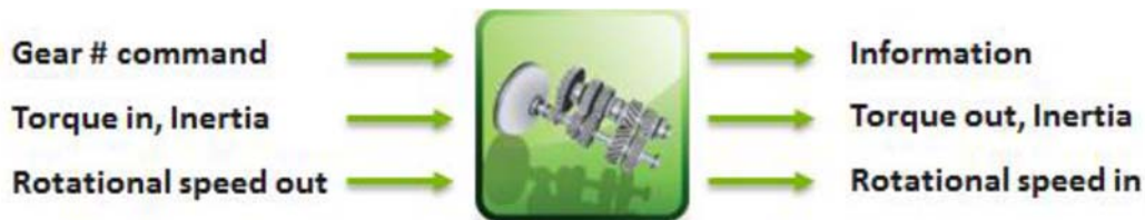
Figure 6-6 - Automatic Gearbox Model Input/Output
