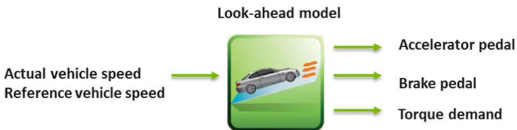
Figure 6-15 - Autonomie Driver Model
