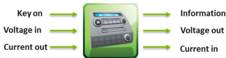
Figure 6-14 - Autonomie Electrical Accessories Model
