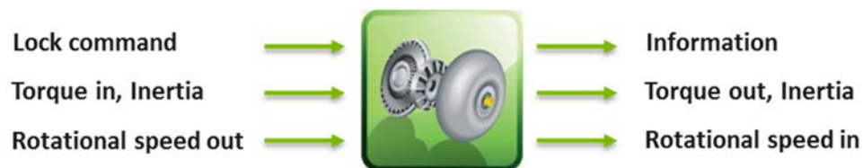
Figure 6-9 - Autonomie Torque Converter Model Input/Output
