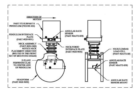
Figure W4. Neck lateral flexion test set-up specifications.
