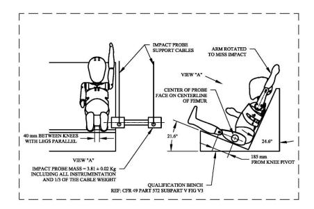
Figure W11. Pelvis lateral impact test set-up specifications.
