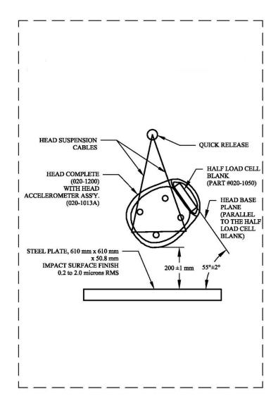
Figure W2. Lateral head drop test set-up specifications.
