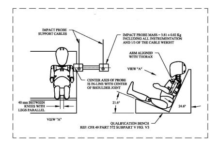
Figure W6. Lateral shoulder impact test set-up specifications.
