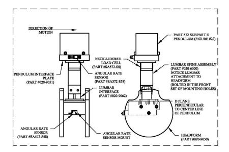
Figure W10. Lumbar lateral flexion test set-up specifications.
