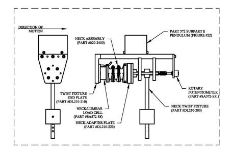
Figure W5. Neck torsion test set-up specifications.
