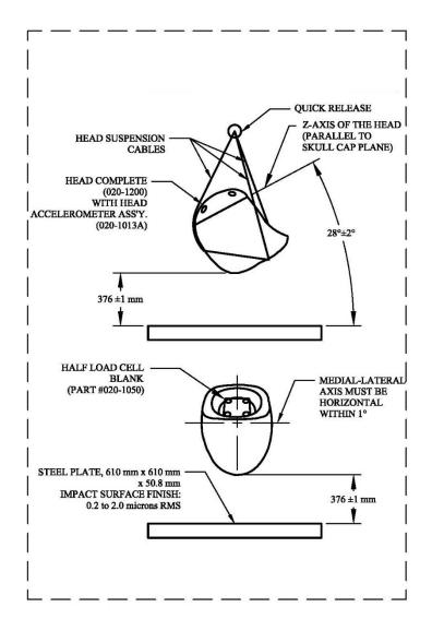
Figure W1. Frontal head drop test set-up specifications.
