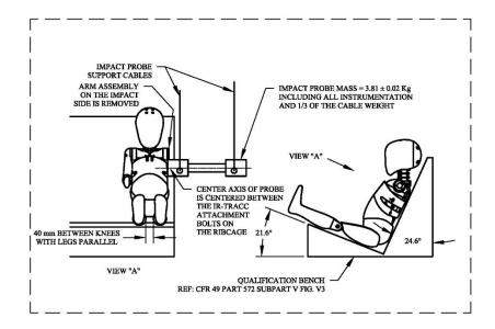
Figure W8. Lateral thorax without arm impact test set-up specifications.
