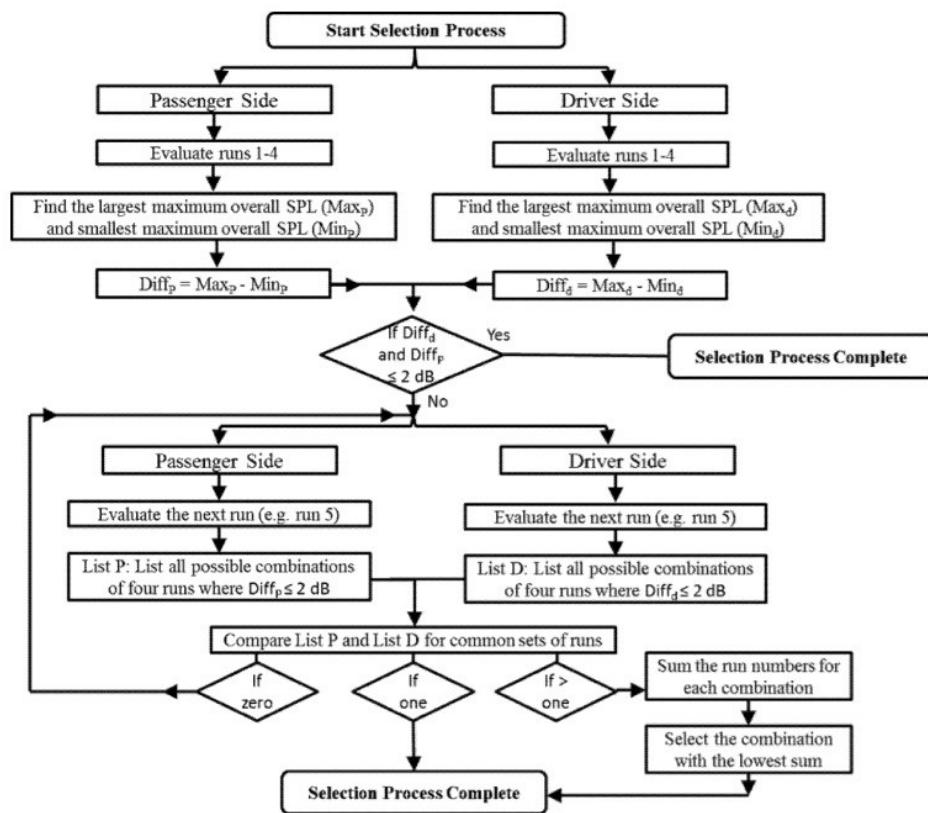
*Figure 2: Selection process to determine “first four valid test runs within 2.0 dBA”*
