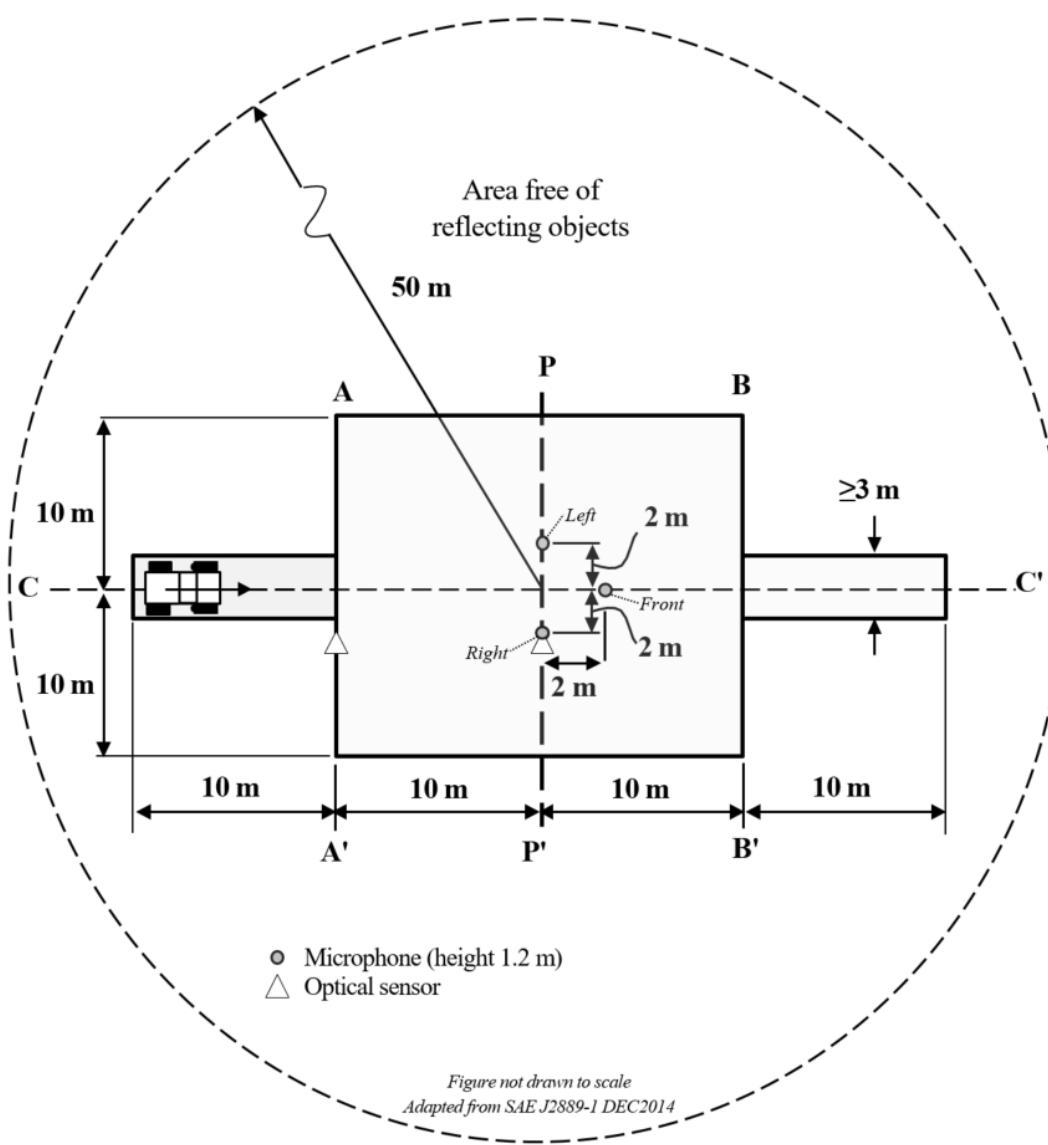
**Figure 1: Test site dimensions. Adapted from SAE J2889-1. Modifications include addition of a front microphone used only during stationary/directivity measures and optical sensors to record trigger signals for pass-by tests.**
