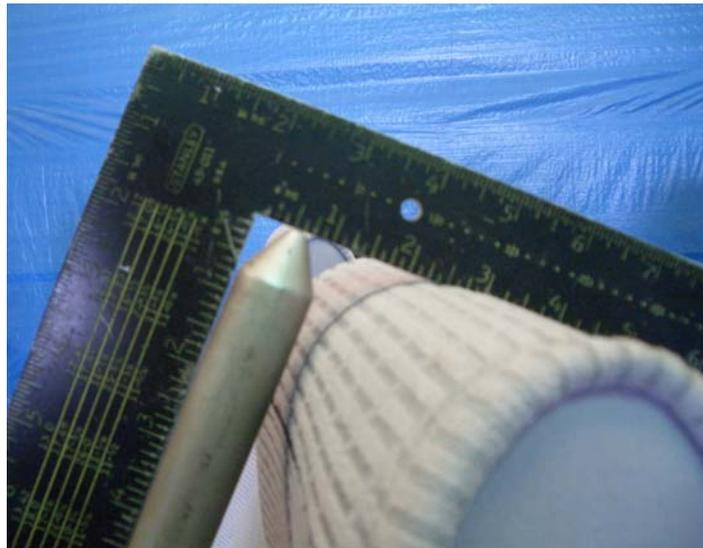
Measure the distance, H, between the H-point and top of probe. Without moving the carpenter's square, mark a point on the head restraint, 65 mm from the top of the extension, draw a line through the point along the width of the head restraint to each end. On each the side of the head restraint, draw a line parallel to the perpendicular edge of the carpenter's square.
