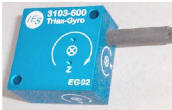
Figure 4 – Denton ATD Rate Gyro, Model IES 3103
