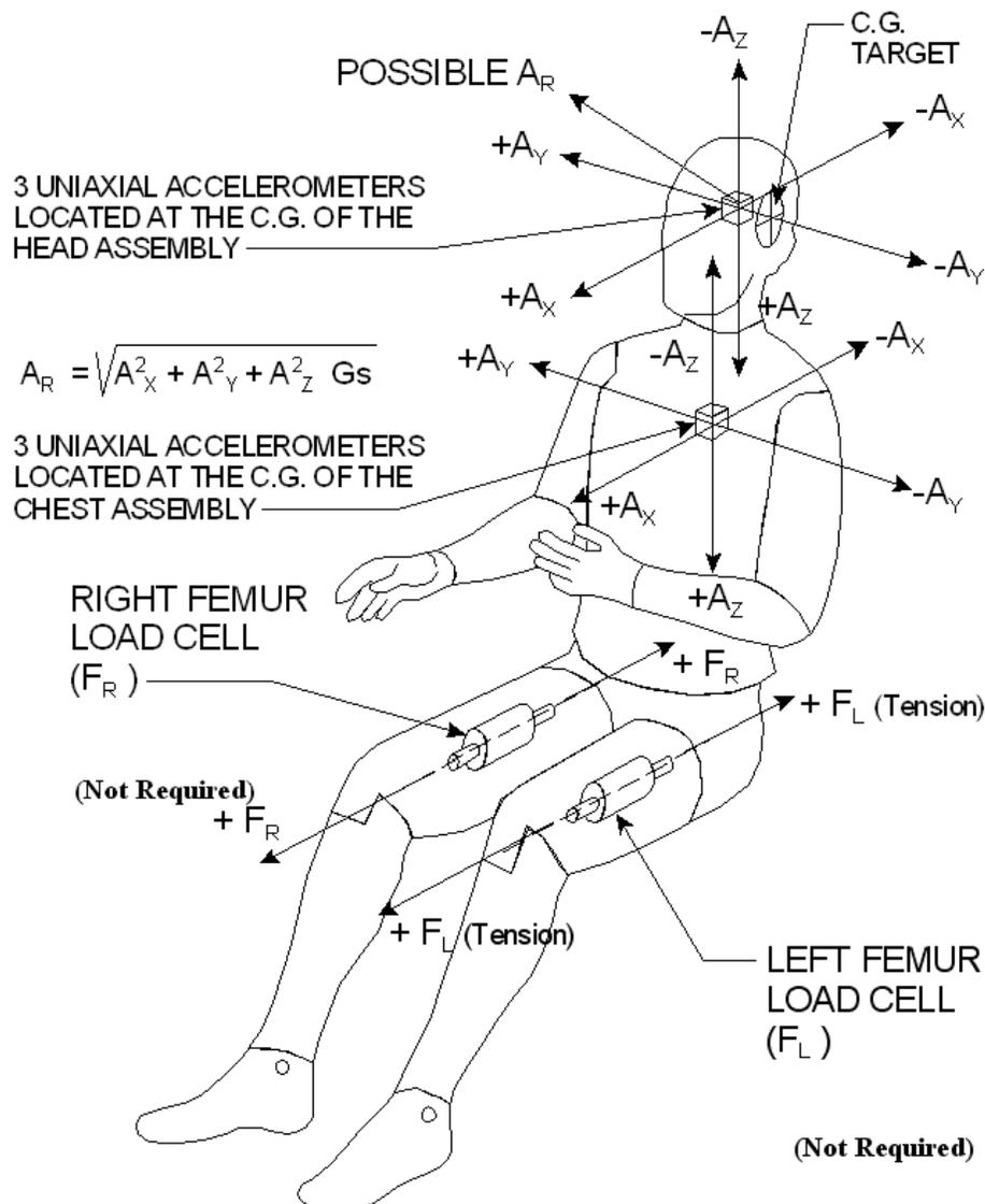
Figure 6 – Sign conventions for dummies. Part 572 Subpart E Test Dummies
