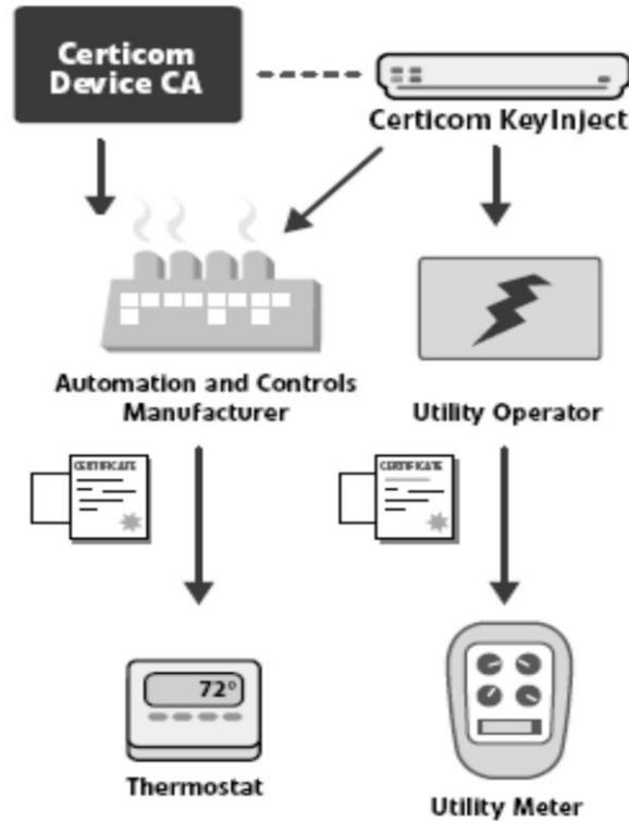
**Figure V-2 ZigBee Smart Energy Certificate System**
