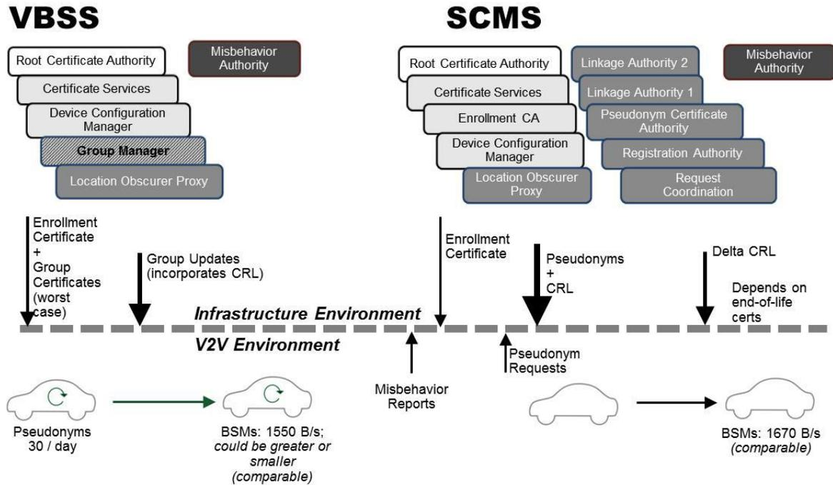
**Figure V-7 VBSS versus SCMS High Level Architecture**
