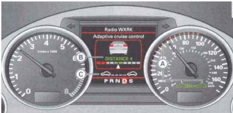
Figure A-1: Audi A8 Adaptive Cruise Control interface elements
