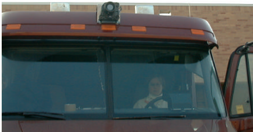
Figure 8. Camera Installed on Truck Airfoil
