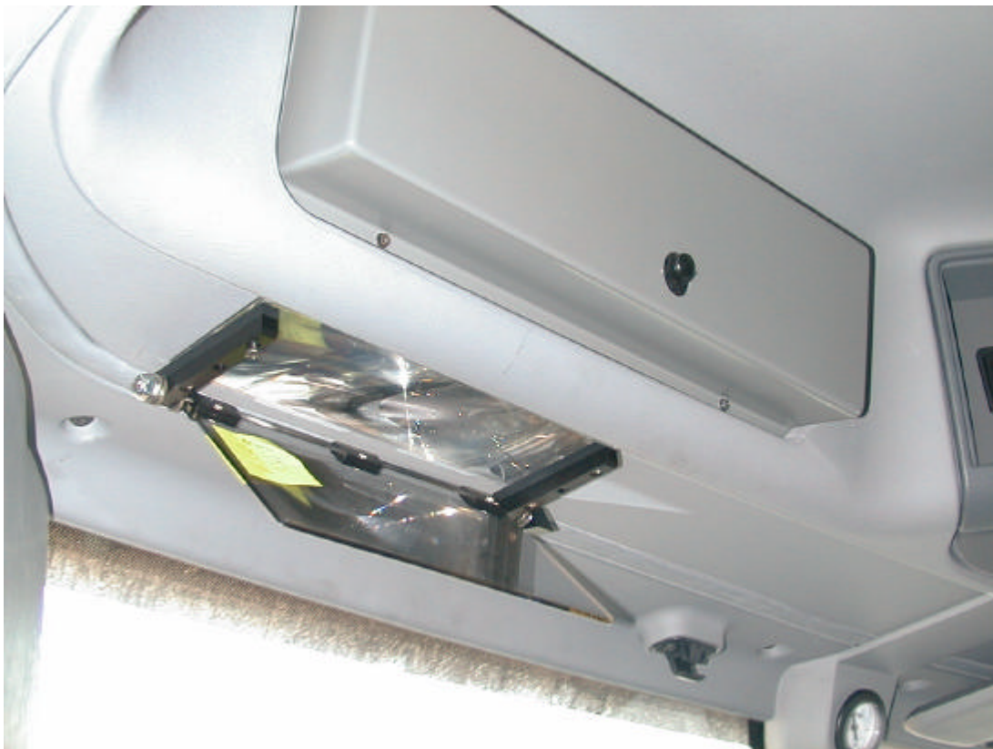
Figure 6. Truck HUD Mounted in Overhead Compartment
