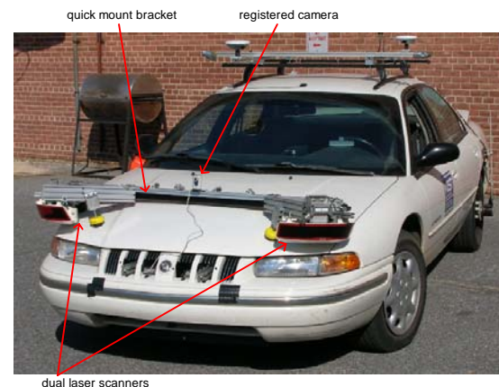
Figure 23. Test-bed Vehicle with Dual-head Laser-range Scanner
