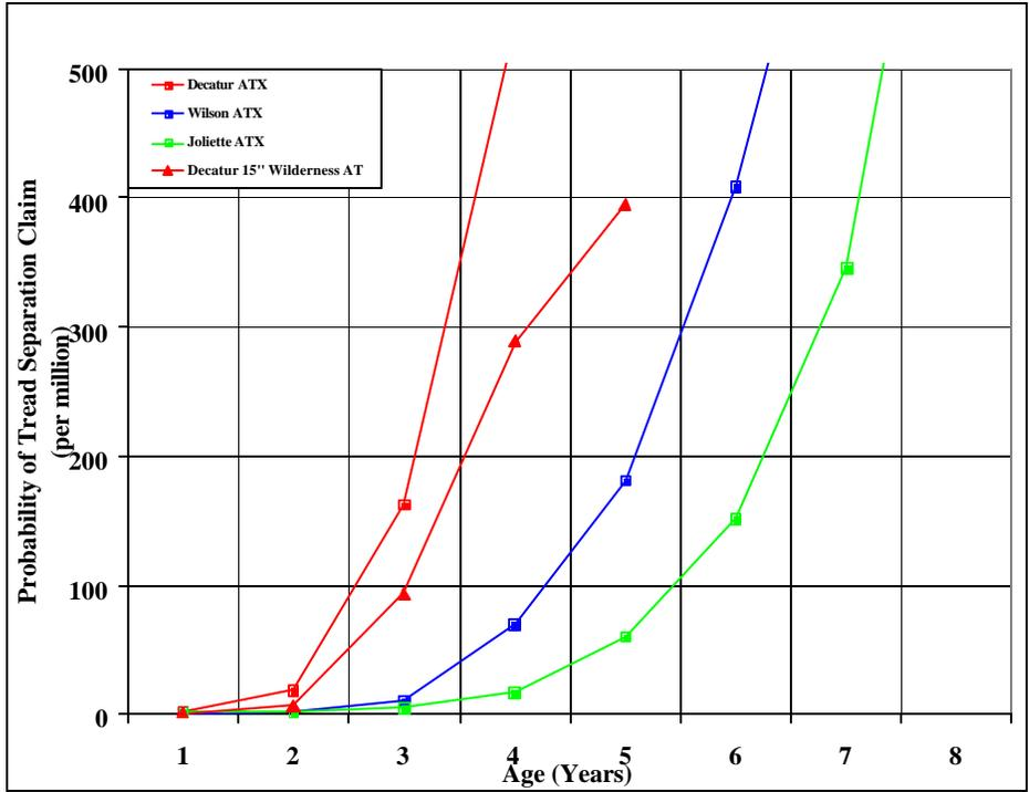
**Figure 18 – Cumulative hazard function, recalled tires, by model and plant.**
