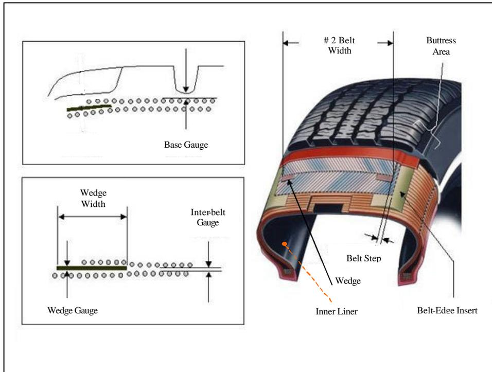
**Figure 7 – Radial tire construction.**
