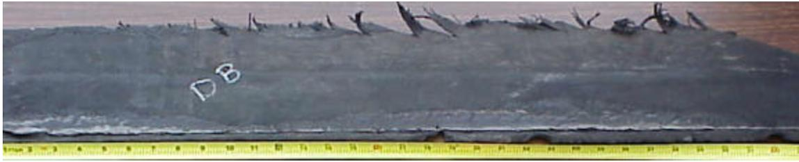
**Figure 37 – Separation patterns on failed Wilderness AT tread
