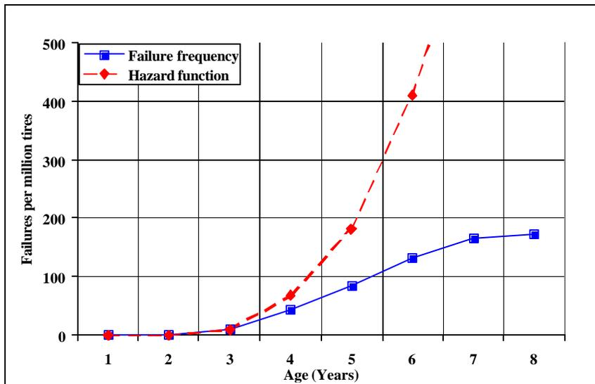
**Figure 17 – Comparison of cumulative hazard function vs. cumulative failure frequency, Wilson ATX P235/75R15 tires.**
