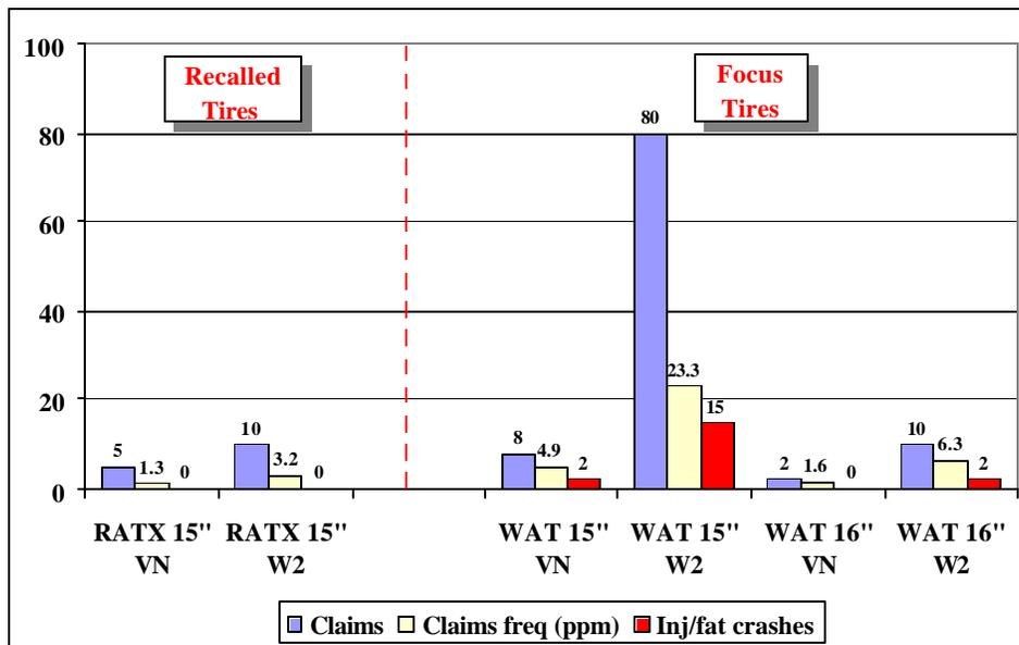
**Figure 15 – ATX vs. Wilderness AT, failure experience comparison, by plant;
