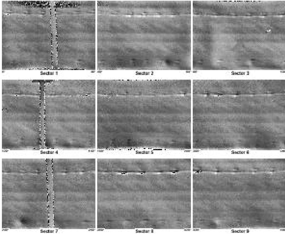
**Figure 30 – Shearography showing localized incipient separations, Wilson P235/75R15 Wilderness AT tire, manufactured in Oct 97(W2 427).**
