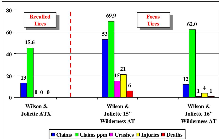
**Figure 42 – Failure experience of ATX and Wilderness AT tires Produced in 1996 at the Wilson and Joliette plants.**
