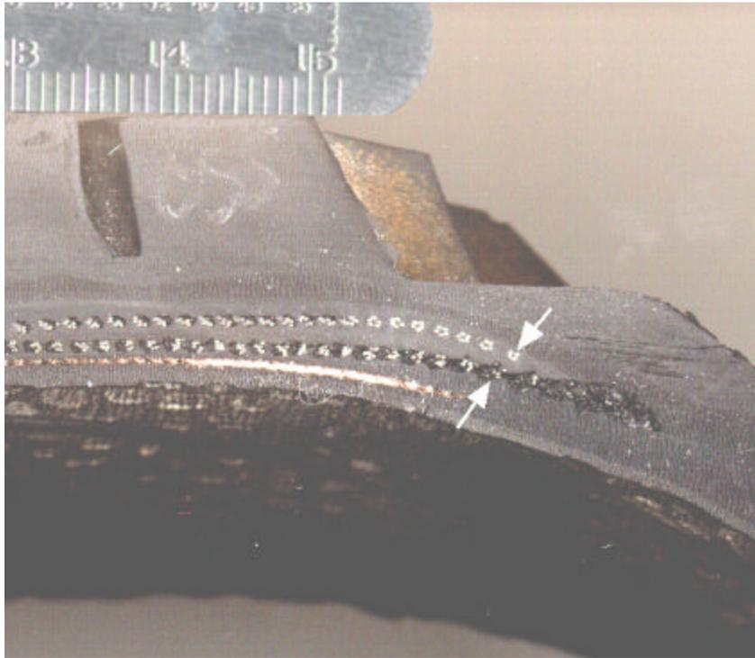
**Figure 34 – Wedge “pinching” under shoulder pocket,
