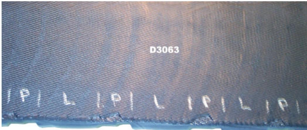
**Figure 31 – Localized separation pattern on tread pull of the same tire; “P” = pocket area, “L” = lug area.**
