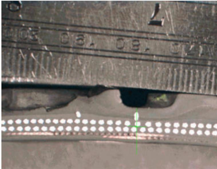
**Figure 28 – Pinched inter-belt gauge under tread groove, Wilson P235/75R15 Wilderness AT tire, manufactured in Nov 97 (W2 467).**
