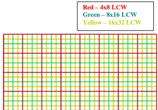
**Figure 5. Load Cell Wall with Increasing Resolution.**
