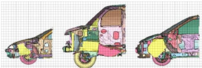
**Figure 3. Vehicle Side Section Cuts: Metro, Econoline, Caravan.**
