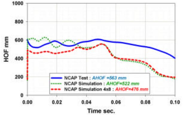
Figure 8. Econoline HOF : Test and Simulation.
