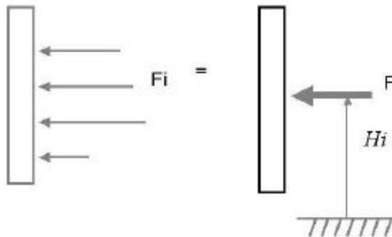
**Figure 1. Average Height of Force Diagram.**
