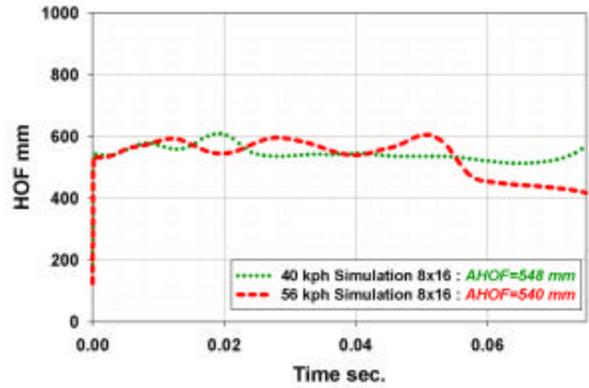
Figure 22. Econoline HOF by Vehicle Speed for 8x16 LCW.
