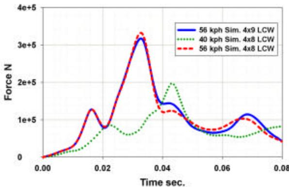
Figure 17. Metro Load Cell Wall Total Force.
