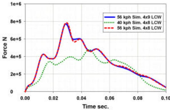
Figure 16. Caravan Load Cell Wall Total Force.
