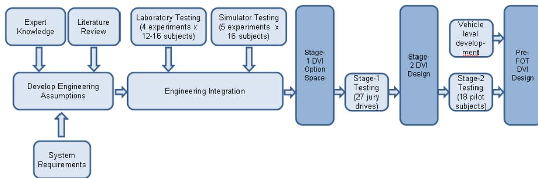
**Figure 1 IVBSS Light Vehicle DVI Design Process**
