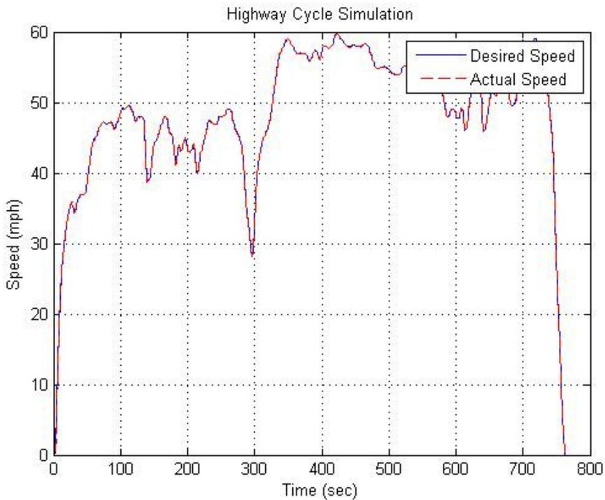
Figure 5-14 Vehicle Speed Trace during Highway Cycle
