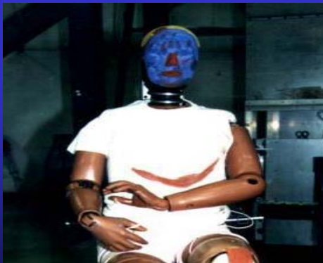
Test 3805 50th Male driver occupant showing transfer paint witness marks indicating steering wheel-to-occupant contact.
