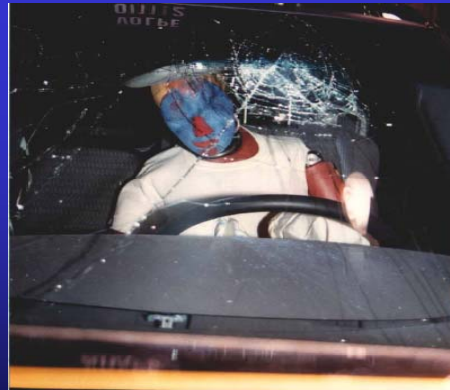
Test 3902 50 th Male driver occupant showing windshield glass-to-head contact.
